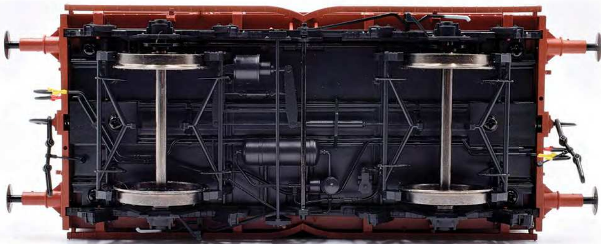
Left: The underframes are equally well-appointed. This is the exquisitely detailed air-braked example.
