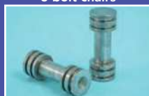
Roller gauges check rail clearance for RTR
