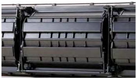
Hopper bay doors are moulded into the underframe and have separately fitted parts for the mechanism.
