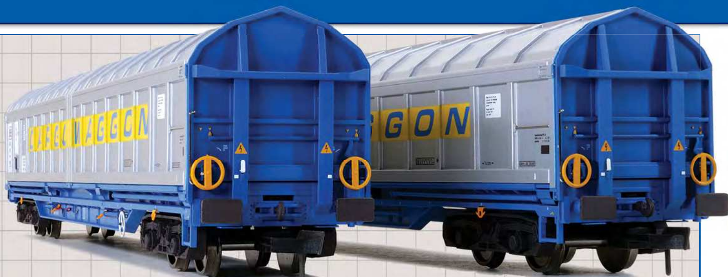
Above: The van ends feature the distinctive handwheels which operate the doors on these vans as well as the rectangular buffer heads.
