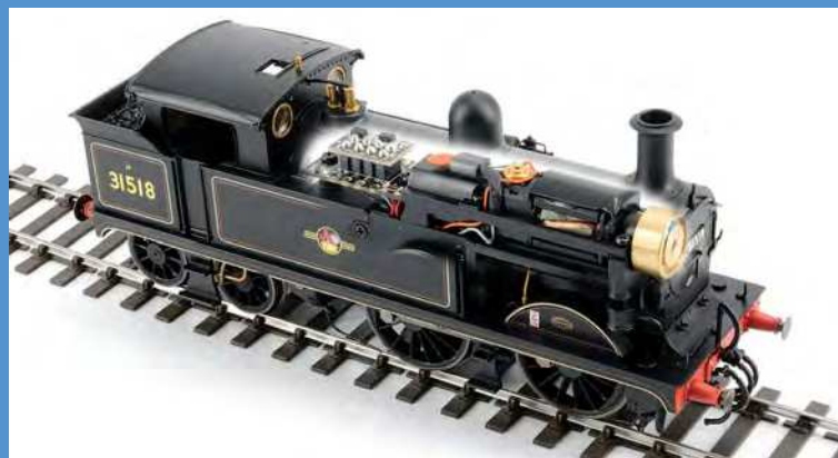
Modern locomotives have decoder sockets inside which allow DCC chips to be added. This Hornby 'H' 0-4-4T has an 8-pin type socket inside.
