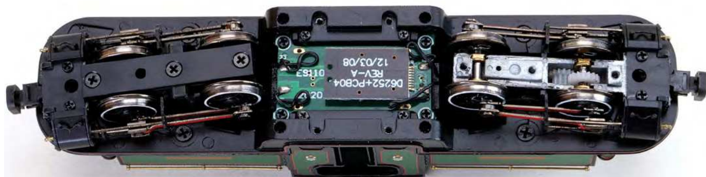
The chassis provides drive to the outer axle of each bogie with a centrally mounted coreless motor. A Next18 decoder socket is positioned beneath a removable panel in the chassis base.
