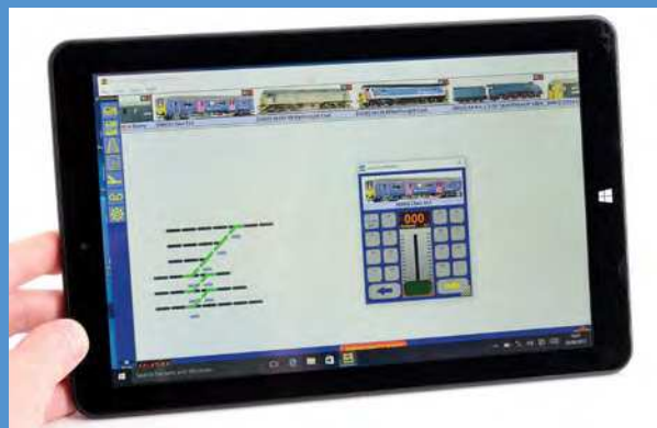
In digital control there is the option for computer control through Bachmann's Railcontroller and Hornby's RailMaster software which allows driving of trains as well as control of points and signals.
