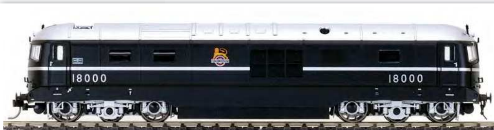
In profile the different wheel sizes of the A1A-A1A bogies are clear. A Kadee coupling is fitted here for testing purposes – tension locks are supplied with the model.
