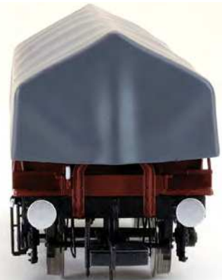
Sprung buffers are mounted at all four corners while optional vacuum brake pipes are included in the accessory pack.
