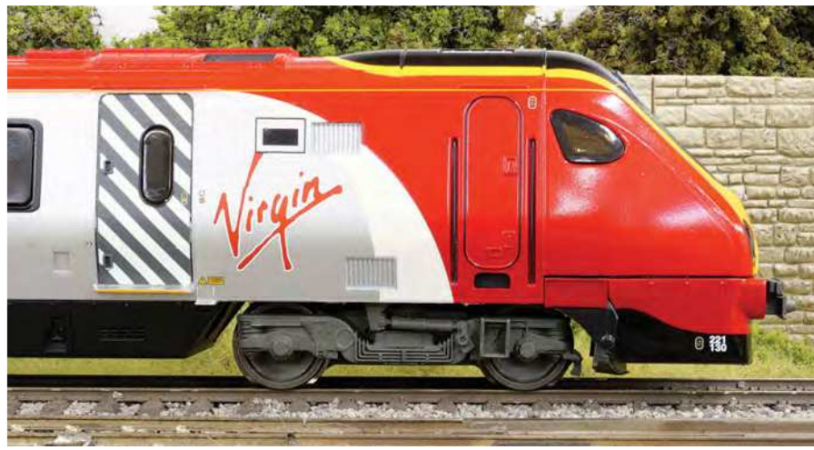
The Class 221 Super Voyagers were distinct from the standard Class 220 Voyager for their outside frame bogies, five-car formation and tilting ability.
