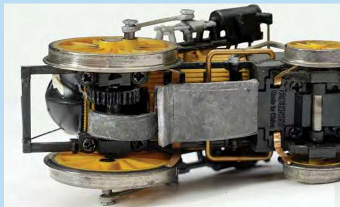
The underside of Rocket showing the unpainted layers of lead added to give the required adhesion.
