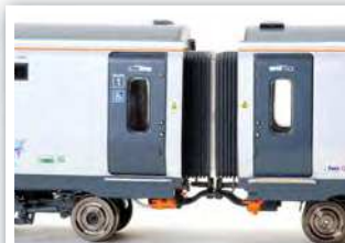
Accurascale has developed new magnetic inter-vehicle couplings for the Mk 5a carriages.
