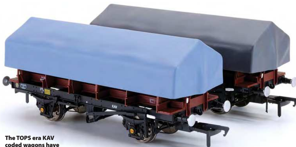
Sprung buffers are mounted at all four corners while optional vacuum brake pipes are included in the accessory pack.
