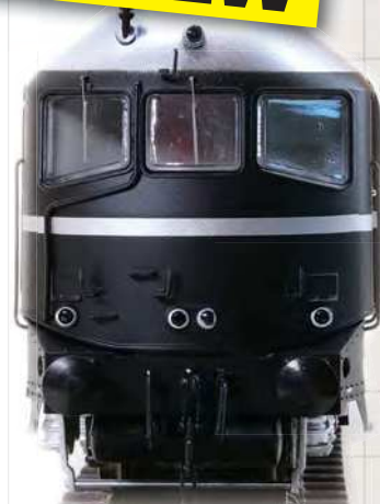
The cab front features all the important details including lamp irons, fine windscreen wipers, steps and more.
