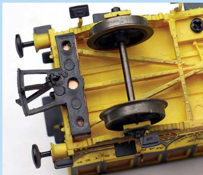
The underside of one of the coaches showing the replacement tension lock couplings fitted (Bachmann 36-025). These have been glued in this position for close coupling.
