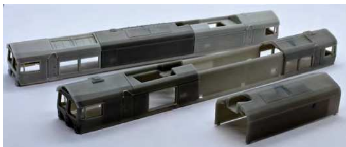
First shots of Revolution Trains' all-new Class 59 diesel with removable centre covers, providing ease of access for installing a DCC decoder.
