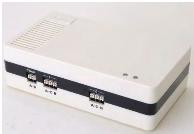
The HM6010 accessory control unit can power point motors, signals and lighting through its four outputs. A 15v DC or DCC track feed are required to power it.
