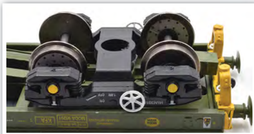
Left: Bogies are injection moulded while brake discs are modelled on opposing wheels in each bogie.
