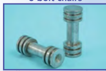
Roller gauges check rail clearance for RTR
