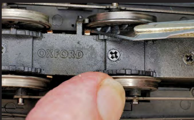
Occasionally you will find that locomotive pick-ups lose contact with the rear of the wheels leading to a model stalling. This can be reshaped carefully to ensure contact.
