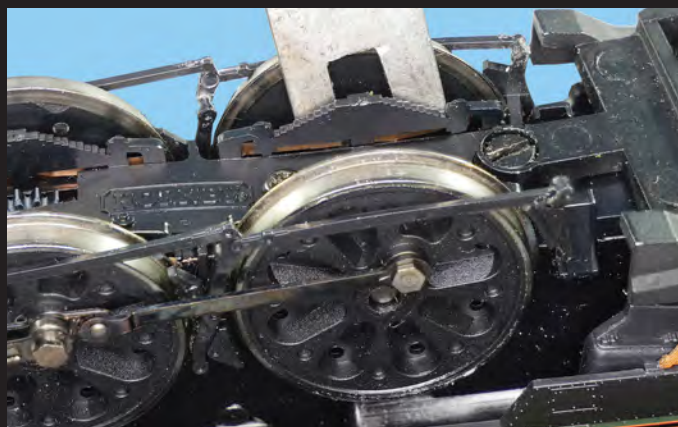
Adjusting wheel spacing calls for careful work. On this Bulleid 'West Country', the rear driving wheel spacing is being adjusted with a specially modified craft knife blade which slots around the axle.
