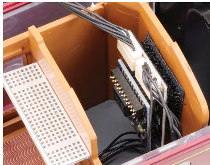
A 21-pin decoder socket is mounted in the toilet compartment to allow for control of interior lighting on DCC. Analogue users can use switches in the chassis.
