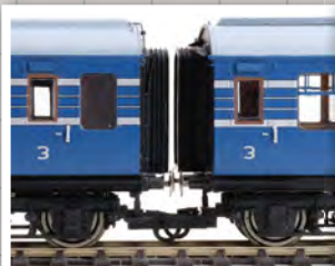
Alternative close couplings and extended gangway connections are optional parts from the accessory bag.
