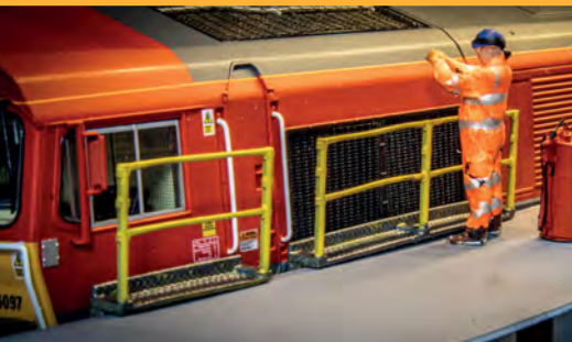
Depot Walkway Safety Barriers
