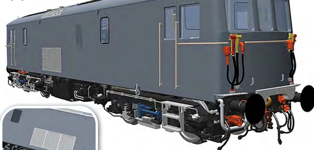
Underframe detail for Heljan's 'O' gauge Class 73.
