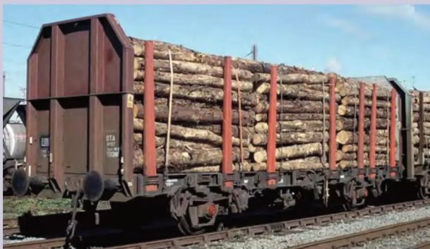
One of the OTAs converted by EWS from an OBA, 110381 is seen at Warrington in September 2001. The stanchion design of these was distinctive with their tapering shape, although only seven of the nine positions were in use on this occasion. David Ratcliffe
