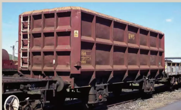
Following re-bodying at RFS Doncaster some five years earlier, SSA 470151 was stabled in Tees Yard during May 2002. While retaining the previous general look, the ends and ribs were of a more substantial construction.
