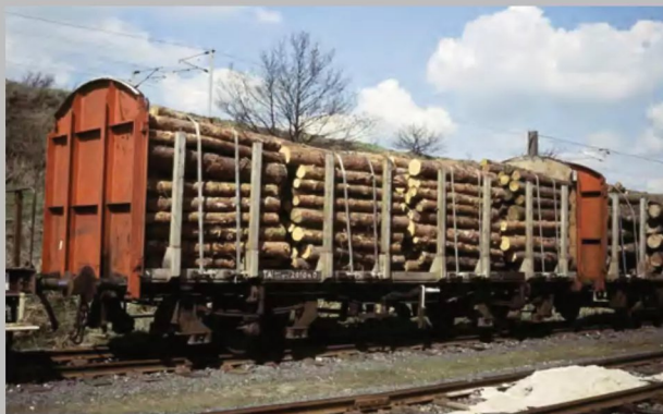
In its original Railfreight colours, OTA 201040 stands at Warrington in April 1989. Converted from a VDA van, this is from the batch fitted with the unusual and somewhat experimental Taperlite suspension. Eight stanchions are carried.
