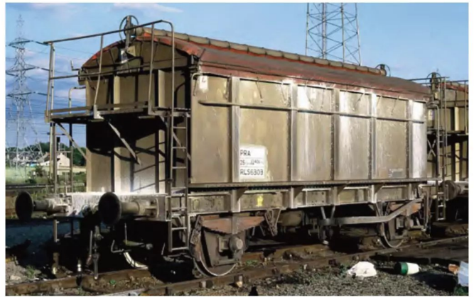
The PRA clay hoods also racked up huge mileage on their trips from Pontois Mill, near St Blazey, to Corpach, a short distance from Fort William, to supply the Wiggins Teape paper mill. With the latter having no hopper discharge facilities, a grab-unloaded box wagon design was necessary. The first of the build, RLS6303, is seen at Mossend during July 1984. Trevor Mann
