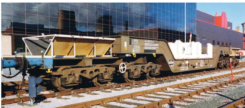
The first of the 1977-built well wagons, BNFL95600 is pictured at Sellafield in August 1993 when fitted with a cradle designed to accommodate two cuboid Magnox flasks. In addition to handling the traffic from Japanese and some of the European pressurised water (PWR) and boiling water (BWR) reactors, all of which arrived in cylindrical flasks, these wagons were also used to carry the flasks that were shipped to Barrow Docks from the Magnox power stations built at Latina in Italy and at Tokai in Japan. David Ratcliffe Collection
