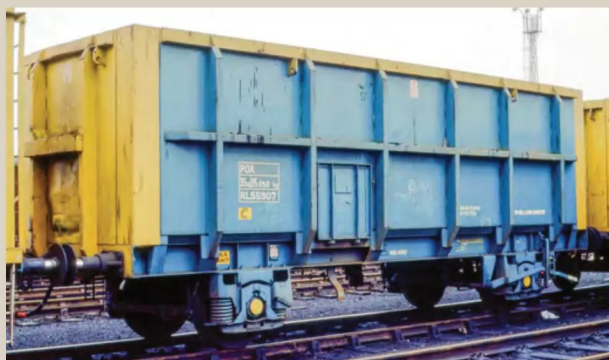
The first production batch of Railease POAs featured an access hatch for internal cleaning and thick corner posts without ribs. After a year in traffic, RLS5907 was still in good shape at Tinsley Yard on November 6, 1983.
