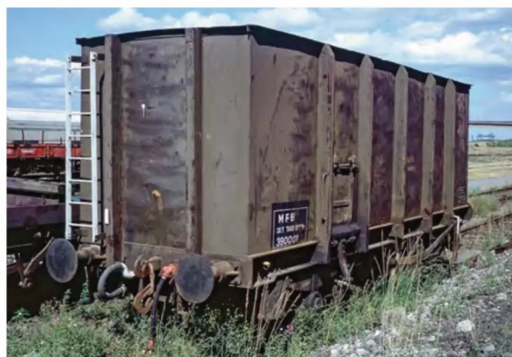
RIGHT: The battered and bent Railease POA prototype RLS5900 stands in the Heywood yard of Standard Wagon awaiting repairs in December 1986. Built eight years earlier, there is not a straight panel to be seen, illustrating the harsh environment that scrap wagons had to endure. By the end of the decade, it would have a much more substantial body in place, this being based on the POA 'blackadder' design and would become SSA 470100 in the 1990s. David Ratcliffe
