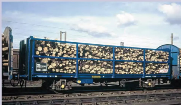
An unsuccessful prototype was PNA CAIB4800, which is seen shortly after delivery at Warrington in May 1990. Featuring mesh sides, the timber was loaded transversely but this limited the length of logs that could be carried. David Ratcliffe
