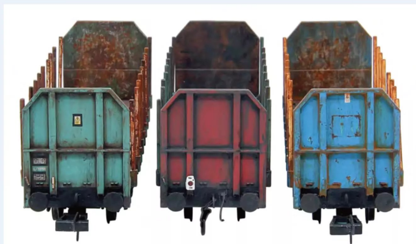
A comparison of different weathering on the outer ends shows how dirt and rust can be added in varying amounts. The Thames Board blue example also illustrates how the outline of the removed logo can be replicated. With the red OTA nominated as the rear vehicle of the set, this has received a tail lamp, screw coupling and brake pipe.
