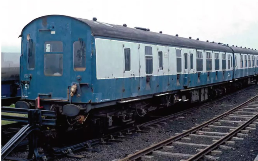
ABOVE: The original MoD escort coaches MODA99150 and, behind, MODA99151 are seen at MoD Bicester in April 1995, from where they would soon be withdrawn. The modifications to the brake end are evident as are the bodyside vent recesses. The generator exhaust is also visible on the roof along with small louvres in the former luggage door. David Ratcliffe
