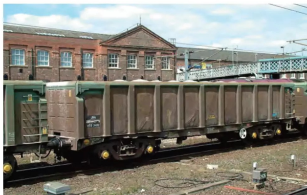
ABOVE: Initially built to serve the virtual quarries set up by Railtrack, the Marcroft-built JNAs have seen considerable use in scrap and other traffic following their replacement. Now owned by VTG, they retain the green livery under the grime. VTG3460 is seen at Doncaster on July 14, 2006, although not in scrap traffic. Martyn Read
