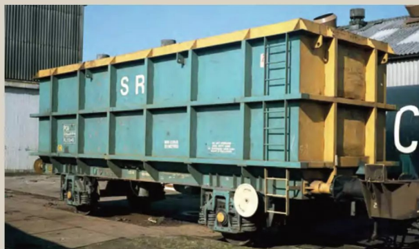
Built on the underframe of a British Steel PGA hopper, RLS5040 consequently inherited its disc handbrake equipment. The wagon is seen at Standard Wagon's Heywood workshops in October 1985 waiting for its rib plates to be fitted. David Ratcliffe
