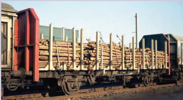
112372 shows the most common variant of ex OCA conversion with the taller angled ends at Warrington Dallam in April 1986. Livery is the original red/grey with 13 pockets provided for 11 stanchions to theoretically cater for different lengths of log. David Ratcliffe
