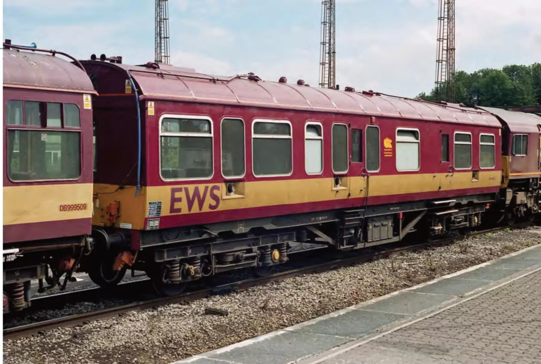
LEFT: On August 15, 2002, DM45020 and DB999509 were both recorded at Bristol Temple Meads while heading for Devonport behind 66115. Built in 1944 by the LMS, the saloon was modernised in the early 1990s with new hopper windows and B4 bogies while one end window was plated up for escort use. Simon Bendall
