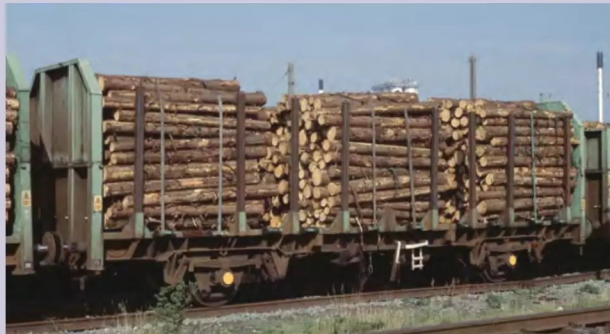
Another OTA in the revised green livery, 112272 is again seen at Warrington in September 1999 and with its original 13 stanchion pockets now reduced to just nine, of which eight were in use. This brought the ex OCAs into line with the former VDAs. David Ratcliffe
