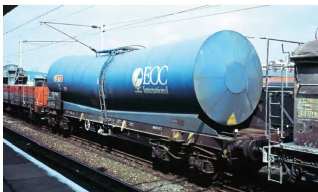
TIA 83 70 7895 201-2 was one of the four 50ft long STS bogie slurry tanks built using underframes from withdrawn LPG tanks. Although ferry fitted, they rarely, if ever went abroad and this tank was returning to Cornwall from Aberdeen when seen at Warrington in May 1989.
