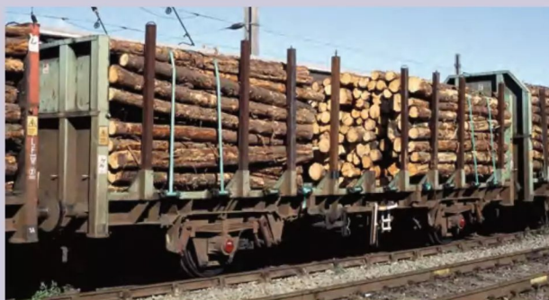
Another of the original OTAs seen on the same day, 112347 displays the pale green livery that appeared in the early 1990s. When converted, this batch had 11 stanchions but both wagons were down to nine positions by this date, losing two outer pairs. David Ratcliffe
