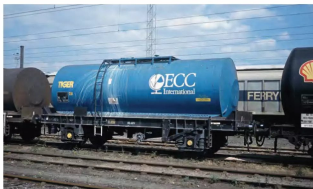
By 1988, Tiger Rail's batch of 51t caustic soda tanks were no longer required by ICI and many of the 28 wagons were reassigned to clay slurry traffic. TUA TRL70705, one of a dozen to be repainted in ECC colours, was spotted at Warrington Arpley yard in July 1990.
