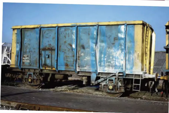
RIGHT: The battered and bent Railease POA prototype RLS5900 stands in the Heywood yard of Standard Wagon awaiting repairs in December 1986. Built eight years earlier, there is not a straight panel to be seen, illustrating the harsh environment that scrap wagons had to endure. By the end of the decade, it would have a much more substantial body in place, this being based on the POA 'blackadder' design and would become SSA 470100 in the 1990s. David Ratcliffe
