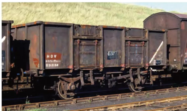
ABOVE: To allow late surviving 21-ton minerals to work amongst air-braked stock, a number were given a through air pipe and recoded MDW. B312194 is seen at Tinsley on July 20, 1986, and they were also found in Scotland and on Teesside. Trevor Mann
