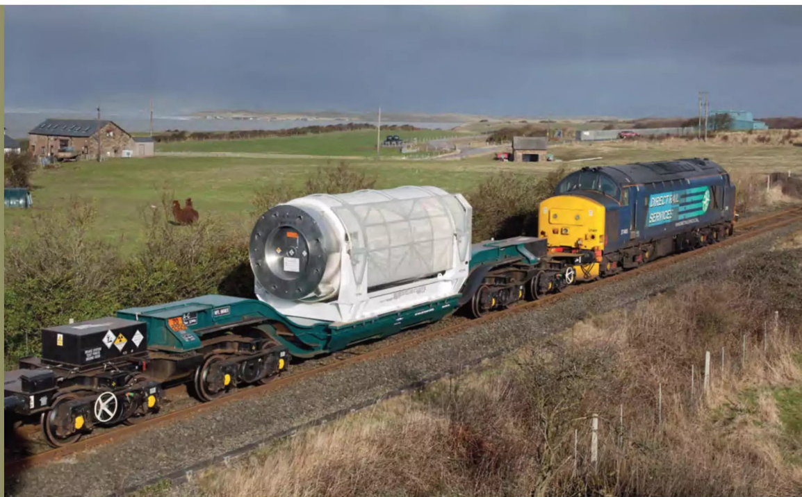
RIGHT: Current day KXA BNFL96905 is seen near Barrow in February 2014 while loaded with a TN28VT flask being returned to Japan, this carrying vitrified waste. Reflecting modern construction methods, these flask wagons are much less bulky than their predecessors but able to carry heavier flasks. Examples have also visited Eastleigh Works in the past for maintenance work, taking them well out of their usual operating area. Dave McAlone
