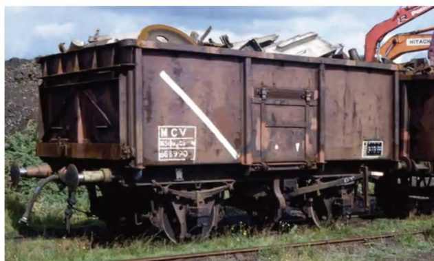
Vacuum-braked and re-bodied 16-ton mineral wagon B68990 (diagram 1/114) is seen at Central Wagon, Wigan Springs Branch, on August 10, 1982. It is carrying the remains of other newly-scraped wagons! Trevor Mann
