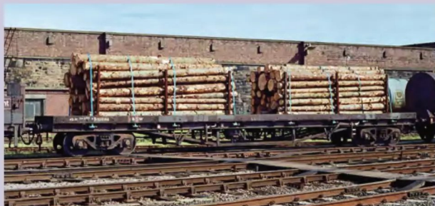
The BSW bogie bolsters were a useful addition to the timber fleet, being vacuum-braked and air-piped. B928188 is seen at Workington in March 1986 carrying two long bundles of logs but three piles could also be accommodated. Dave McAlone
