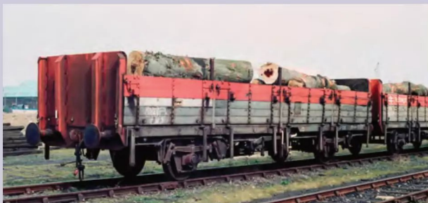
With some of its door pillar stanchions raised, OBA 110691 stands at Middlesbrough Goods Yard on April 9, 1990, loaded with substantial logs. Unlike the OTAs, timber loaded in OBAs was not always strapped in place. Adrian Nicholls
