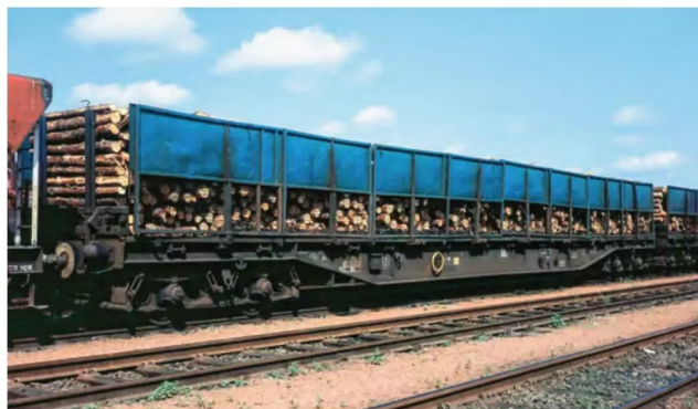
In 1989, to cope with a shortage of wagons suitable for carrying short lengths of round timber, six Cargowaggon flats (five Type 1 and one Type 3) were fitted with side sheets. Leased by BR, they ran from loading points at Huntly, Inverness, Inverurie and Keith to the Caberboard factories at Irvine and Stirling. However, this use proved to be short-lived and all had been returned to their original condition by the end of 1990. IPB 33 80 4742 041-3 is pictured at Mossend in July 1990 while en route from Inverness to Irvine; it would receive the more familiar IGB TOPS classification the following year. David Ratcliffe
