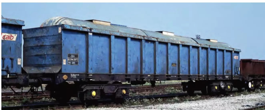
ABOVE: Displaced from Sheerness traffic, 15 of the JXAs received covers made from recycled TEA barrels to carry lightweight scrap from Shotton to Port Talbot, this being conveyed as part of existing services between the two locations. On August 10, 1997, PR3110 displays the unusual looking result while laying-over at Dee Marsh. David Ratcliffe
