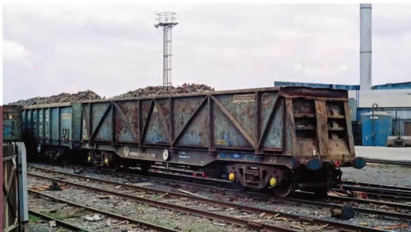
One of the original Sheerness Steel POA (later PXA) scrap wagons is seen at 'home' on March 27, 1988, while it waits to be unloaded. Like its seven sisters, PR3003 was built as a bolster wagon by Procor in 1974/75 before being converted into a scrap carrier during 1981 with new sides added to the original ends. The fragmented scrap load suggests it was either loaded at Ridham Dock or the 600 Ferrous Fragmentisers Ltd plant at Willesden.
