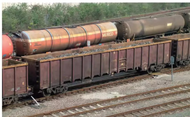
ABOVE: Scrap transport has been one of the primary roles of the MBA 'monster boxes' since they were built for EWS by Thrall Europa at York Works in 1999. Now operated under the DB Cargo banner, 500127 is seen at Washwood Heath, Birmingham, on April 23, 2005, with its maroon paint having seen better days. Martyn Read
