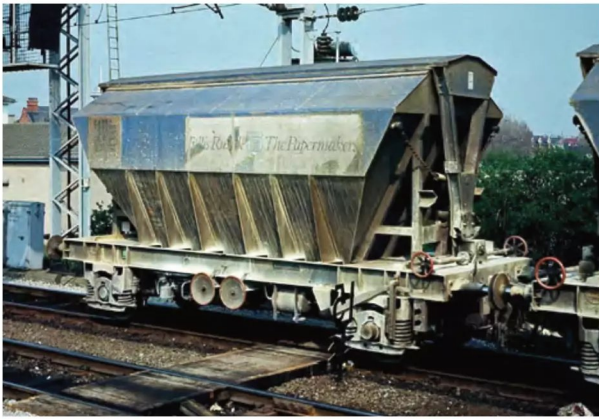
The Tullis Russell PAAs made one of the longest journeys of all the clay wagon types, running from Cornwall to the firm's paper mill at Auchmuty, Fife, via the restricted clearance branch from Markinch. On April 15, 1987, an empty TRL12807 brings up the rear of a Speedlink working at Warrington Bank Quay on the long journey back to the southwest. David Ratcliffe
