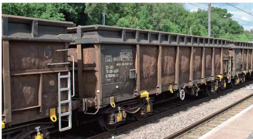
The JRAs were originally built for Tiphook Rail in 1988/89 for aggregates use but have found several roles over the years. One of the more recent was the DC Rail scrap traffic to Cardiff Tidal, for which they received somewhat obvious height extensions during the course of the operation. Now owned by Touax after its acquisition of GE Rail Services, 33 70 6790 040-3 is seen at Kings Norton on June 15, 2015, while returning empty to Stockton. Dan Adkins
