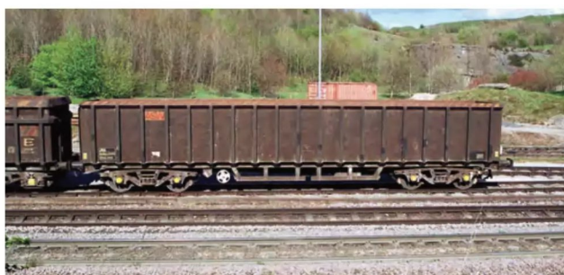
ABOVE: The last of the new box wagons were the WH Davis-built JNAs, these again serving ASW/Celsa when first delivered in 2002. Built using the bogies and running gear from withdrawn TEA tankers, they have subsequently seen use on other traffic as well with GERS4414 pictured at Peak Forest on May 16, 2012. David Ratcliffe
