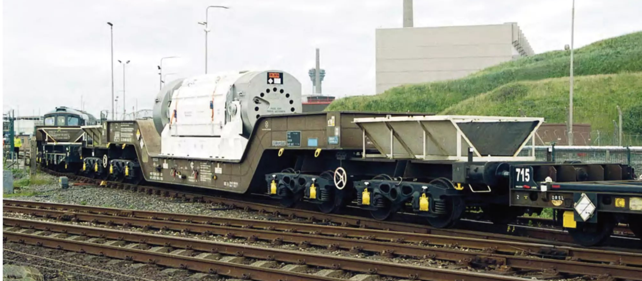
The last of the three 116t BNFL KYAs 33 70 9986 008-8 arrives at Sellafield from Barrow Docks in June 2005 carrying a NTL11 81t flask. This type of flask was used for European shipments, this consignment having originated at Beznau, Switzerland. The silver shock-absorbers would sit in the cradles over the bogies while moving internally around Sellafield. David Ratcliffe
