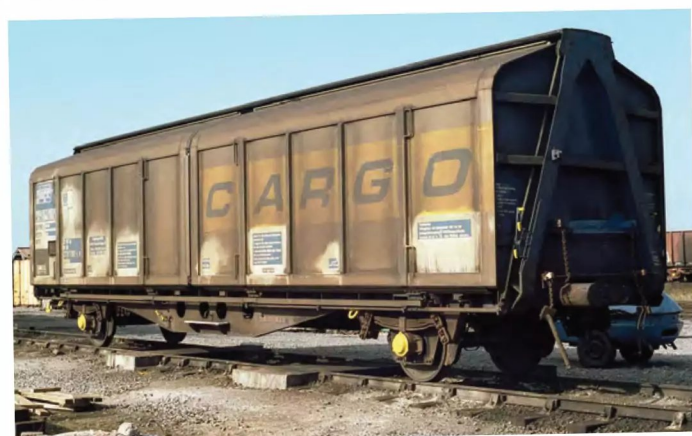
ABOVE: IZA 23 80 2793 192-8 had been split for maintenance when recorded at Immingham Yard on October 9, 1995. These vans lacked conventional buffing gear on the inner end.
