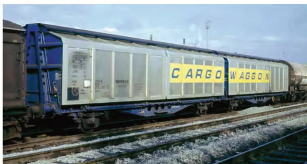
ABOVE: Cargowagon twin-vans were a common sight in Speedlink and later Enterprise wagonload services. From the first batch, IZA 23 80 2794 010-1 was en route from Hereford to Glasgow with a load of cider when recorded at Warrington Walton Old Junction yard in March 1987.
