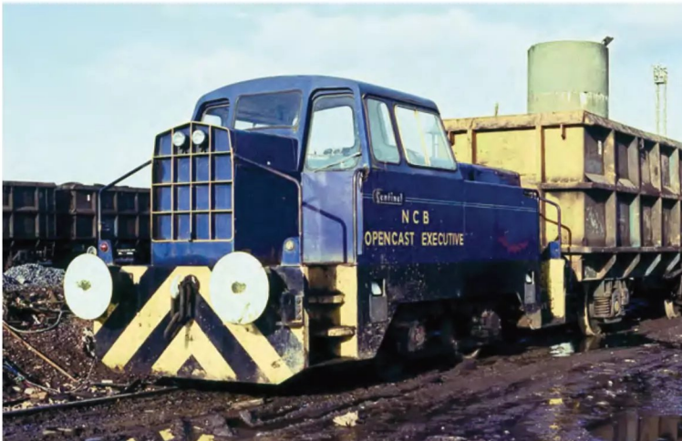
LEFT: Many scrap yards had their own industrial shunter to move wagons around, even if the yards were not overburdened with trackwork. Seen at EMR, Kingsbury, around 1990, this former National Coal Board Sentinel had found a second industrial career and could be easily reproduced in 4mm scale using the Hornby model. Simon Bendall Collection
