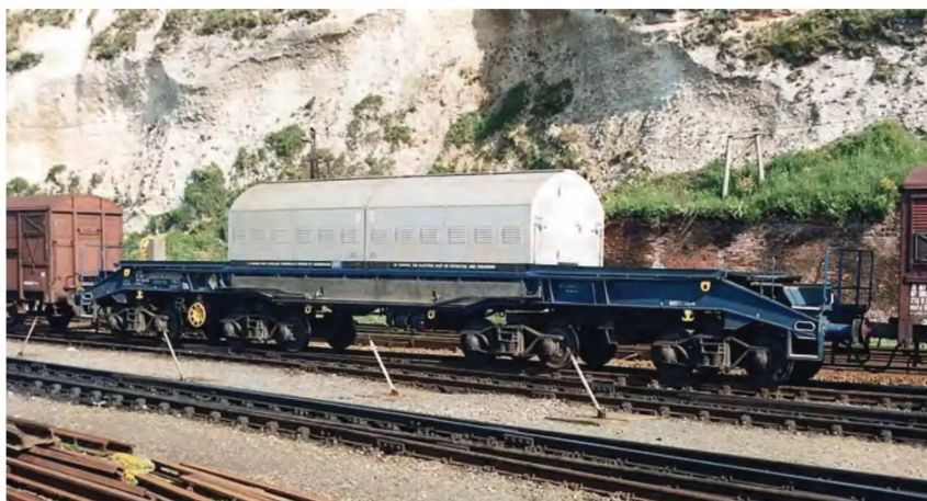
RIGHT: The first of the two German-registered IQAs, 33 80 9987 000-2 is pictured at Sellafield in October 1993 after recently arriving from Gundremmingen. The distinctive angular shape of the cover makes for an interesting comparison with the more rounded style used on the other NTL flasks. David Ratcliffe Collection
