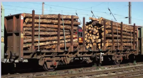
One of the original OTA conversions from 1985 is seen at Warrington in September 1999, ex OCA 112263 retaining the lower flat end. Surprisingly, these wagons were never altered even though it reduced the number of logs that could be carried. David Ratcliffe
