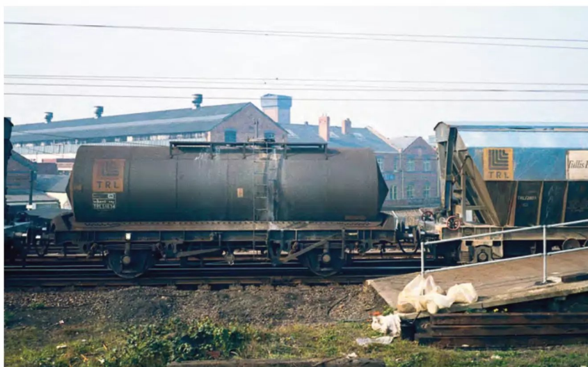
Tiger Rail modified 20 45t caustic soda tanks to carry clay slurry via Speedlink by replacing their leaf springs with parabolic suspension. TTA TRL51634 passes through Warrington Bank Quay in September 1985 while en route from Burngullow to Stirling.
