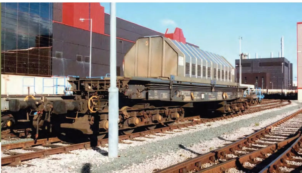
RIGHT: The first of the two German-registered IQAs, 33 80 9987 000-2 is pictured at Sellafield in October 1993 after recently arriving from Gundremmingen. The distinctive angular shape of the cover makes for an interesting comparison with the more rounded style used on the other NTL flasks. David Ratcliffe Collection
