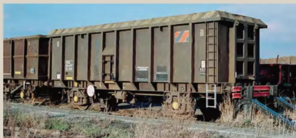
The striking livery on the 'blackadders' was soon lost under the grime but RLS5225 was showing traces of it at Cardiff Tidal on the same day. An example of the Standard Wagon build, it had a 51 tonne GLW and lasted longer. Adrian Nicholls
