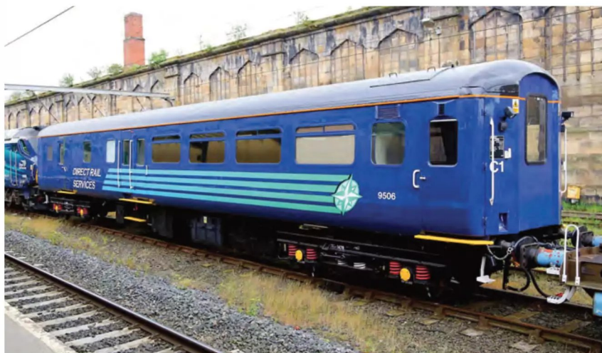
ABOVE: The latest escort coaches to be converted by DRS are a pair of Mk2e BSOs, 9506 being newly completed when recorded at Carlisle on May 22, 2017, behind 68008 Avenger . It was coupled to an empty IKA Megafret intermodal twin with 88001 Revolution on the rear as part of a turning move from Kingmoor TMD. The modified saloon windows with their hopper ventilators are a notable addition while the generator grille is at the far end of the vehicle. Nathan Williamson
