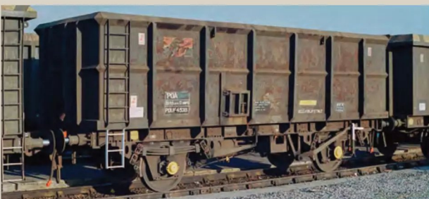
Representing the Powell Duffryn POAs, PDU4538 was residing in the yard at Cardiff Tidal on October 20, 1993. Built on a Shell TTA underframe, this example was rated to carry 33 tonnes with a GLW of 46 tonnes.
