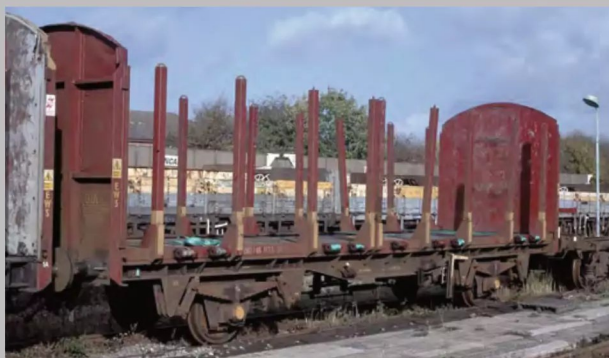
Some of the ex VDA OTAs were modified with a ninth stanchion, this being located in the centre of the wagon, curiously directly adjacent to another. Repainted in EWS colours, 200746 is seen at Crewe Gresty Lane on October 31, 1999.
