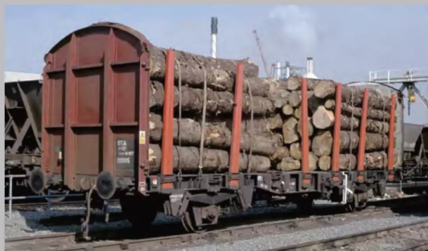
An example of a VDA converted in the late 1990s by EWS, 210185 was at Warrington on April 16, 2000. Just six stanchions are fitted while the placement of the data panel on the ends was commonplace on the EWS livery. All: David Ratcliffe
