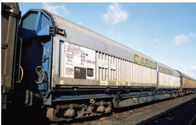
ABOVE: The prototype 'hold-all' van 83 80 4741 000-0 is seen at Cardiff Tidal on September 27, 1991. It had a series of narrower ribs along the sides than the production batch and had arrived empty in South Wales to be loaded with rod coil for export.
