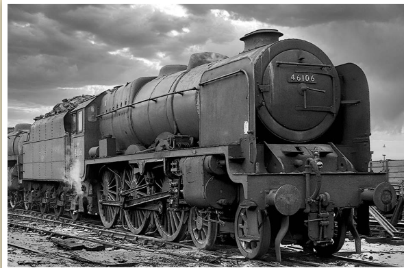
Above: 46106 Gordon Highlander with its unique BR standard class smoke deflector. Irwell Press.
