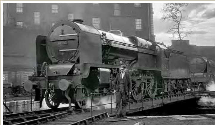
46137 The Prince of Wales' Volunteers showing the smaller deflector with the curved top. Irwell Press.
