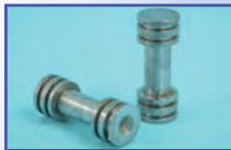
Roller gauges check rail clearance for RTR
