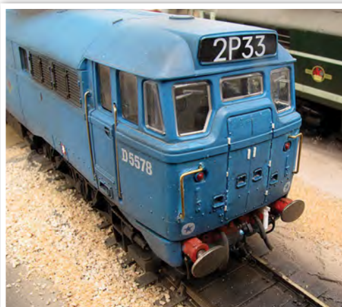
In June 1961 Brush Type 2 No D5578 was released into traffic in the same 'Electric Blue' carried by the first batch of LMR 25kV electrics. It later received yellow warning panels but was repainted standard green in 1964. This is a Lima body on a sawn-up Hornby chassis.
