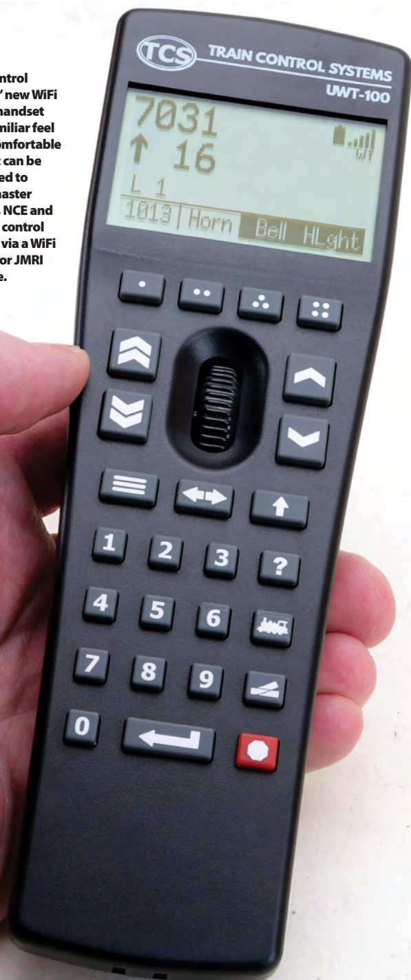
The memory stores previously used locomotives in the handset for future use. Recall is accessed as the first step in the main menu.
