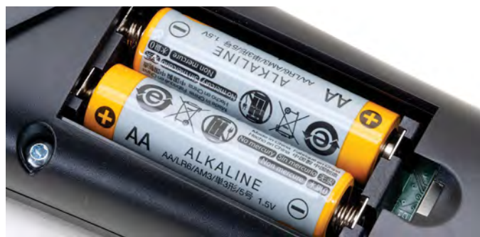
A pair of AA batteries are all that power the UWT-100 handset. TCS expects up to 20 hours of operation from a single set and both re-chargeable and non-rechargeable types can be used.
