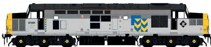
37051 Railfreight Metals (intermediate single rivetted roof)
