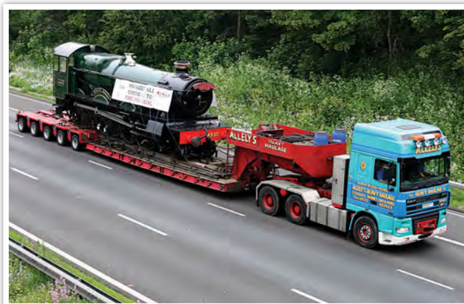
On June 7 2007, 4930 Hagley Hall makes good time along the M5. Shot from a convenient overbridge, this view gives a good idea of the way the locomotive is standing on rails anchored to the trailer as well as the specialised equipment carried on board. Jamie Woodland, Allelys Heavy Haulage Ltd.
