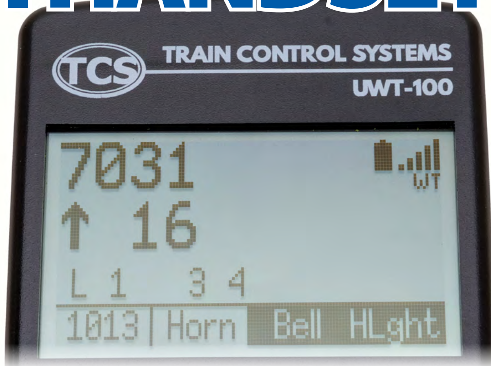
Locomotive control is quick to understand and simple to use. Navigating the menus is made easy by the comprehensive LCD display.
