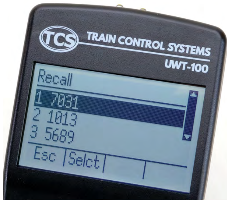
The memory stores previously used locomotives in the handset for future use. Recall is accessed as the first step in the main menu.
