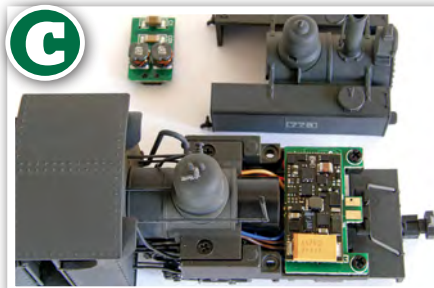
C A push fit of the specially produced Zimo MX659N18 sound decoder is all the installation required. At this point the model can be reassembled and put into service using the factory fitted speaker. The following steps show how to fit an optional larger speaker.
