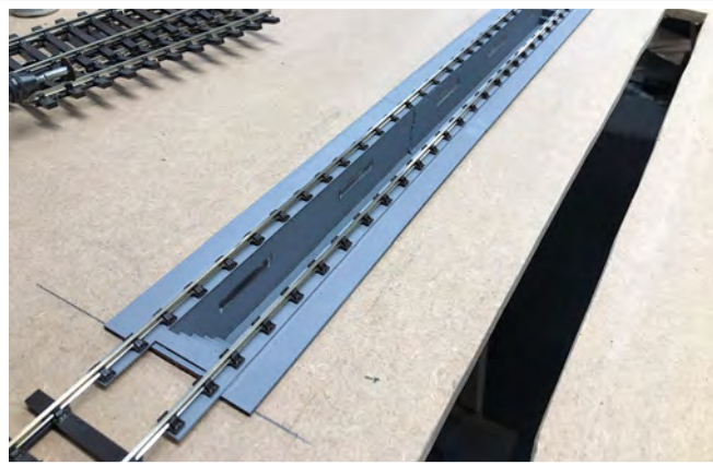
KS Laser Designs laser cut inspection pits were built, cut to length and then set into the baseboard. The openings were marked by drawing around the pit base and cutting out the redundant material with a jigsaw.
