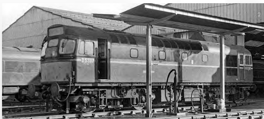
A standard design of fuelling point was created for diesel facilities with an inclined roof to keep rain off crews operating the equipment. BRCW Class 27 D5397 stands at Cricklewood fuel point in April 1969. Railphotoprints.uk .
