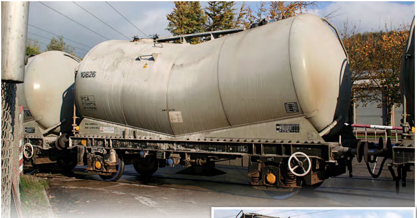
Above: Vee tanks have been a familiar sight on cement traffic since 1973, many of them built by BR at Ashford and Shildon. This example, seen at Hope on October 27 2005, is from a batch built in 1979 for Associated Portland Cement Manufacturers Ltd (APCM), better known by its Blue Circle branding. Since 2001 the organisation has been owned by the French company Lafarge SA. Mick Bonwick.
