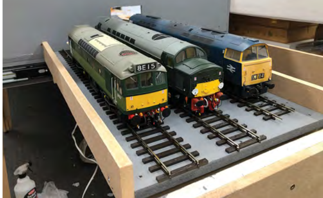
The three-road traverser can hold three large 'O' gauge diesels. All three tracks are live at all times through the DCC power supply.
