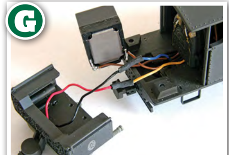
G I soldered the speaker wires (brown) to the new larger speaker and joined the wires for the rear headlamp (red and black), insulating them with shrink wrap tubing. The speaker was insulated at the rear with Kapton tape. The bunker was refitted to the footplate with the speaker part way into the space created with a portion onto the centre of the footplate.
