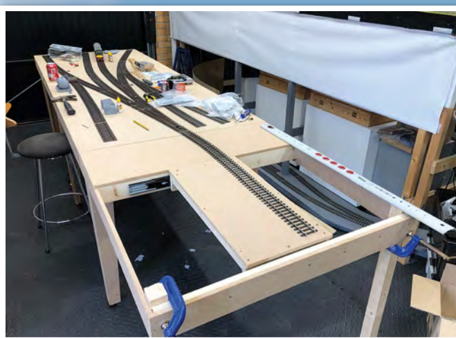
A third baseboard was built from 12mm MDF to create space for a road bridge as a scenic break and a three track traverser storage yard.
