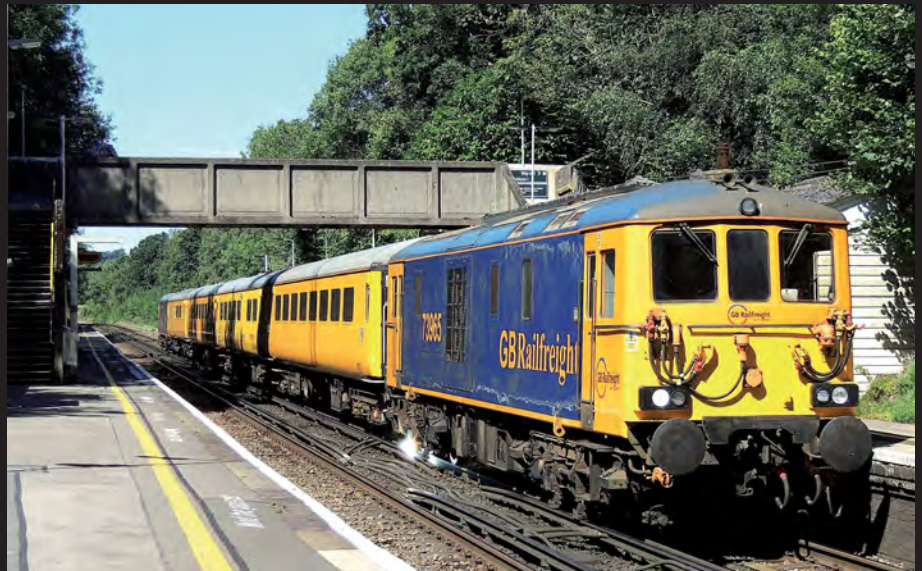
GB Railfreight operates two different types of Class 73/9. Those allocated to its freight and infrastructure train duties have been rebuilt with a pair of Cummins 750hp engines in each locomotive, as well as the capability to take power from the third-rail. On August 23 2015 73965 arcs on the third rail at Balcombe at the head of a Network Rail test train. A.M. Vaughan/Railphotoprints.uk.
