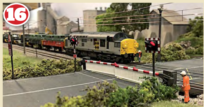
16 The Train-Tech working crossing lights were the final part of the jigsaw to be added. 10mm diameter holes were drilled through the baseboard to accommodate them and they were then connected to the DCC power bus under the layout to bring them into service. For a full installation guide to Train-Tech's crossing lights, see HM125.
