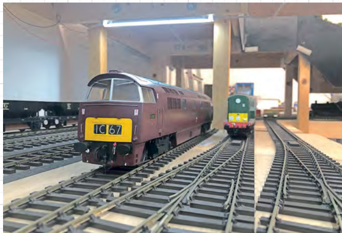
The siding stabling the 'Western' can be powered by analogue or digital while the rest of the depot is solely powered by DCC. Changing the points against the siding with the 'Western' isolates it from the main power feed.
