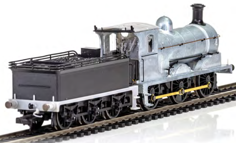
Above: The 'J36' features a fully detailed cab interior as well as a support for the weather sheet.
