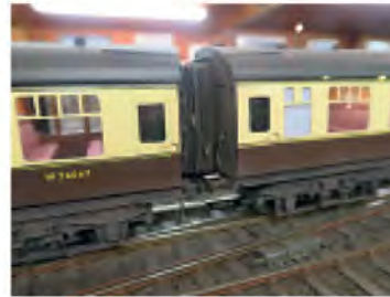
Magnetic coupling corridor connections
