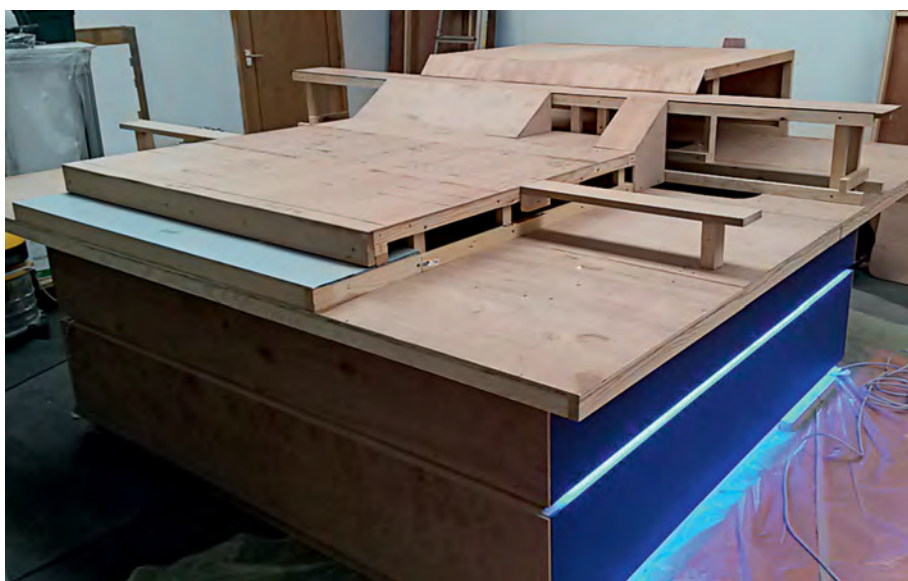
The multi-level baseboard design is shown clearly in this early construction view. The total size is 8ft x 8ft.
