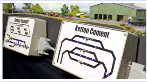
Point control is via servos which are operated from conventional control panels. The two panels control the scenic area (left) and rear storage yard (right).
