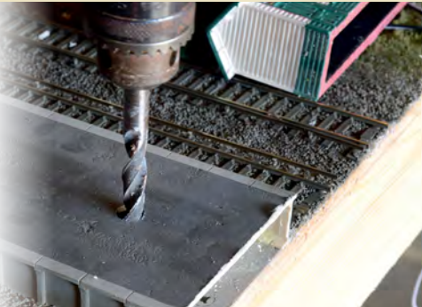
Having drilled the hole and fed the wire through this building is ready to reinstate on the platform. Initially we temporarily positioned all the buildings to check for light leaks.
