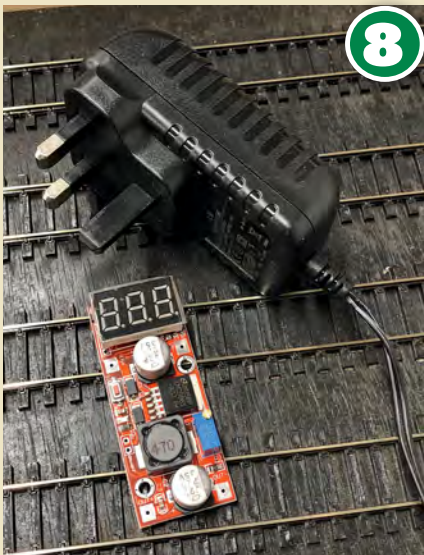
Dapol's signals require a regulated voltage to ensure their safe operation, but fortunately 12v power supplies and variable regulator circuits are cheap to buy – this pair cost just £18 from Amazon.
