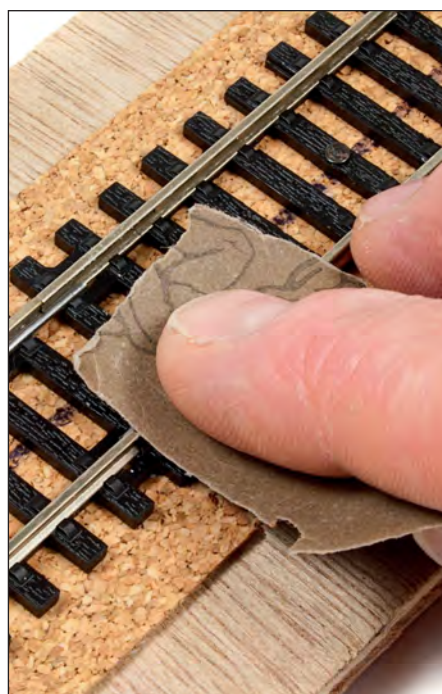
A gentle rub with fine grade wet and dry paper soon removes any rough edges or burrs.
