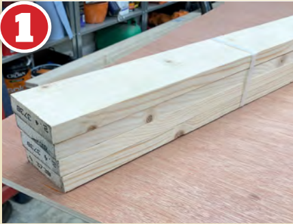
1 The raw ingredients for a simple 4ft x 2ft (1,220mm x 610mm) baseboard: a pack of 18mm x 69mm planed softwood in 2,440mm lengths and a cut to size piece of 9mm plywood.
