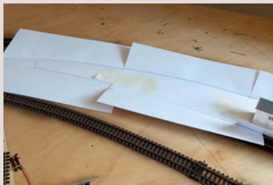
Above: Paper templates allow bases to be cut from 12mm MDF. Below: Wills stone plastic sheet was cut into strips for the platform faces while an airbrush was used to colour the final surface.
