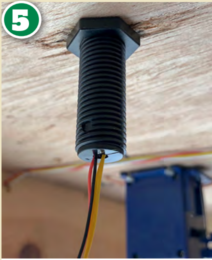
Undemeath the board, wind the securing nut back onto the threaded base to secure the signal in place. Don't over-tighten the nut as it can put strain on the mechanism – finger-tight is perfectly acceptable.
