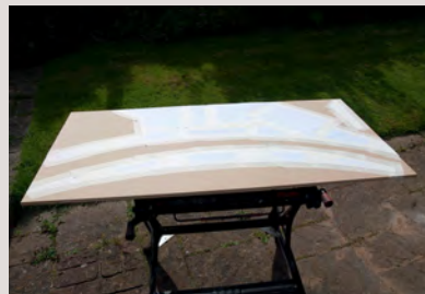
Above: Paper templates allow bases to be cut from 12mm MDF. Below: Wills stone plastic sheet was cut into strips for the platform faces while an airbrush was used to colour the final surface.
