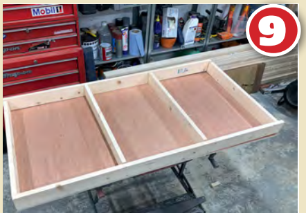
9 Laying the framework out dry means we can check that everything will fit together as planned. This is how the baseboard will look from underneath. Once complete it will be turned over to reveal its smooth and level plywood surface.
