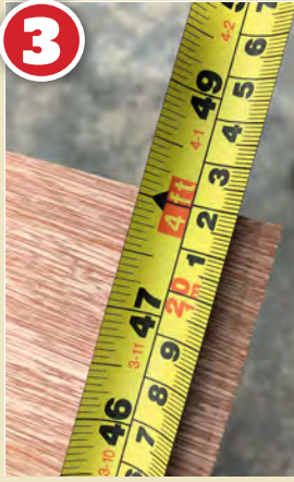
3 Begin by checking the measurements of the baseboard top – just because the DIY store said it was the size you wanted doesn't mean it will be exact on all four sides. In this case the length was identical on both sides at 1,220mm (4ft).
