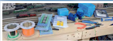
Wiring of the new Cobalt IP digital point motors was carried out swiftly. A handful of analogue Cobalt motors were also used requiring DCC Concepts Cobalt accessory decoder boards to operate them.
