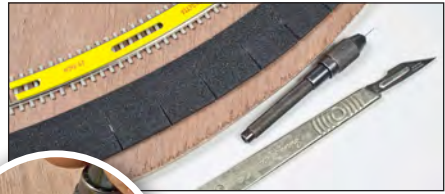
Left: Tracksetta is an extremely useful range of gauging tools designed for use with flexible track in 'OO' and 'N' gauges. An 'N' gauge Tracksetta of 15in radius is shown. It has slots along its length to enable track pins to be used.
