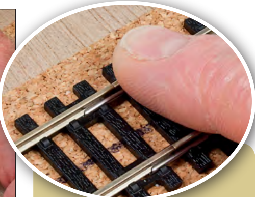
Inspect the rail joiners for misalignment and run a finger over them to find any rough spots that could prevent trains from running smoothly over the layout.
