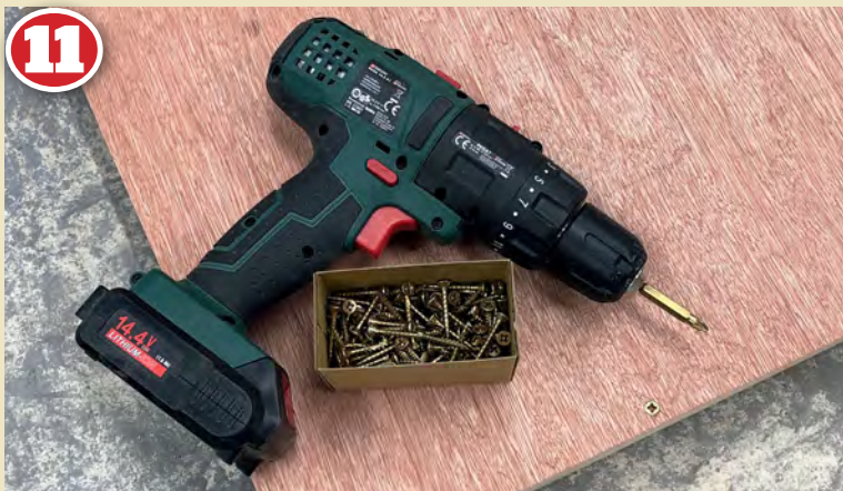
11 Having positioned the first long side timber under the baseboard top, it was then screwed in place with 4.0 x 30mm twin thread wood screws as well as the adhesive.
