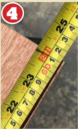
4 Repeating the process for the width showed that the panel was slightly wider than we had expected. This isn't a problem for this project, but it does mean we need to accommodate this in the cross-members underneath the board.
