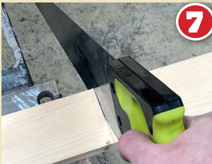
7 We can now move to cut the long sides using a handsaw. If you are confident with cutting timber you can do it freehand as here or alternatively use a mitre box to ensure a consistent 90 degree angle in each cut.
