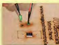
LEDs push into rear panel.
