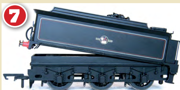
Raise the rear and slide the chassis rearwards to disengage the lug at the front.
