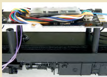
14 There are few large components on the upper surface of the PCB so the decoder can be fitted here.
