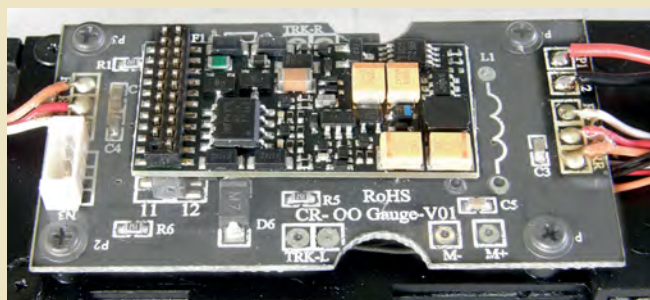
11 This shows the PCB (lightened for clarity) with the MX644D sound decoder fitted. The white connector shown on the left of this picture is the connector for the cab lighting. I reconnected the wiring plug and refitted the body to complete the installation.
