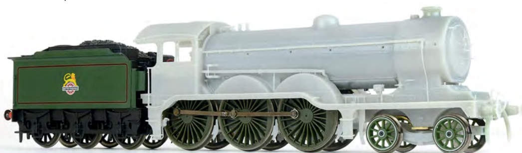
Above: Hornby's newly announced Holden 'B12' 4-6-0 was shown as a stereo 3D printed sample at the Warley National Model Railway Exhibition in November coupled to a standard Great Eastern short wheelbase tender.
