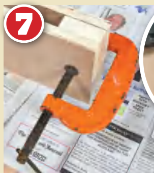
7 A close up of the frame member assembly, damped securely whilst the wood glue hardens.
