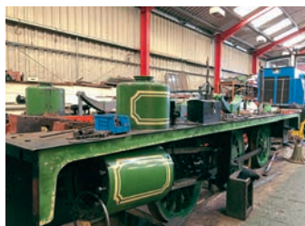
Slough Estates Ltd No. 3 under overhaul in the workshops at the Middleton Railway.
