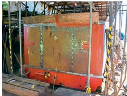
...while in the yard, the tender has seen new metalwork on the tank welded into place. It is hoped that both of the society's locomotives will be in steam together for a brief window in 2028, when No. 506 is due to be withdrawn.
