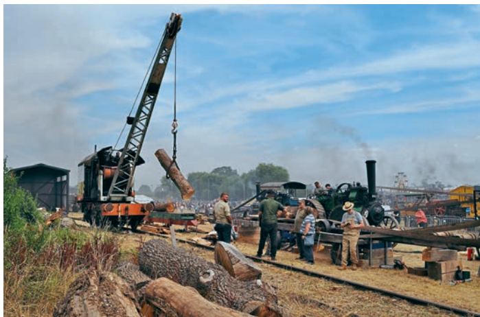
A Grafton steam crane lifted logs onto sawing equipment each day, the machines being steam-powered by the flywheel of traction engines.
