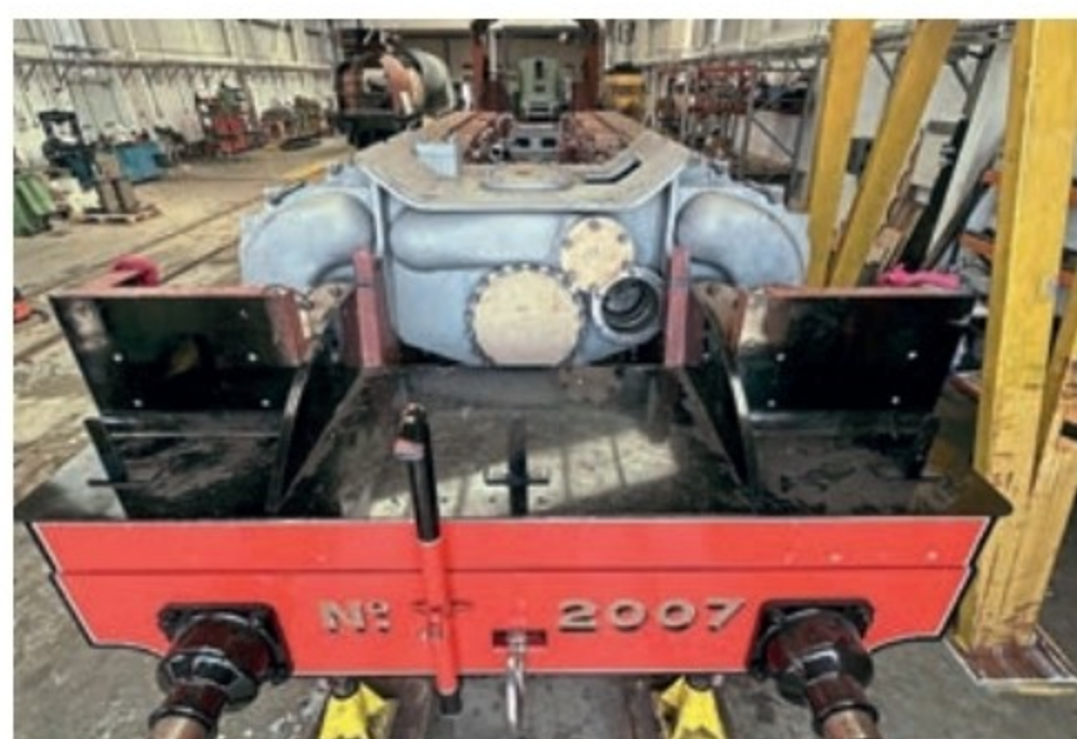
Three-cylinder monobloc fitted to Gresley P2
