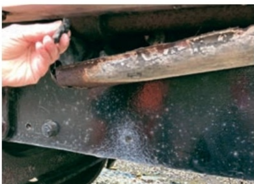
Above: The original ashpan beneath Balmoral . SALLY CLIFFORD
