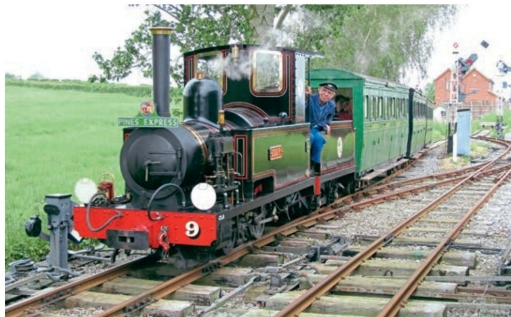
Seen heading the 'Pines Express' – recalling the legendary Somerset & Dorset named train which ran along the route on its journeys from Manchester to Bournemouth between 1901 and 1967 – along the Gartell Light Railway on May 31, 2014 is 0-4-0T+T No. 9 Jean, which was built by Alan White in 2008.
