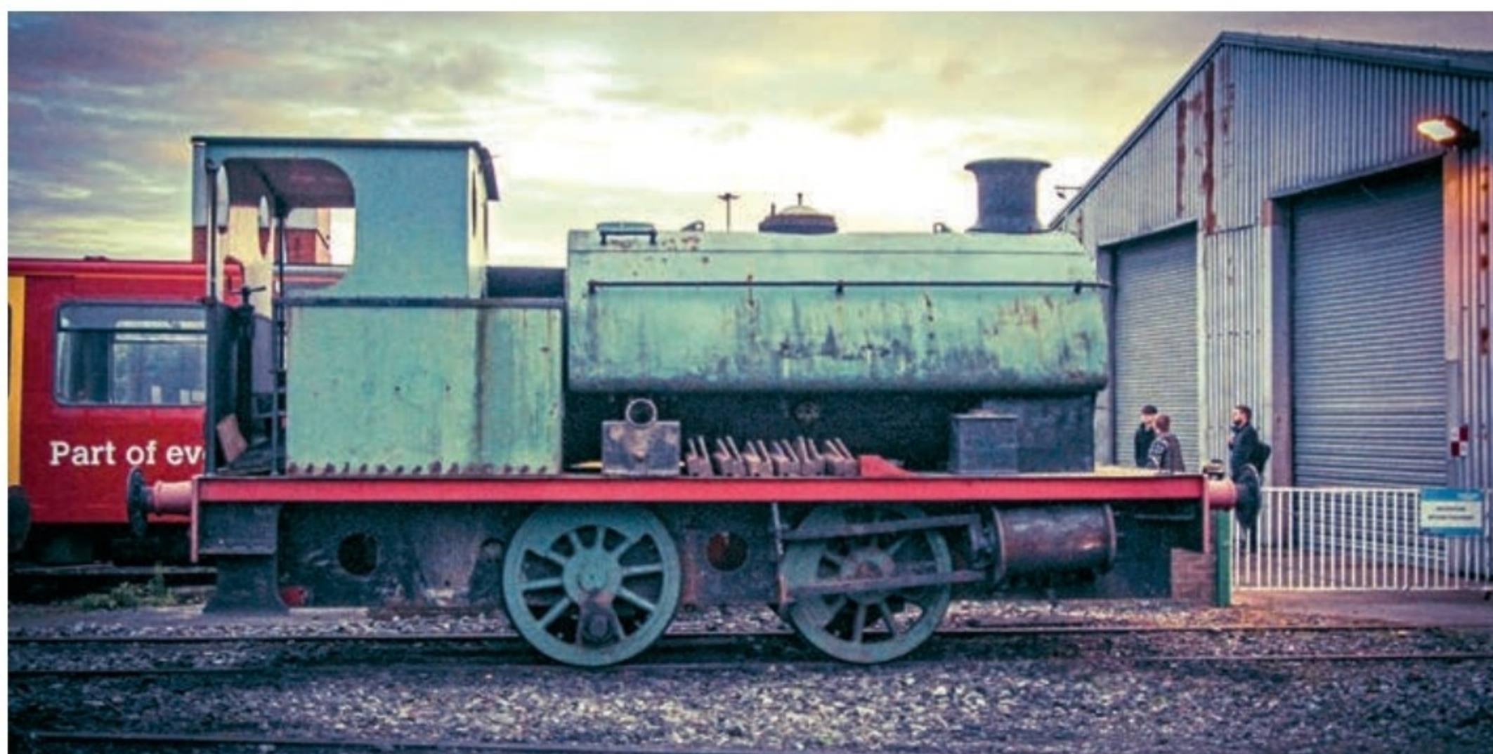
Ex-Blyth Harbour Commission Hawthorn Leslie 0-4-0ST No. 2918 of 1912 No. 2 Pony at the North Tyneside Steam Railway on June 5. The locomotive, which last steamed in 2004, is currently being worked on by apprentice volunteers passing down the skills to restore and fix old steam engines. JAMES GROUNDWATER
