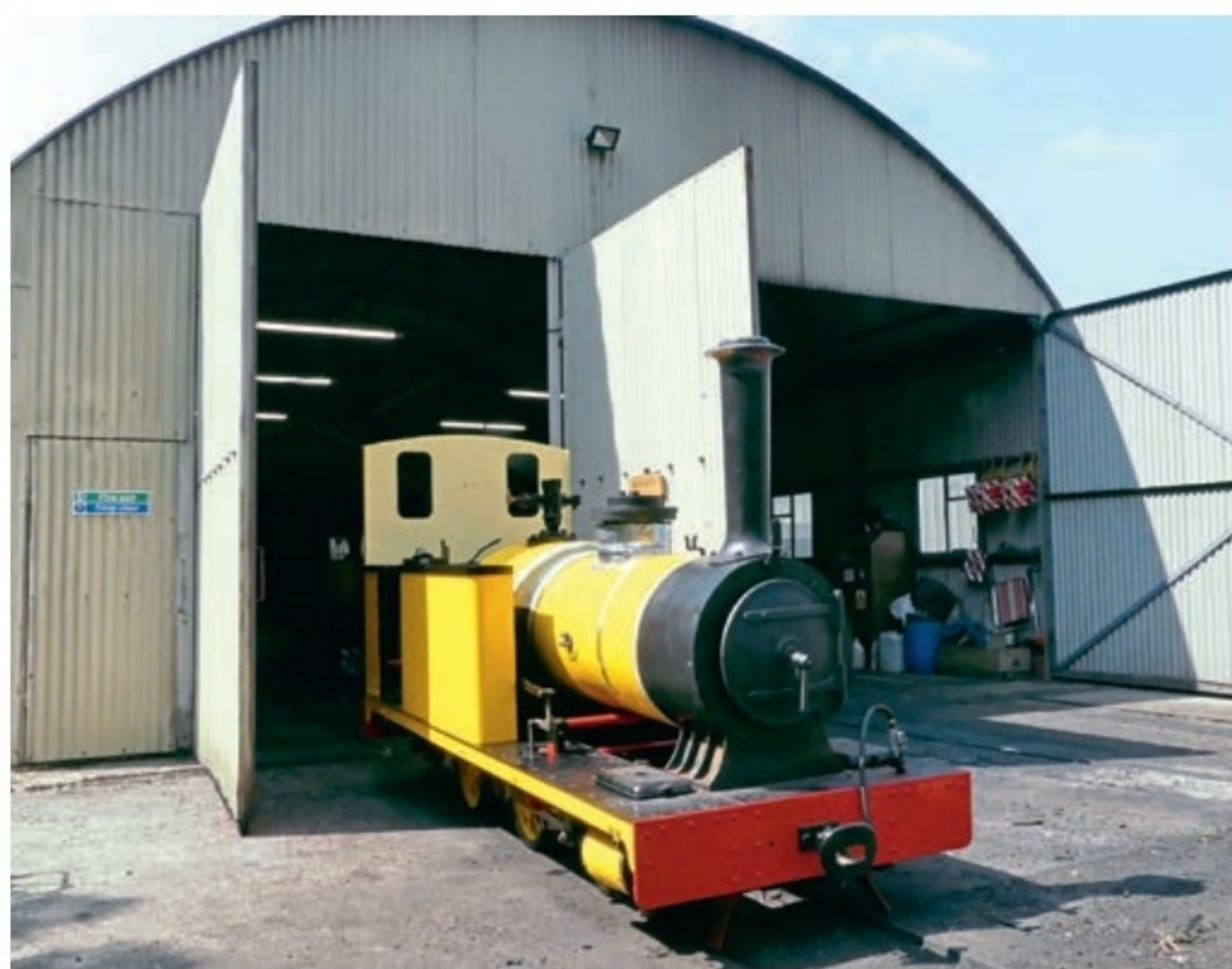
During the Amberley Museum Railway's July 18/19 summer gala, Bagnall 2-4-0T Polar Bear was brought out for static display. Last operational in October 2022, it has been undergoing a thorough overhaul in the museum's workshops and in recent months has started to resemble a complete locomotive once again. There is still much to do to finish reassembling the former Groudle Glen Railway resident, but it is hoped that it will be ready for Amberley's 2027 spring gala. Donations are sought at www.amberleymuseum.co.uk/support-POLARBear PHIL BARNES
