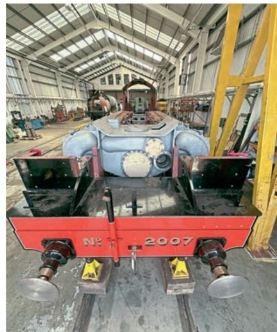
Right: The monobloc sitting inside the frames of Prince of Wales . A1SLT
