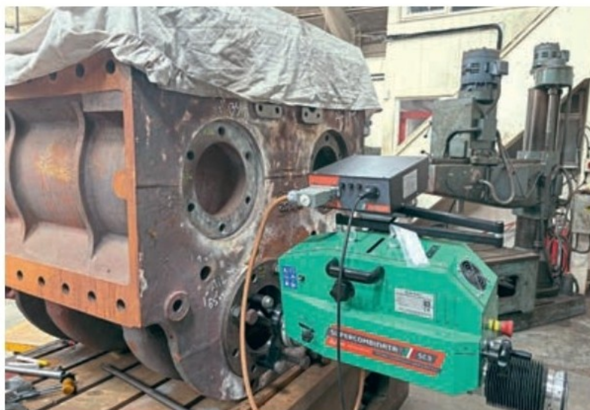
The J21 cylinder being bored at Loughborough. TOBY WATKINS
