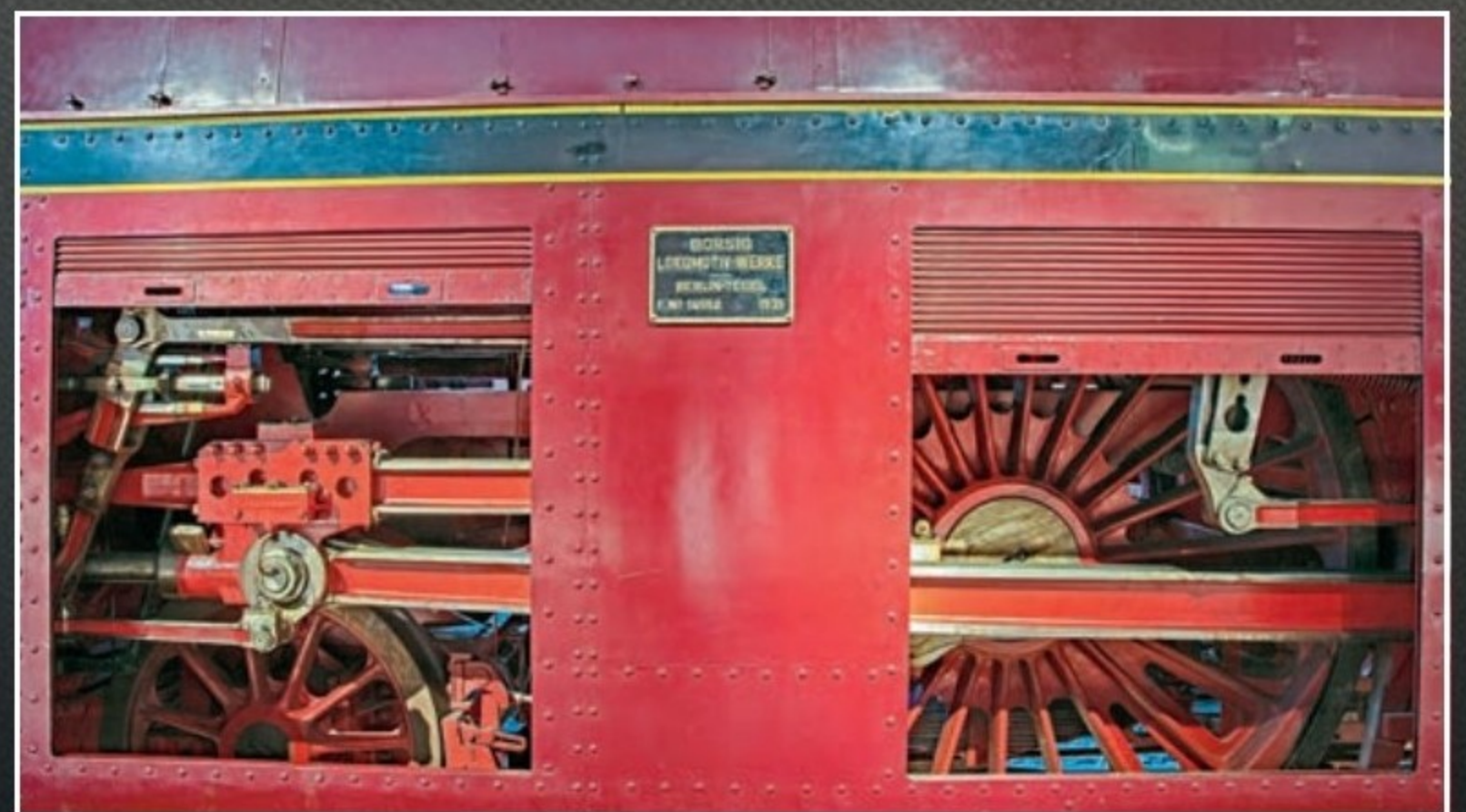
The driving wheels of No. 05 001, with access for oiling and the builder's plate.
