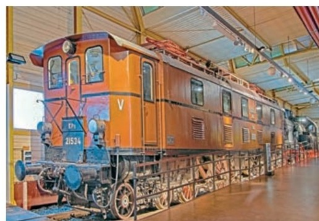
Bavarian Class EP 5 Bo-Bo electric No. EP5 21534, the sole survivor of a class of 35 which hauled heavy passenger trains.
