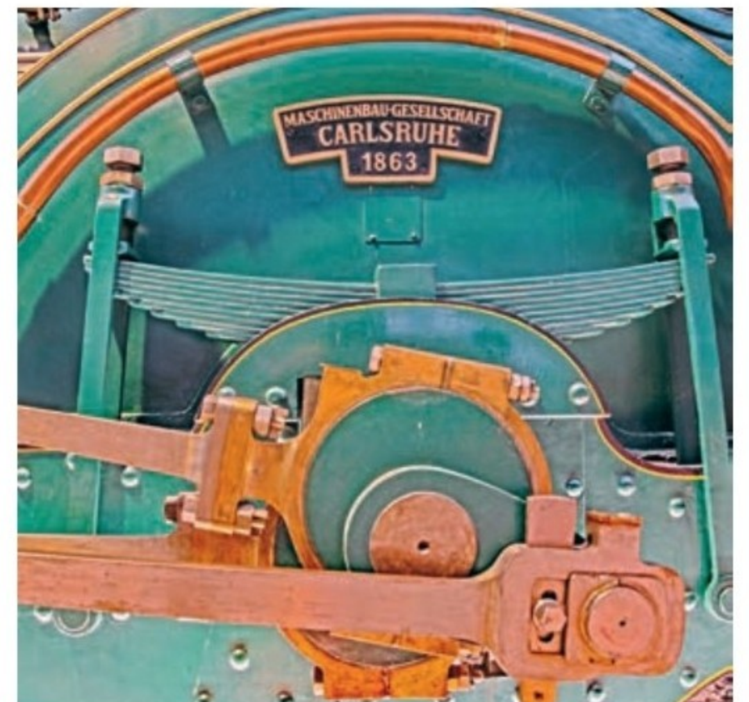
Builder's plate and centre driving wheel of Phoenix .
