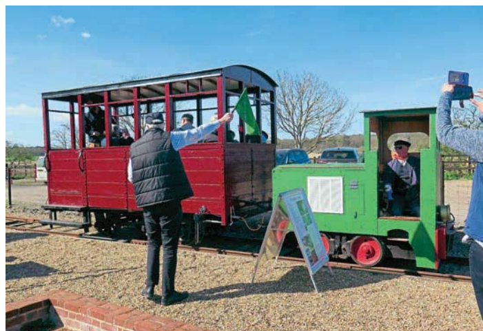
Greenwood & Batley battery-electric locomotive Helen hauls an Easter service at Blythburgh station. HSNGR
