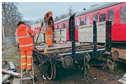
Five-plank open No. 24361 was transformed from a frame and rotting wood (left) into a nearly complete vehicle (right) in a matter of weeks, while LMS van No. 311671 received new doors in addition to a repaint itself. BOTH: DOUGLAS HEBSON
