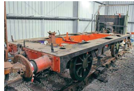
Consideration is being given as to whether the stalled overhaul of SECR P class No. 753 will resume before work on Knowle begins. Currently a kit of parts, recent inspection suggests that its overall condition may not be as bad as initially feared.
