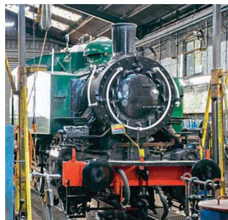
Overhaul of S100 0-6-0T No. 65 Maunsell is nearing completion at Rolvenden, with the locomotive expected to be completed by the summer.
