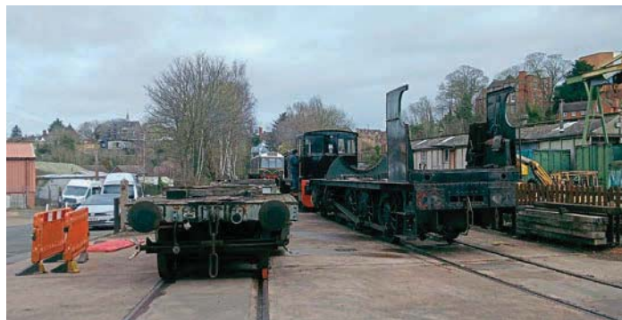
Below: ...and the rolling chassis (right) outside later that same day following the removal of the boiler as its overhaul gets underway. BOTH: 2857 SOCIETY
