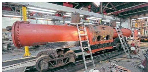
Left: The boiler for Merddin Emrys at Boston Lodge, where it has been overhauled in just five months. Ff&WHR
