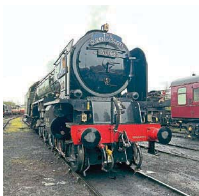
Left: Tornado with front-end features painted black to recreate the feel of an A1 in the 1960s. It has since run in this guise back on the main line. A1SLT
