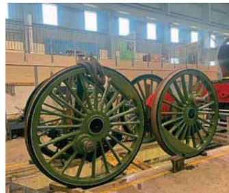
The locomotive's driving wheels, which have been painted into an LNER green top coat. TALYOR SHAW/SRPS
