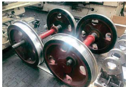
Above: The wheelsets' tyres have been turned so that the profile is correct for safe passenger running. WSVR
