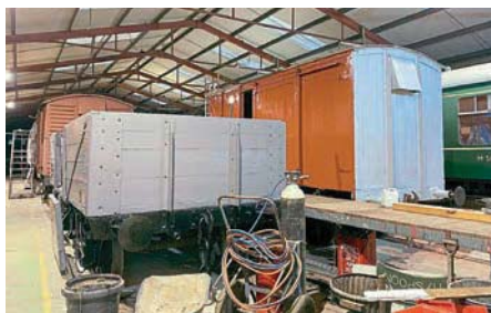
Five-plank open No. 24361 was transformed from a frame and rotting wood (left) into a nearly complete vehicle (right) in a matter of weeks, while LMS van No. 311671 received new doors in addition to a repaint itself. BOTH: DOUGLAS HEBSON
