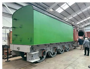
The newly assembled P2 tender. A1SLT
