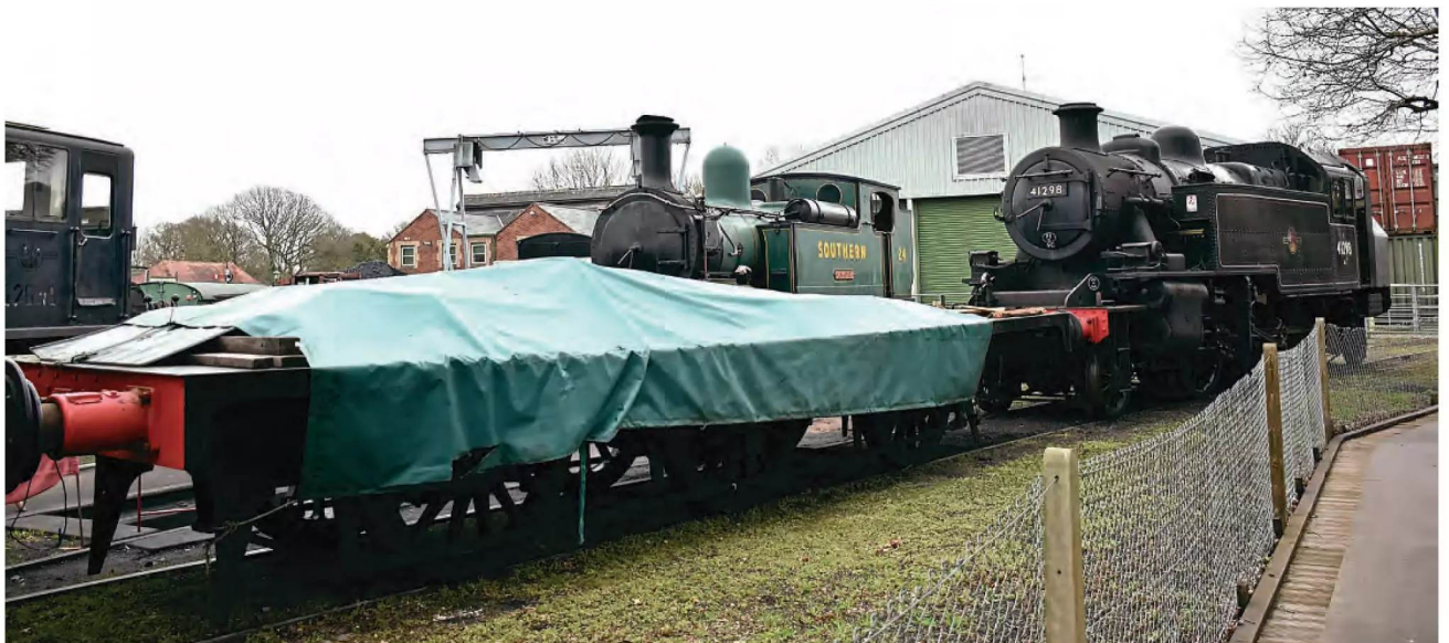
Above: The frames for E1 No. 110 Burgundy (which will adopt the guise of W2 Yarmouth) sit sheeted in the yard at Havenstreet awaiting the new boiler to be delivered. This is expected to be in early 2025, with a return to steam estimated for 2026. Behind is flagship LSWR 02 No. 24 Calbourne up on stands (top), which has had its wheels sent away for new tyres to be fitted – the first time this has had to be done in preservation. To the right, Ivatt No. 41298 awaits its turn in the overhaul queue.
