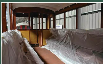
The beautifully restored Ryde Pier tramcar will soon gain a reconstructed trailer, which has had a new body built by local boat builders and fitted out by railway volunteers on a replica chassis. Once completed, the rear driving end in the first car will be removed. With hopes of being completed by the end of the year, it will prove an invaluable asset to the railway for low season workings.
