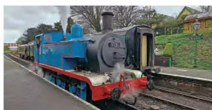
Converted from Hunslet Austerity 0-6-0ST No. 3781 Linda in 1994, the Mid-Hants Railway's Thomas returned to service in March after an overhaul that saw new cylinders fitted – a preservation first for an example of this class. RICHARD BENTLEY/MHR
