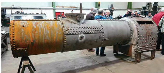
Above: The boiler of No. 19B minus its inner firebox on display for supporters at Statfold Barn. DTLT
