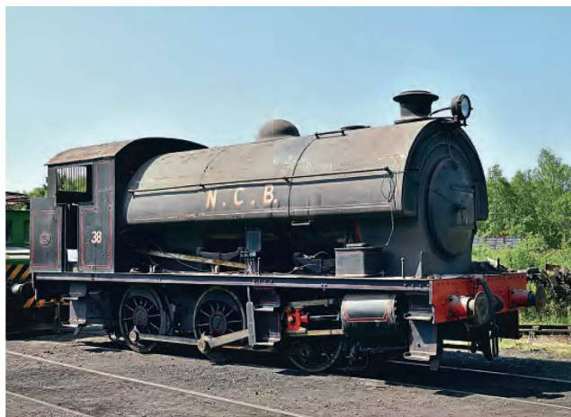
Robert Stephenson & Hawthorn 0-6-0ST No.38 before it entered the workshops, where it is now dismantled and under overhaul.
