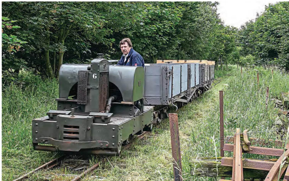
About to return to the task they were built for 108 years ago during the First World War, transporting materials across muddy, rain-soaked ground, trench railway wagons restored by the Lincolnshire Coast Light Railway Historic Vehicles Trust will take construction materials to the site of the new station. DAVE ENEFER/LCLR
