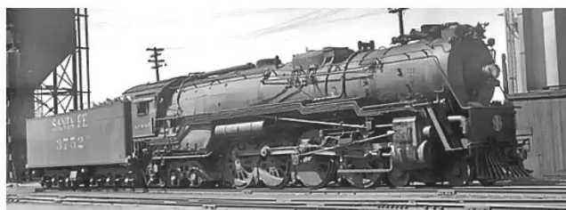
The Franklin Company further developed the Lentz valve gear and incorporated it into Atchison, Topeka and Santa Fe Railway Baldwin 4-8-4 No. 3752. The A1 Steam Locomotive Trust has obtained copies of the blueprints for this locomotive and the valve gear modifications and further adapted them into those for the new P2. A1SLT
