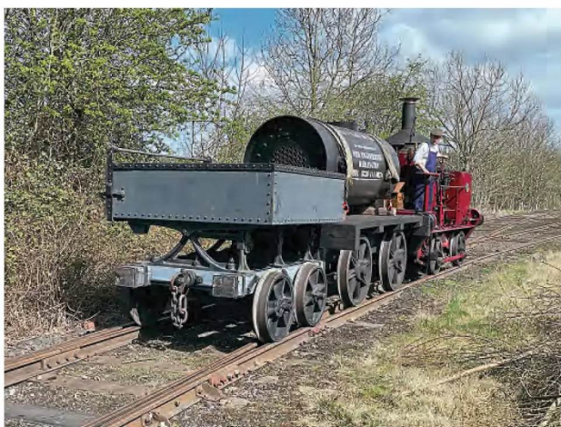
Coffee Pot No.1 on a goods rake which included the new boiler for NER K class 0-4-0T No. 559 being built at Beamish. The project to build a new example of the smallest standard gauge locomotive as produced by a main line company was launched in October 2022.
