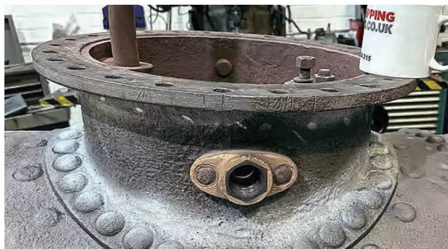
The Sharp Stewart 19b No. 4977 stamp found on the bronze flange fitting on the chimney driver's side. DTLT
