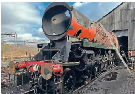
On February 15, the overhauled boiler from No. 34010 Sidmouth was steam-tested in the frames of No. 34053 Sir Keith Park at Tyseley Locomotive Works. This half of the locomotive then returned to Herston for its overhaul to continue. MALCOLM GARNER/SLL
