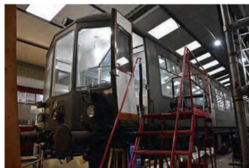
The EVR will soon boast both a single and two-car Derby Lightweight DMU, with driving trailer No. 79612 completed and finished in BR blue livery (above left), while the restoration of motor car No. 79018 continues in the workshops.
