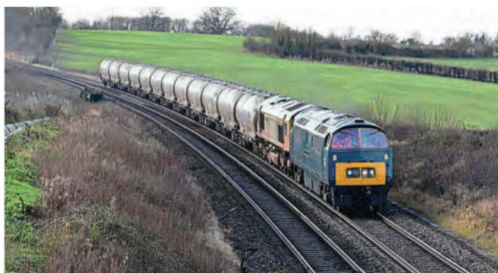
On the morning of January 10, the Diesel Traction Group’s Class 52 D1015 Western Champion undertook a loaded main line test run on a GB Railfreight-worked train following engine repairs, its first outing on the network since 2021. In December 2016, one of its MD655 engines failed, which was subsequently replaced by an overhauled unit in 2021 that also failed. Now fitted with two MTU 12V538 engines, the test was to prove them and, if successful, resume making the locomotive available for future railtours. PAUL FINCH
