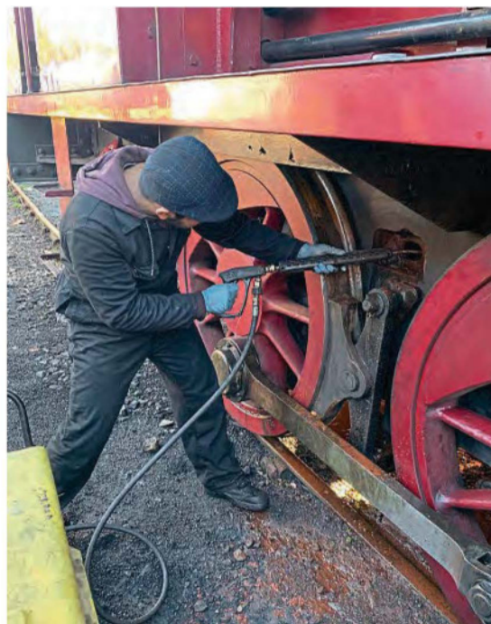
Boiler work: Muhammad washes out the boiler foundation ring, removing sludge and scale. DAVID GRINDLEY
