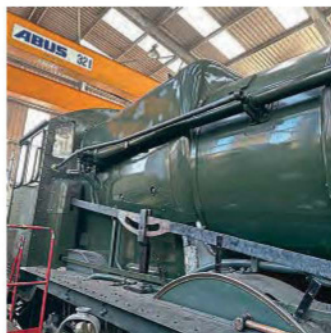
Handrails being fitted to the newly-painted Betton Grange inside Tyseley Locomotive Works on January 6. 6880
