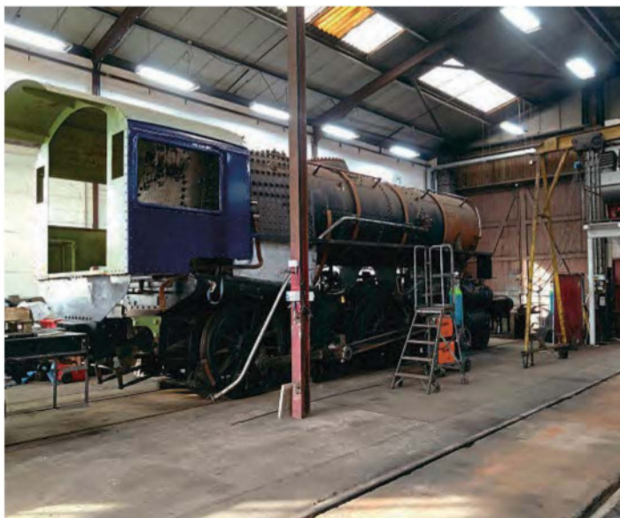
The overhaul of a third S160, No. 3278 Franklin D Roosevelt , continues in the workshops at Cheddleton. The boiler has recently passed a hydraulic test. CVR
