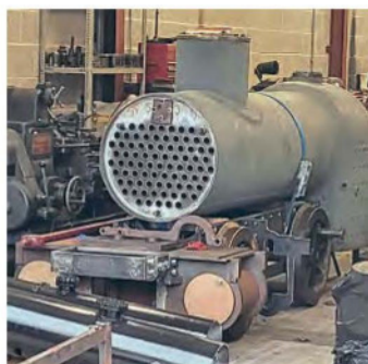
The boiler of the new Mountaineer on the chassis at North Bay Railway Engineering. 1863MLL
