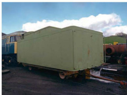
The newly built tender tank for No. 3278 in the yard at Cheddleton. CVR
