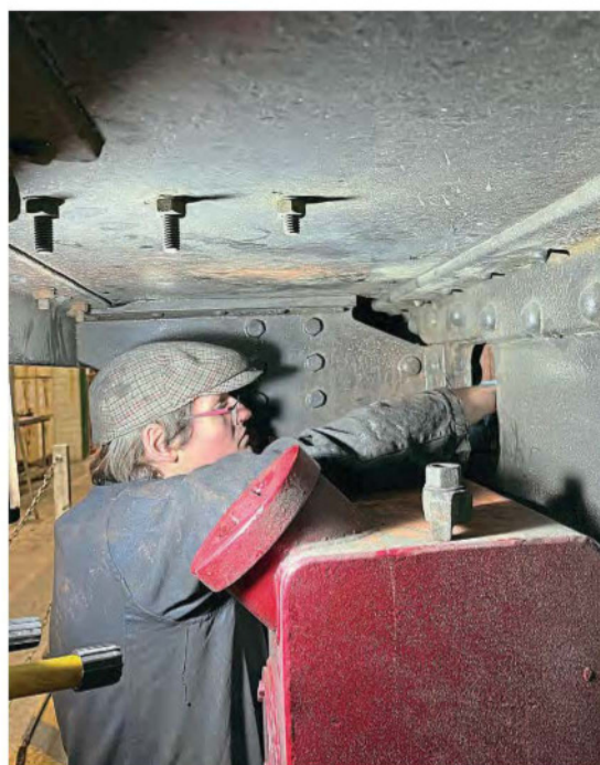
Practical: Tom fits a mudhole door with a new door joint. DAVID GRINDLEY
