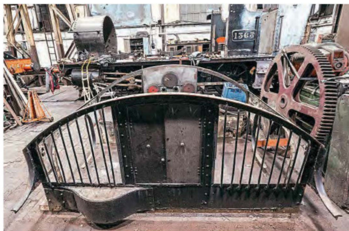
The upper part of the cab of No. 1363 being prepared for a new roof sheet to be fitted. The chassis is in the background, with a new coal bunker fitted. GWS
