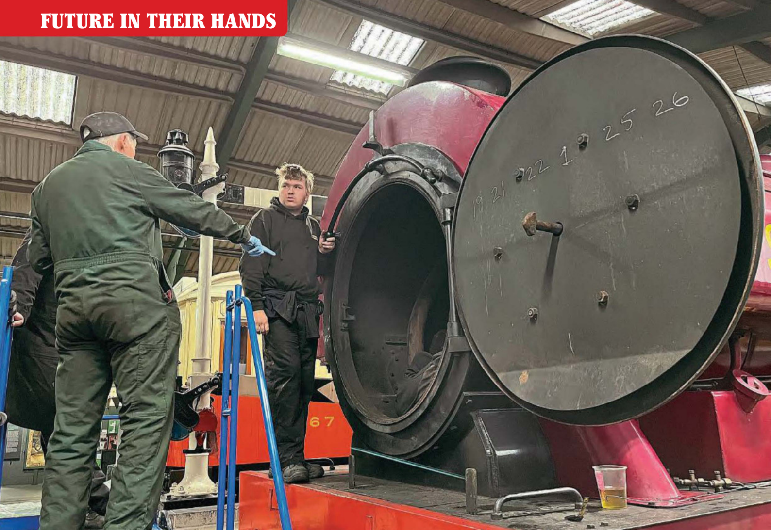
Taking it all in: Aaron Denny learns about the boiler with Tom Ashcroft and BESTT trainer Lawrence Donaldson, removing wash-out plugs in the smokebox during the BESTT Boiler Wash Out and Examination course at Stephenson Steam Railway. DAVID GRINDLEY
