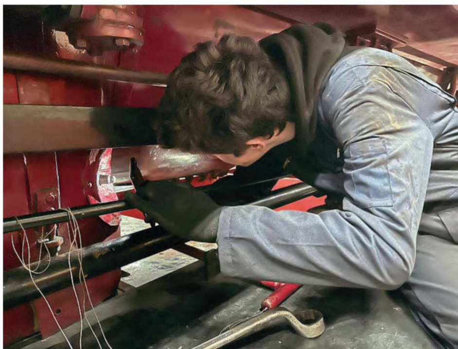
Hands on: Benjamin fits a mudhole door and checks alignment. DAVID GRINDLEY
