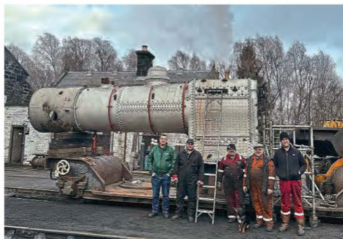
Volunteers who have been working on the overhaul of Ivatt 2MT No. 46464 were delighted with the news that the out-of-frames steam test was passed on November 22 at the Strathspey Railway's Aviemore workshops. CPCL
