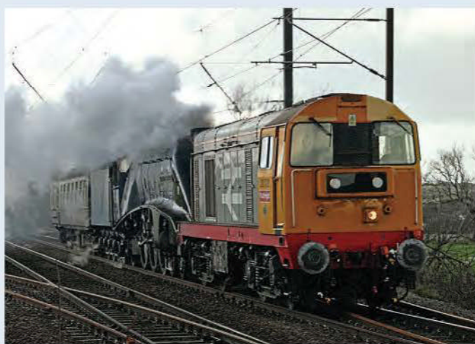
No. 60007 underwent a temporary fix after a valve failure so it could return to Crewe and is seen here at Wooden Gate, just south of Alnmouth, being hauled by Class 20 No. 20132 on November 27. LESLIE WHEELER
