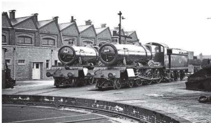
At Swindon Works, the GWR's two versions of 4-6-0s with 5ft 8in driving wheels: No. 7827 Lydham Manor , now on the Dartmouth Steam Railway, and No. 6879 Overton Grange , the last of 80 Granges built, until No. 6880. MIKE PEART
