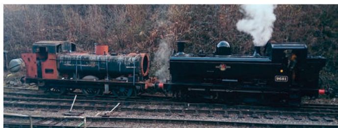
A stark contrast between two locomotives of the same class but in very different conditions. On March 10, newly overhauled WR pannier No. 9681 shunts its partially dismantled classmate and immediate numerical successor around the yard at Norchard to position it ready for the tanks and boiler to be craned off; this will allow a full assessment of the condition to take place. This will then help form the overhaul plan to return No. 9682 to steam. TOM HALFORD/DFLG
