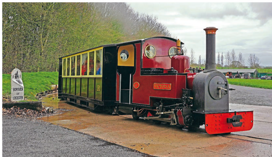
Statfold Barn's Spectacle of Steam was the first time that Exmoor Steam Railway-built 2-4-2T Victoria was used on public services, despite having been built 16 years ago. The 12 ¼in gauge locomotive was also operating on the venue's new Mease Valley Railway, which was opened at the March 18 event. GAVIN THOMSON
