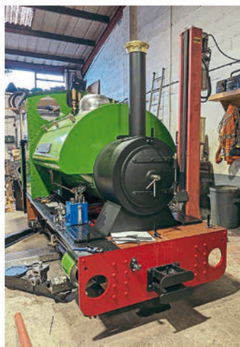
The new Perrygrove Railway saddle tank in the final stages of completion at the North Bay Railway Engineering Services workshop in Darlington.
