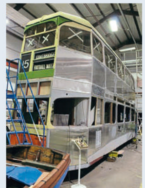
Glasgow Coronation tram 1245 with panelling complete and glazing underway, ready for the paintshop. HUGH DOUGHERTY
