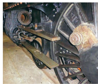
The new slide bars have been fitted to GWR 4-6-0 County Class No. 1014 at Didcot, where the locomotive will be on show coupled to its tender for the April 22 supporters' event. GWS
