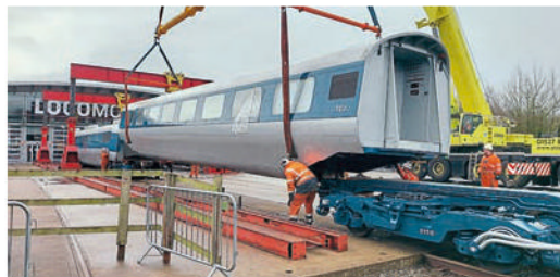
One of the APT-E centre carriages is lifted from its bogies during the reconfiguration process at the end of March. LOCOMOTION
