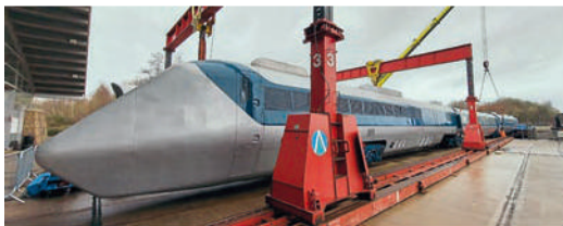
Outdoors for the first time since 2004, the BR APT-E was reformed at the end of March into a three-car unit. Supporting rigs and a crane supplied by Allelys are seen being prepared to conduct the lifting of one of the centre carriages. LOCOMOTION
