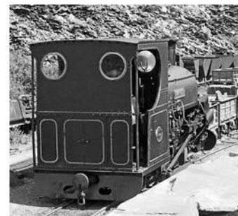
Above: Blanche at the quarry in 1960, giving a clear view of the cab backsheet that was originally fitted to the Hunslet.
