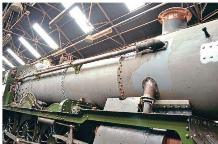
The vacuum exhaust pipe fitted to No. 6880 Betton Grange at Tyseley Locomotive Works. LYNN MOORE/6880 BERTON GRANGE SOCIETY
