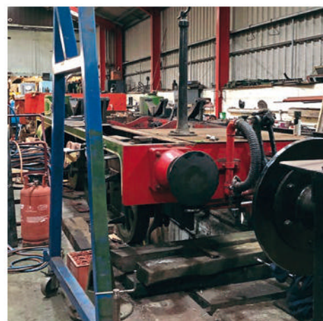
Above: The overhaul of Hudswell Clarke 0-6-0ST No. 1544 of 1924 Slough Estates No. 3 is currently work in progress, which volunteers continued in earnest during the build-up to the festive season. SALLY CLIFFORD
