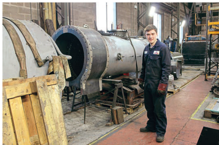
Jack Kerswill with a boiler for the Isle of Man Railway, made at Bridgnorth Works on the Severn Valley Railway as part of a large contract. LESLEY CARR/SVR
