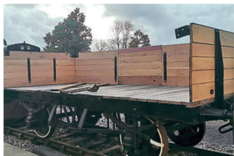
The Bluebell Railway's Bulleid open wagon is progressing well. The unpainted oak planking will remain as seen here, which will certainly stand out in the freight train. MATTHEW LANDER/BR
