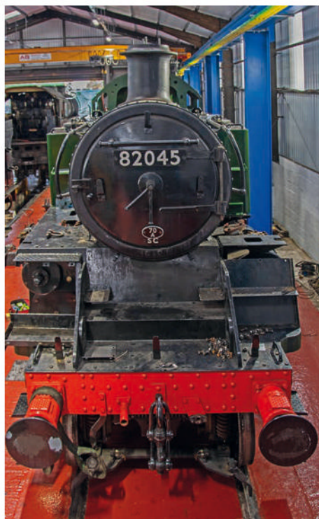
Pictured in Bridgnorth Shed on October 31, new BR Standard 3MT 2-6-2T No. 82045 is beginning to look more like its long-lost sisters, especially from the front with the fitting of its second tank and their painting in green undercoat. The 46th member of Robert Riddles' 82000 class – designed for light passenger, secondary main line duties and branch lines – was booked for display at this weekend's Warley National Model Railway Exhibition at the National Exhibition Centre in Birmingham (November 26/27). The boiler is under construction and further funds are needed: Visit www.82045.org.uk/index.html JOHN TITLOW
