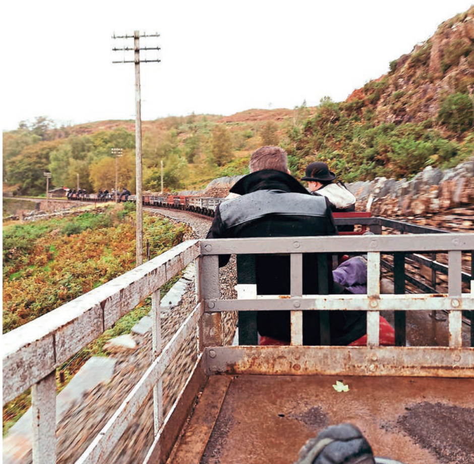
The downhill gravity working rounds Coed-y-Bleddiau curve as it prepares to stop clear of the track circuits at Garnedd Tunnel.
