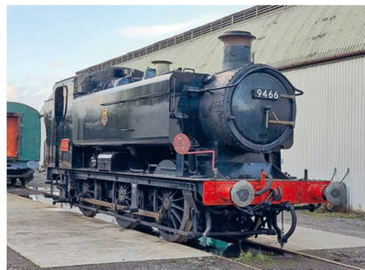
Jonathan Jones-Pratt's WR 0-6-0PT No. 9466 has passed its steam test following maintenance and now has a new 14-month boiler ticket which will allow it to participate in the West Somerset Railway's winter services if required. It has also retained its main line registration. WSR
