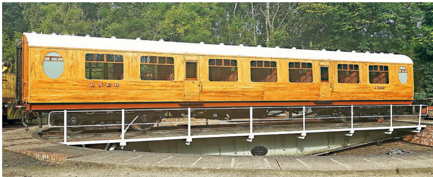
Earlier this year, the sole-surviving Thompson third corridor No. 1623 benefitted from having the 'scumble' (wood effect) livery refreshed, pictured here on the turntable at Pickering after outshopping from the Atkins shed. By no means a simple task, it took several weeks and entailed grinding out screws where the filler cap had 'popped' through the surface of the paint and replacing them with a longer stainless steel screw. The mustard colour base coat was applied to a rubbed-down surface and the scumble coats applied after. MURRAY BROWN
