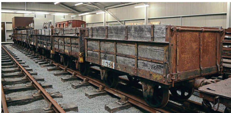
Converted from three-ton slate wagons pre-preservation, they were used out of Brookes Granite Quarry, which was located just north of the old Moelwyn tunnel.
