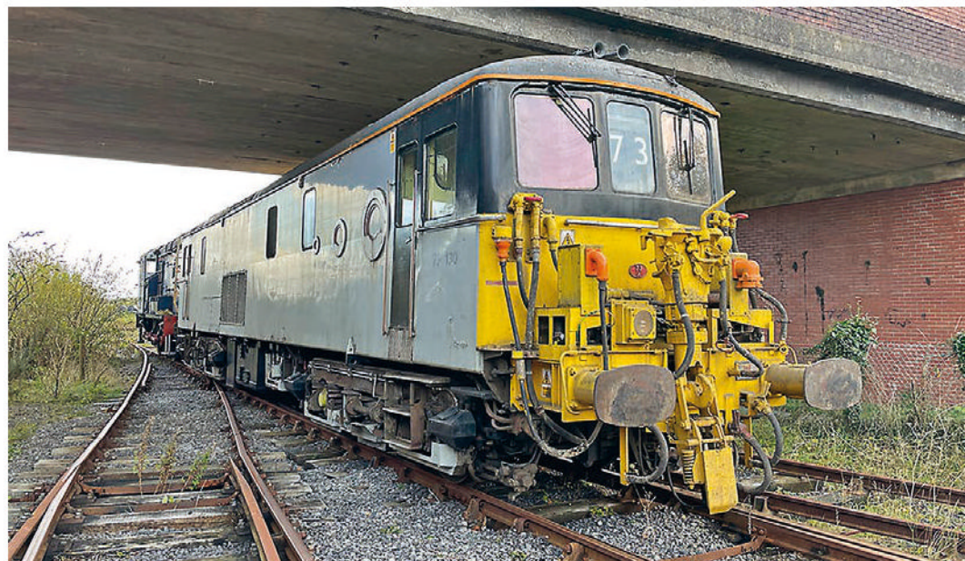
Class 73 No. 73130, complete with Scharfenberg coupling adaptors for Eurostar linking, newly arrived at Cynheidre on the Llanelli & Mynydd Mawr Railway on November 4. LMMR
