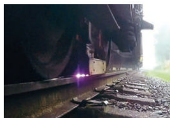
Slightly more subdued in brightness, one of the lasers used during the railhead treatment trials. NETWORK RAIL
