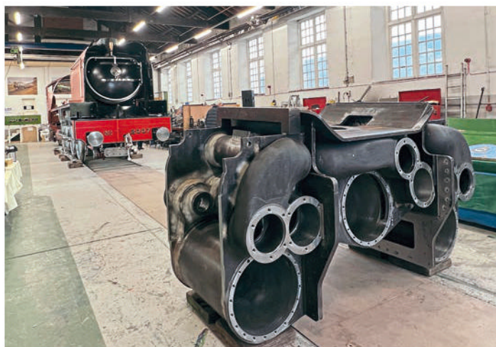
The monobloc for P2 2-8-2 No. 2007 Prince of Wales in front of the locomotive after being unveiled at Darlington. A1SLT
