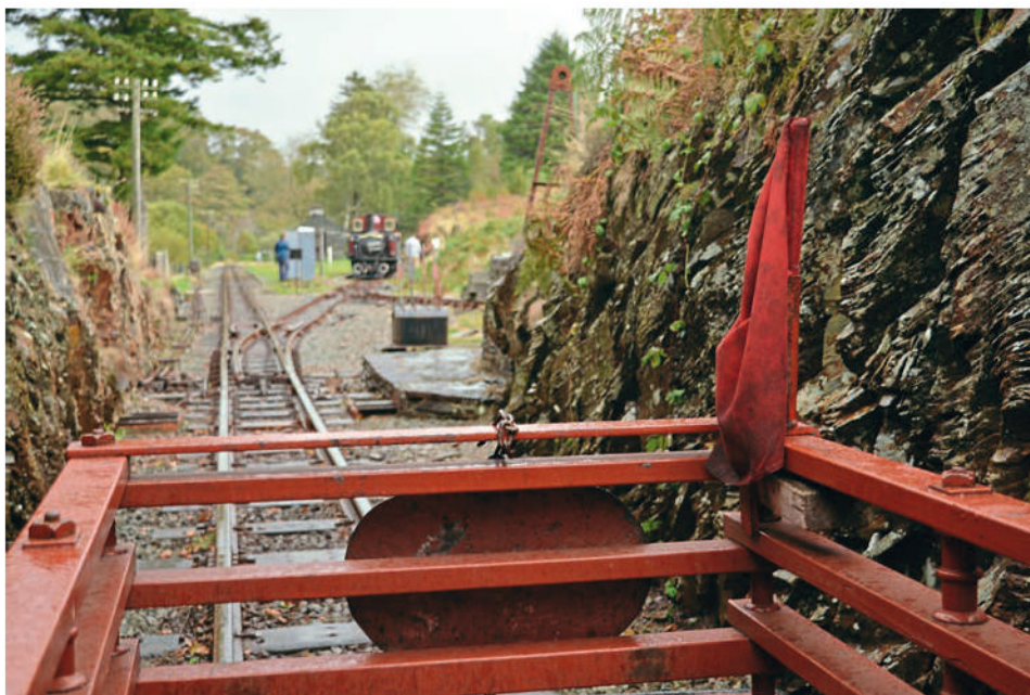
With the locomotive detached and run into the loop at Dduall, the flag and last vehicle board have been attached to denote the end of the train for the downhill run.
