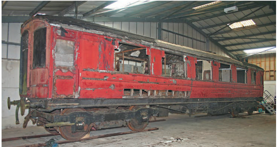
After almost a decade of outdoor storage, restaurant first open No. 22118 became the first vehicle to enter the Kirby Misperton workshops in 2021. Assessment is underway to determine the full extent of work required to restore it, which, as can be seen, will be quite a big task. MURRAY BROWN
