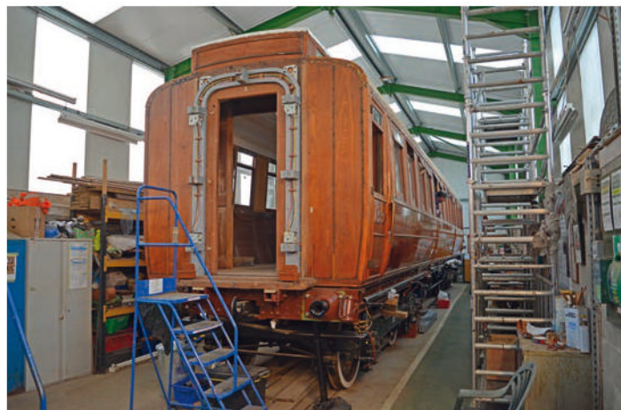
East Coast Joint Stock third class dining car No. 189 is undergoing restoration in the Atkins shed at Pickering. OWEN HAYWARD
