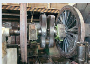
The Duke's crank axle on Tyseley's wheel lathe for profiling the new tyres in early September. C8SLT
