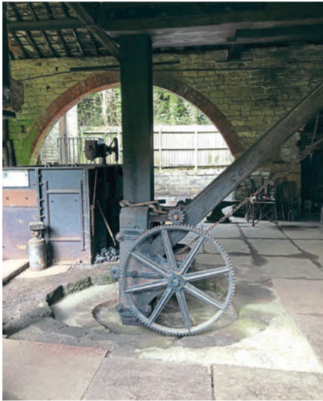
The crane inside Wortley Top Forge, which would have been used to lift railway axles. SALLY CLIFFORD
