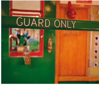
The guard's 'compartment' is simply one end of a motor car separated from the passenger bays by a bar, with a limited control panel and brake handle. OWEN HAYWARD
