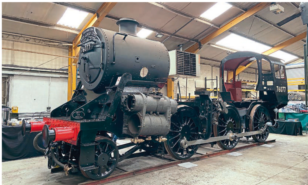
The 'kit of parts' including coupling rods and a cab comes together at in Loughborough. Much work remains to be done on the cab, however, and the number was a temporary addition for the open day. IAIN CROWDER
