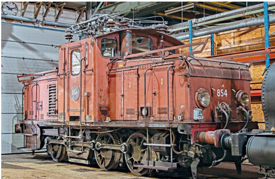
ASEA/Motala Ud No. 854 was of 1955 is one of 152 electric shunters built for use in both Sweden and Norway.
