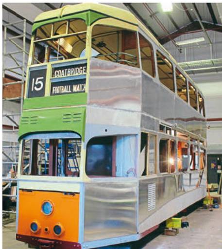
Could Glasgow Coronation No. 1245 be ready in time for the coronation of King Charles III in 2023? Panelling has been completed on the 1939-built car. HUGH DOUGHERTY
