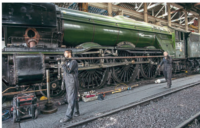
Boiler tubes removed during Flying Scotsman 's overhaul at Riley & Son (E) Ltd in Heywood. STEVE MORGAN/SCIENCE MUSEUM GROUP
