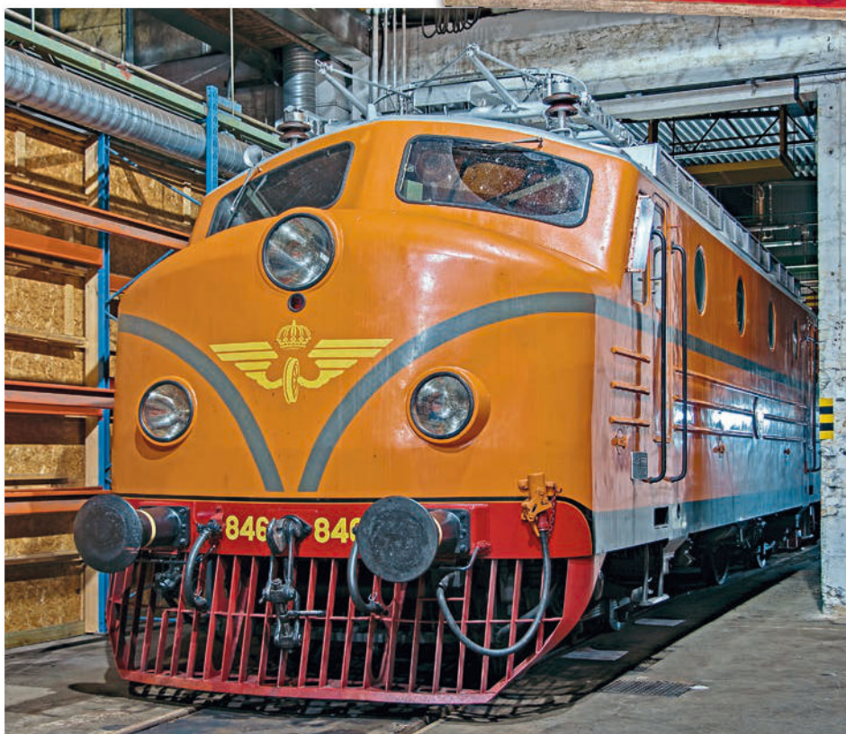
SJ Class Ra electric locomotives were built in 1955 and 1961 for on express trains, having a top speed of nearly 100mph. 5 of the 10 built survive.
