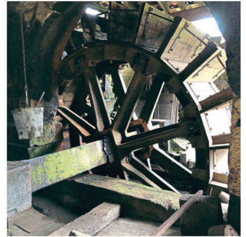
One of the water wheels which powered the production of railway axles at Wortley Top Forge – the only equipment that was used to power the machinery. SALLY CLIFFORD
