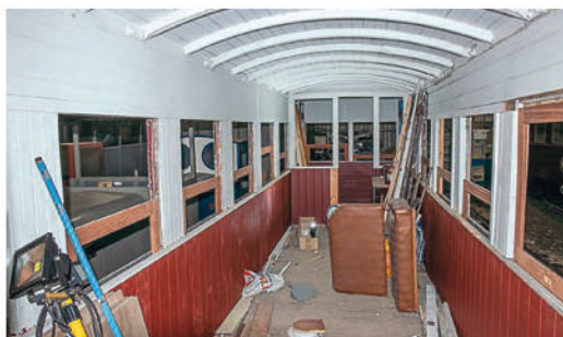
Restoration work already in progress on the interior of carriage No. 1, with new frames for the drop lights in which the safety glass will be installed. DAVID ENEFER/LCLR
