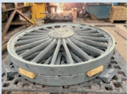
The new Patriot driving wheel castings. COOK CAST PRODUCTS/ LMS-PATRIOT PROJECT
