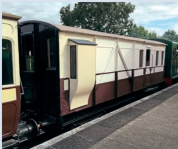
Luggage brake No. 422 has been converted from a Toad brake van. VTP
