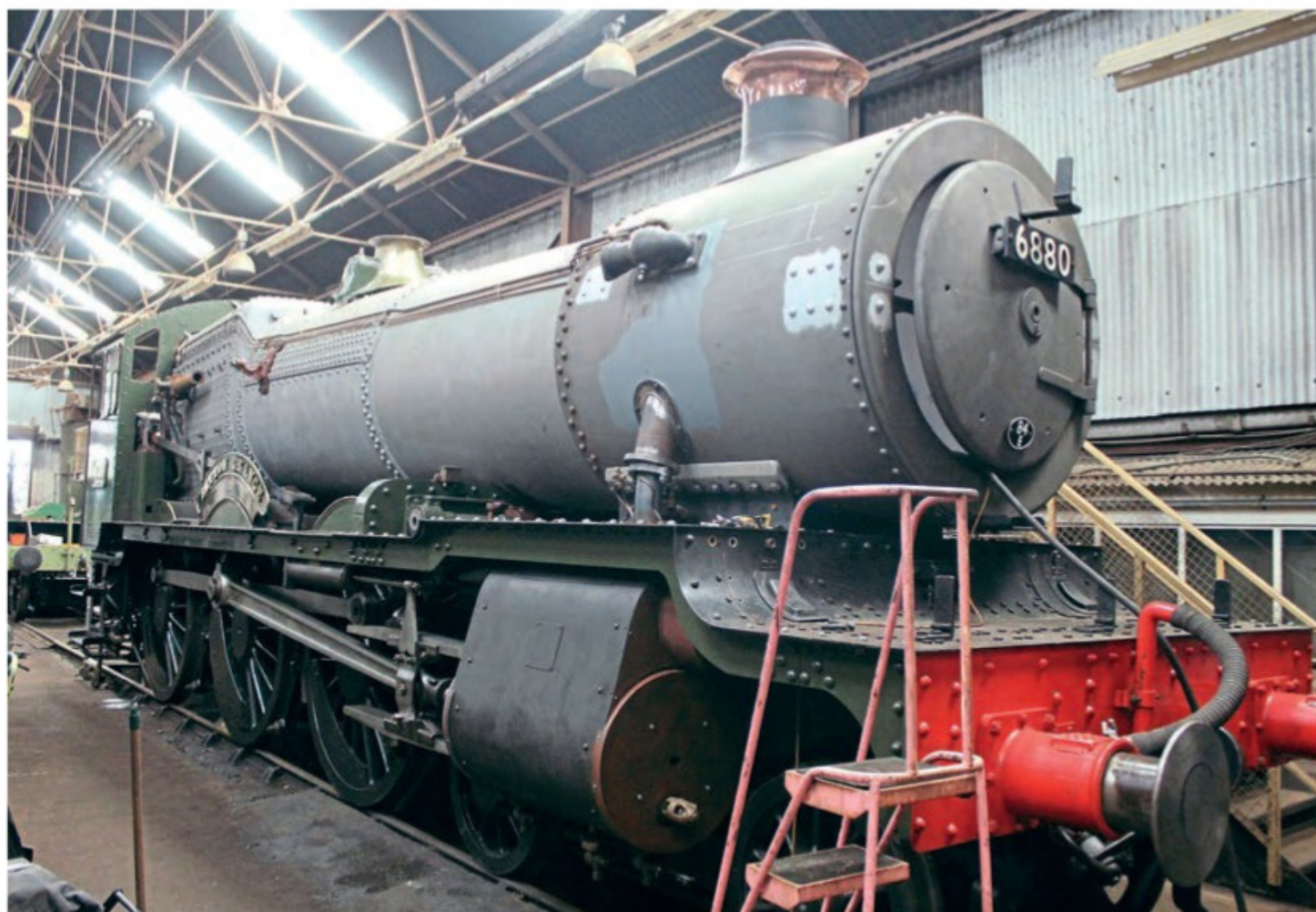
On May 30, No. 6880 Betton Grange made a rare excursion outside the Tyseley workshop to have its chimney craned into position. It is pictured back inside on June 10. The almost-complete 4-6-0 is now on course to steam for the first time this autumn. OWEN HAYWARD
