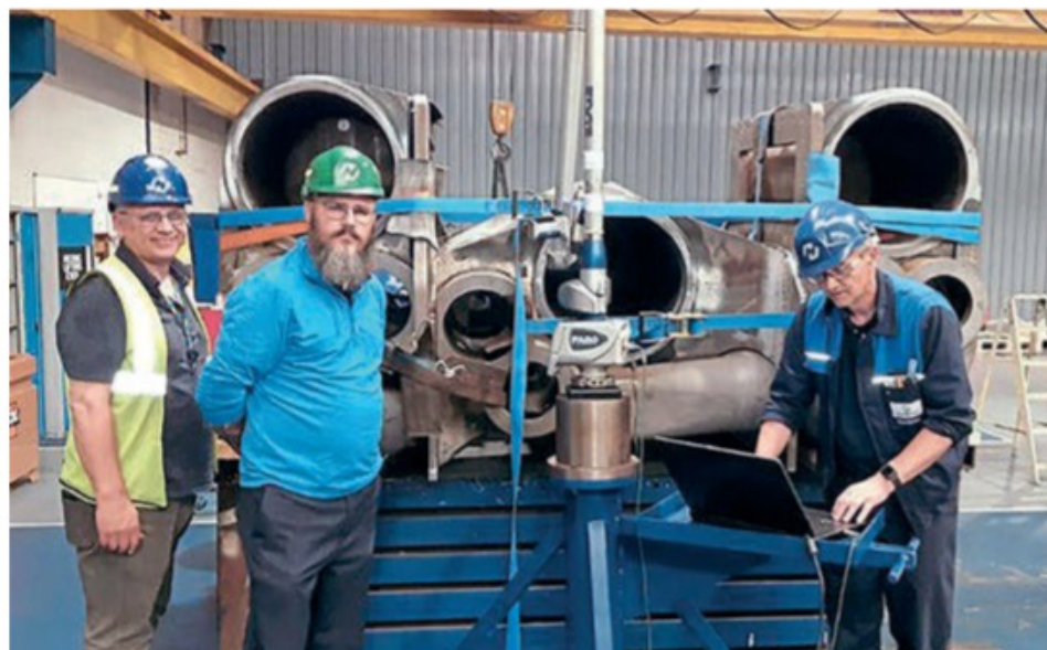
Measuring the front of the monobloc with the Faro arm on June 8. A1SLT
