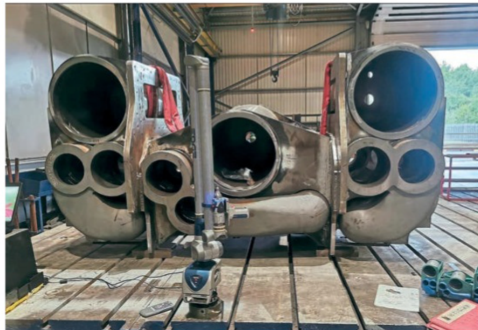
The three cylinders for P2 2-8-2 No. 2007 tack welded together at Howco for the first time, in advance of making the fitting permanent. A1SLT
