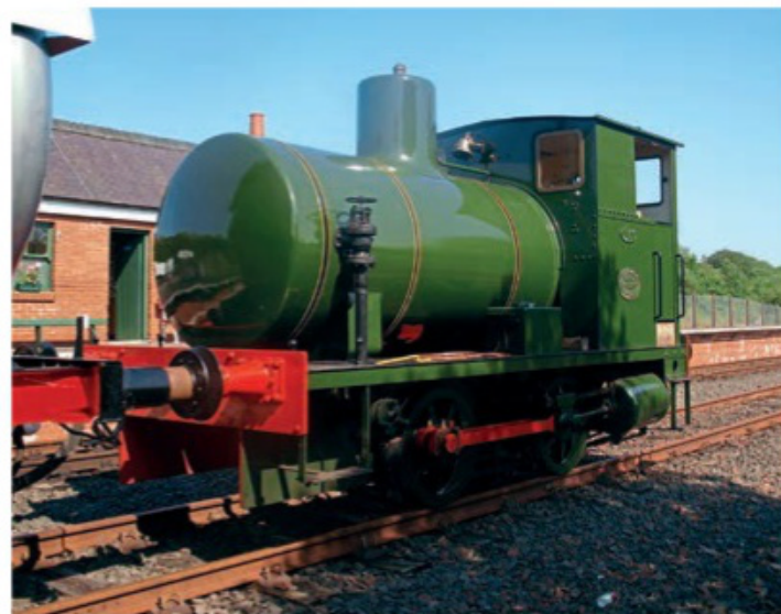
Barclay 0-4-OF No. 1952 of 1928, currently the sole working fireless locomotive in the UK. ARPG
