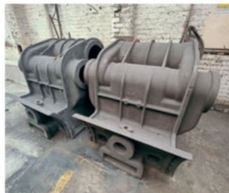
No. 3840's two cylinders at Hargreaves Foundry in Halifax. MIKE SOLLOWAY
