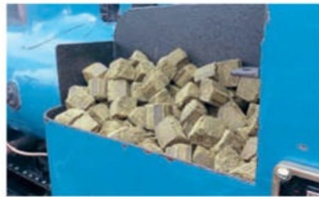
The rapeseed oil biomass briquettes being tested in Barclay 0-4-0WT No.6 Douglas on the Talyllyn Railway. STEPHEN THORPE/TR
