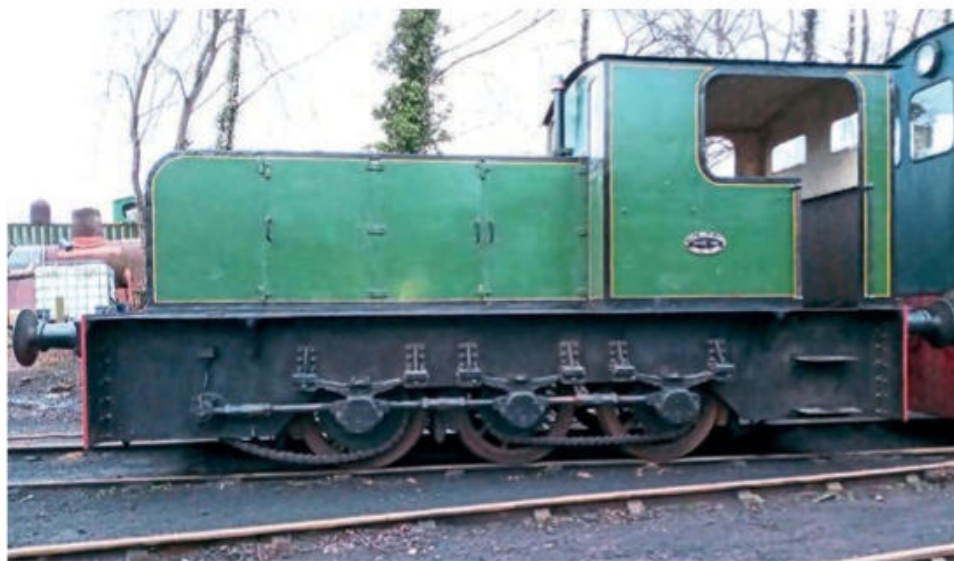
Rom River was the UK's first purpose-built standard gauge diesel constructed by Kerr Stuart in 1929. FR
