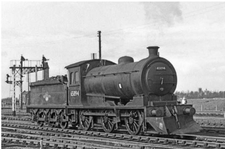
Snow use: As a reminder that the north of England climate can be cold even as spring approaches, J27 class No. 65894 sports a rather rudimentary but doubtless effective snowplough at York in March 1964. The 0-6-0, which was saved by the North Eastern Locomotive Preservation Group after its withdrawal in September 1967, will move south to the KESR next month to help out with the line's busy summer schedule. TRANSPORT TREASURY/JACK KIRKE
