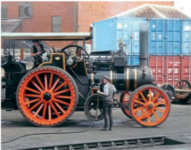
In attendance at Minehead station for the gala was Mike White's 1910-built McLaren 8hp traction engine No. 1148, which travelled from his Exmoor yard. Built for export to dealers Caccialanza & Bronzini in Piacenza, Italy, it was designed for direct ploughing and general heavy haulage, capable of pulling a 14-furrow plough continuously. In the 1920s it was converted into a colossal 23-ton roller with 9ft rolls for use on Italian roads, and in 1937 it was commandeered by Mussolini for road-making duties in Ethiopia, returning to Italy to end its working days. Mike discovered it in on a Tuscan mountain in 2017, brought it back to England, and restored and returned it back to its as-built form. ROBIN JONES
