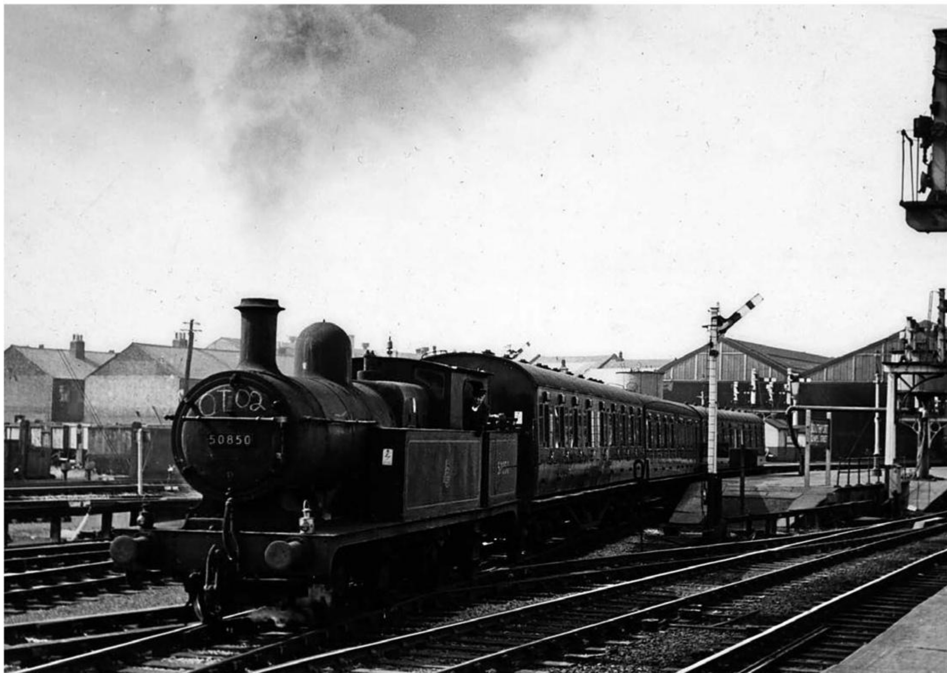
With longer tanks, extra coal capacity, Belpaire firebox and extended smokebox, Aspinall 2-4-2 radial tank No. 50850 works empty coaching stock at Chapel Street station, Southport, on August 25, 1961. The last to remain in service, it was withdrawn that October. MORTONS RAILWAY MAGAZINE ARCHIVE/IAN G. HOLT.
