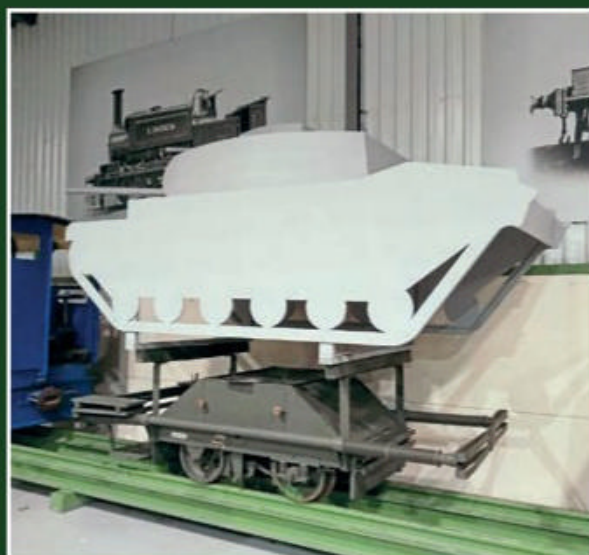
Built in the early 1940s, Trolley No. 3170 was one of a batch made for the military. It would be set off unmanned with a wooden mock-up mounted on top for target practice. It is now on display at the Statfold Barn Railway. ROY HENNEFER/RTT
