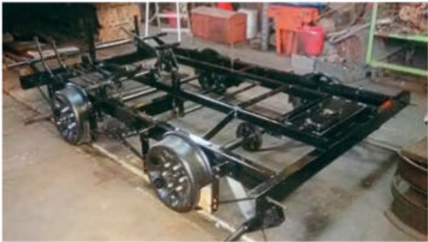
No. 6857 is perhaps the most famous Wickham around after starring in The Great St. Trinian's Train Robbery , but now it's just a rolling chassis as restoration work has paused in need of further funding. JONATHON FLOOD/RTT
