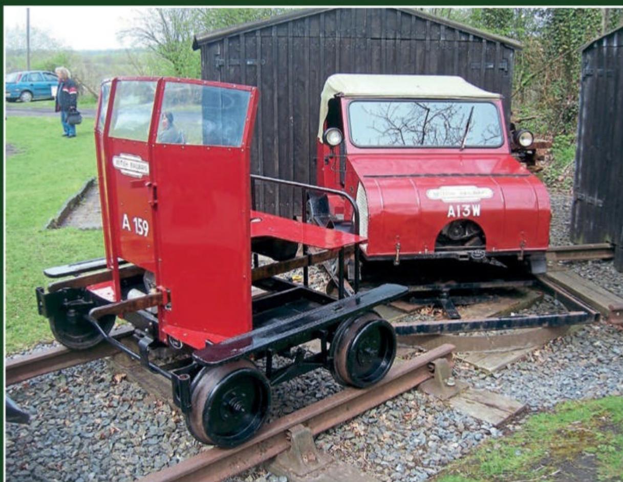
Two polar opposites when it comes to Wickham designs – the type 8S (left) is basic in appearance when compared to the type 4B (right), with its passing resemblance to a car. ROY HENNEFER/RTT
