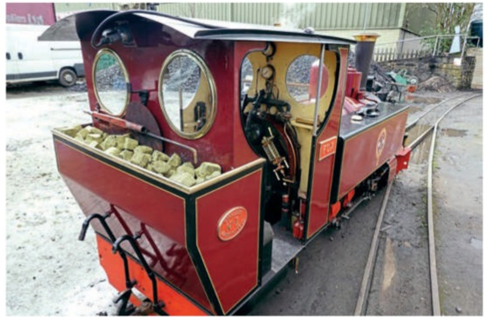
The rapeseed oil biomass briquettes being tested in Barclay 0-4-0WT No.6 Douglas on the Talyllyn Railway. STEPHEN THORPE/TR
