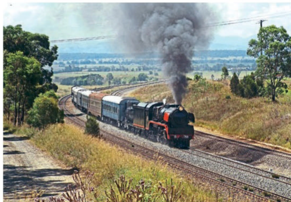
Climbing to the top: North British-built Victorian Railways' R class 4-6-4 No. 766 heads its 383-ton train on the 1-in-75 Minimbah Bank east of Singleton on Australia's Main North Line during a load trial on February 18, a month before its return to revenue-earning duty after 18 years out of service. GRAHAM BLACK
