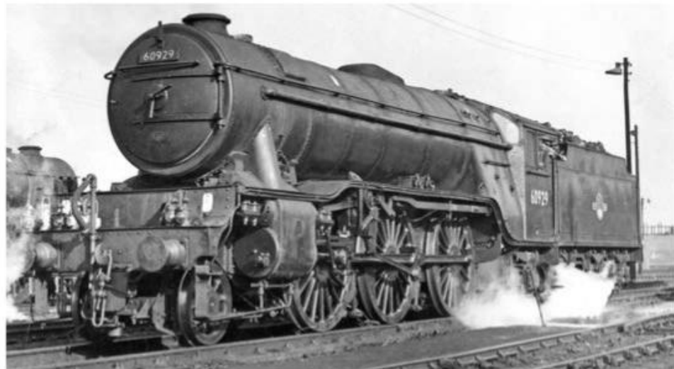
Looking smart in its late BR livery, V2 2-6-2 No. 60929 heads for the coaling plant at York MPD on March 12, 1965. The very prominent steam pipes from smokebox to outside cylinders mark the locomotive as one of the examples where cracked monobloc cylinder casting was replaced by three separate castings. MORTONS RAILWAY MAGAZINE ARCHIVE/J. D. BENSON.
