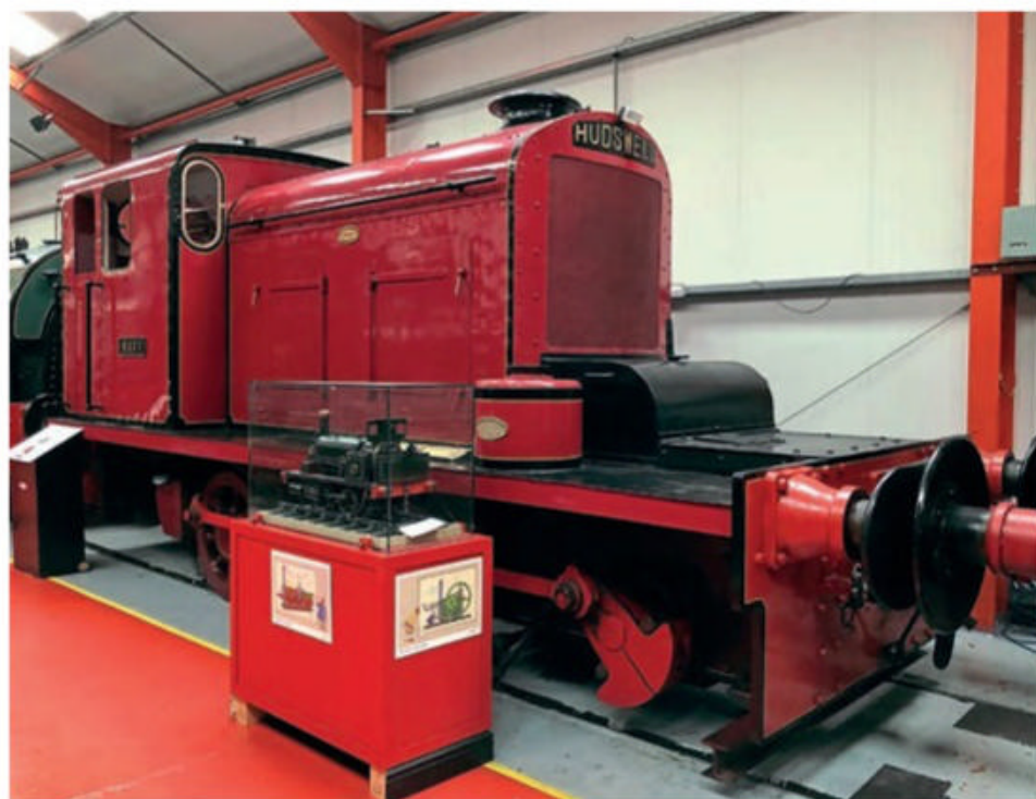
Hudswell Clarke 0-4-0DM Mary was built with a chimney and steam locomotive-style regulator because drivers were 'more used to a steam engines'.
