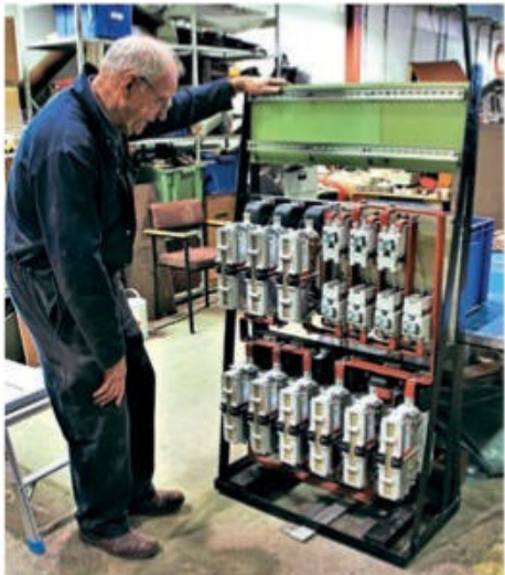
Everything under control: The team's electrical wizard, Bob Davidson, inspects the replacement contactor unit before being fitted into the tram. ALL: HUGH DOUGHERTY
