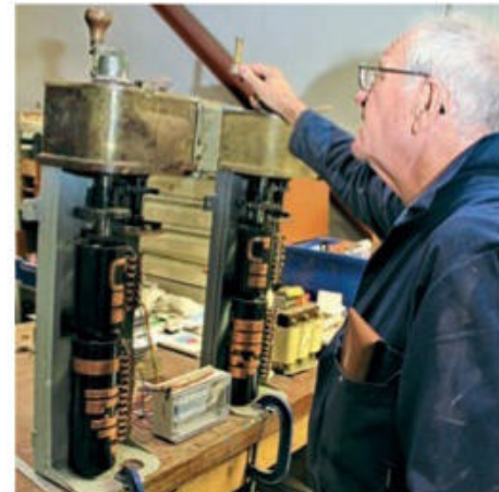
Above: The original controllers have been refurbished for use with the new contactor equipment.
