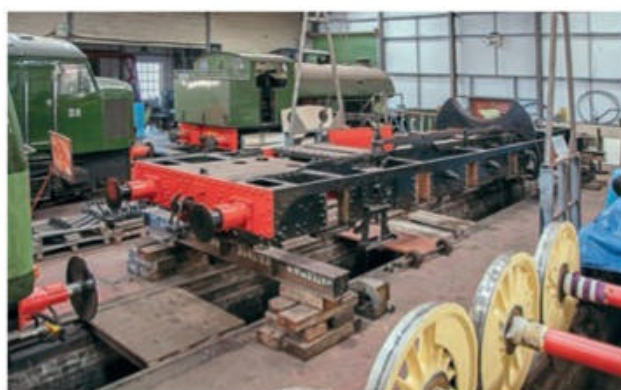
Inside the Waterman Shed at Rowsley South can be seen Class 44 D8 Penyghent , WD150 and the painted frames and re-profiled wheels of GWR 2-8-0T No. 5224.
