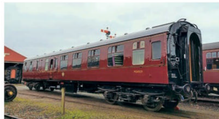
BSK No. 34929 emerges from Winchcombe carriage and wagon works after its rebuild, in which it was adapted for disabled travellers. ALEX CAULFIELD
