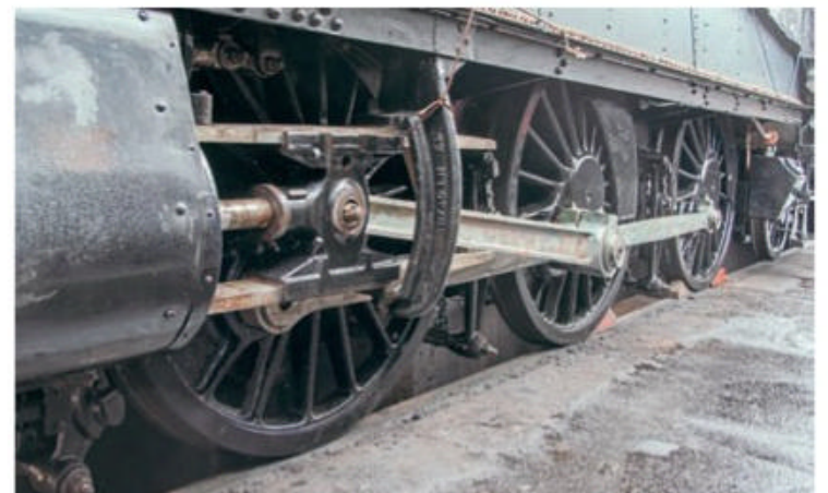
GWR large prairie No. 4150 – the last ex-Barry scrapyard locomotive on the Severn Valley Railway to be restored to steam – has now had its slide bars and rods fitted. Presently an 0-6-2T, the 1947-built locomotive is awaiting its turn on the Bridgnorth wheeldrop for the fitting of its front pony truck. If you want to help return this loco to steam, pay a visit to www.4150.org.uk JOHN TITLOW
