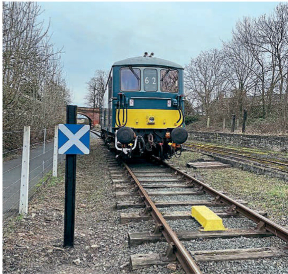
Class 73 No. E6306 (73129) with the AWS (Automatic Warning System) magnet at Oswestry station throat. The old cattle dock can be seen on the right, while a footpath is on the left. CHR
