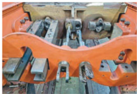
Above: The valve rod assembly trial-fitted at Statfold Engineering. STATFOLD ENGINEERING
