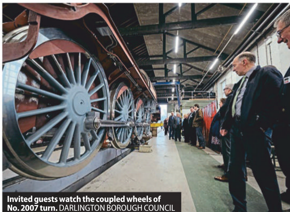
A still-boilerless No. 2007 Prince of Wales at Darlington Locomotive Works on February 25 with coupling rods in place, awaiting wheel testing on the rotator, seen to the left. GRAEME PICKERING
