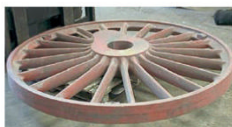
The wooden driving wheel pattern for Patriot No. 5551.
