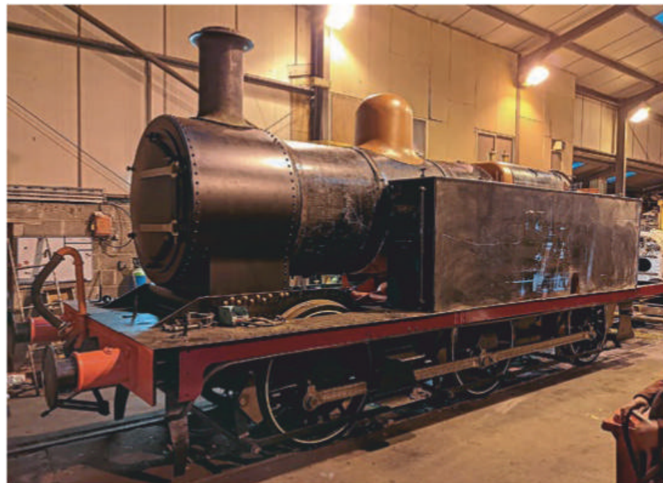
Looking more like a 'Jinty' every day: No. 16440 in the final stages of overhaul at Swanwick Junction on February 5. CRAIG BUXTON/MR-B
