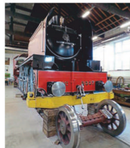
A still-boilerless No. 2007 Prince of Wales at Darlington Locomotive Works on February 25 with coupling rods in place, awaiting wheel testing on the rotator, seen to the left. GRAEME PICKERING
