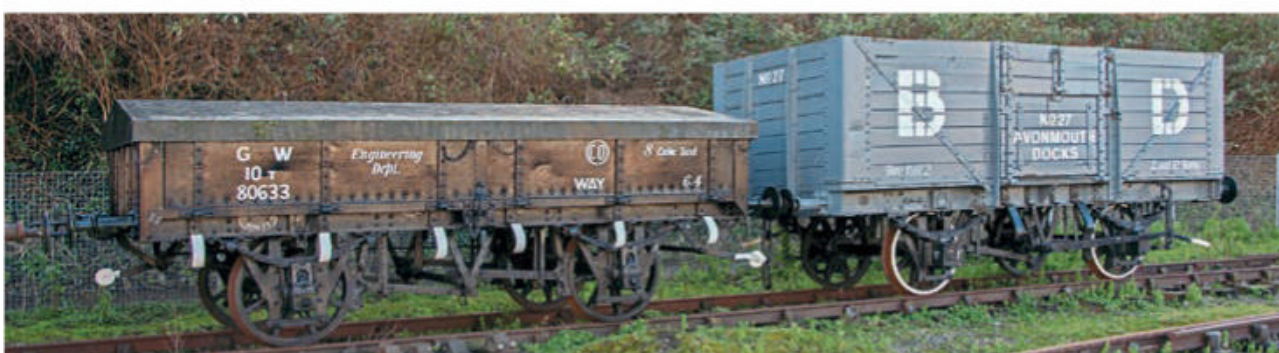
Stored alongside Wapping Wharf is GWR 10-ton engineering department Starfish ballast wagon No. 80633, built at Swindon in 1936, and LSWR and Avonmouth Docks No. BD27, a mineral wagon built in 1921.
