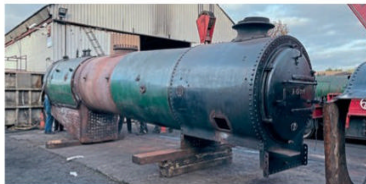
The boiler of No. 777 ready for the next stage of the overhaul after lifting. MARK ATKINS/5305
