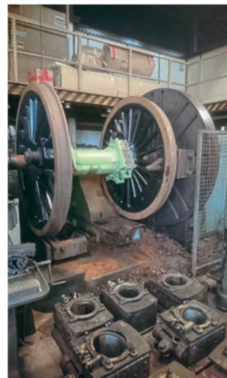
The rear coupled wheelset of No. 71000 Duke of Gloucester having its tyres profiled at Tyseley Locomotive Works. BR CLASS 8 STEAM LOCOMOTIVE TRUST
