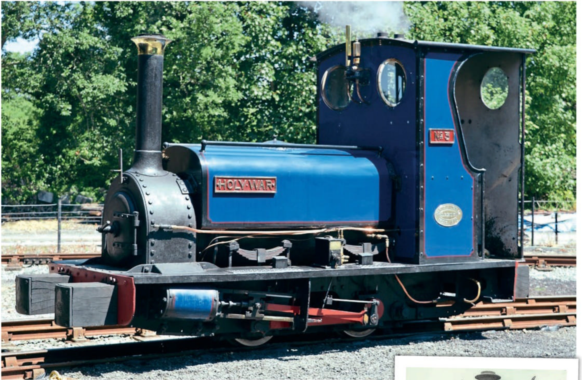
Holy War is seen here at Minffordd during the Hunslet 125 Gala. The chunkier mainframes (as pioneered on George B ) when compared with Velinheli and the current Maid Marian will be immediately apparent, as will the authentic block buffers. A cab has been fitted in preservation.
