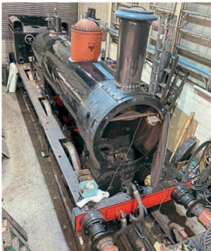
An unusual view of LNWR Coal Tank No. 1054 without the side tanks in position inside Ingrow workshop. PETE SKELLON/BLS
