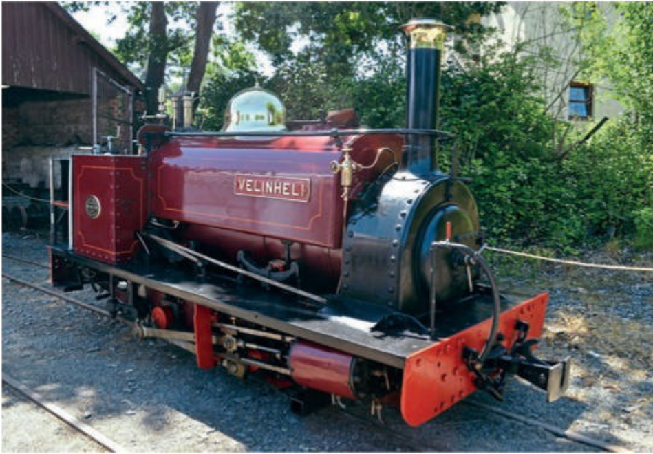
Dinorwic's Velinheli was the effective prototype of the 'Alice' class. The locomotive was extensively rebuilt in 1952, latterly running with a replacement Dinorwic Dry Dock Company-built boiler, apparently intended for the original Maid Marian , and the latter locomotive's 'square-cornered' raised waist sheets, which are higher than the back sheet and rail. Velinheli is seen here at Minfordd during the Ffestiniog & Welsh Highland Railway's Hunslet 125 gala of May 2018.
