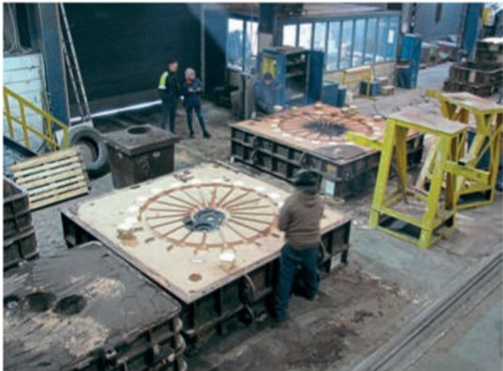
After removal of both halves of the wooden wheel pattern, complete shapes of the front face and rear face are contained in compressed sand in the left-hand moulding box (top half) and the right-hand moulding box (bottom half) respectively. B17SLT
