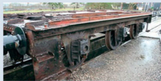
Ex-Barry scrapyard GWR 5205 2-8-0T No. 5227 at Didcot Railway Centre, destined to donate its boiler, pony wheelset and other components to new-build GWR County 4-4-0 No. 3840 County of Montgomery . PAUL HARLEY
