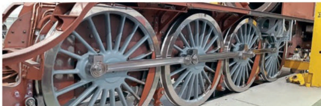
Right: The P2's right-hand connecting rods are now in place. A1SLT
