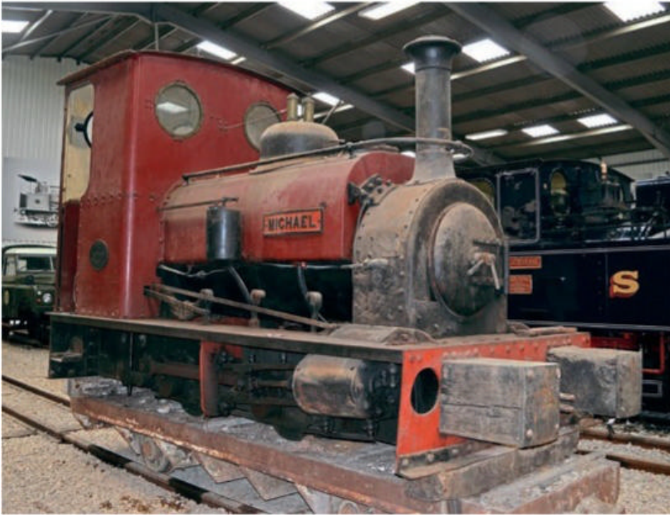
Michael at Statfold Barn on April 9, 2016, and, as with King of the Scarlets , no restoration work has taken place since repatriation. The original pattern sandboxes are still in place.
