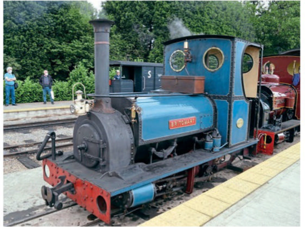
Britomart at rest near the main museum complex at Statfold Barn on July 10, 2021. Apart from its gauge and buffer design, it was the 'bridge' between the second and third generation Dinorwic 'Alice' classes. Note the neat and modest rear tank valance.
