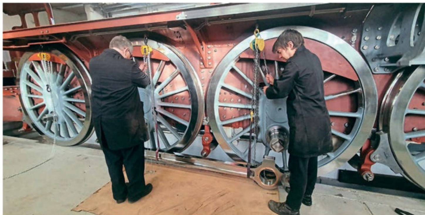
Above: David Elliott and Ed Laxton prepare to lift the first coupling rod to be fitted at Darlington Locomotive Works. A1SLT
