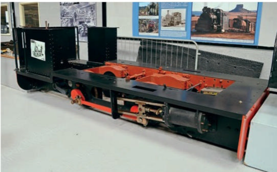
A view of current reconstruction work on Lady Madcap in the Welsh Highland Heritage Museum in May 2018, incorporating new mainframes. This view shows the 'splasher mountings' for the brake hangers, along with the firebox stretcher.
