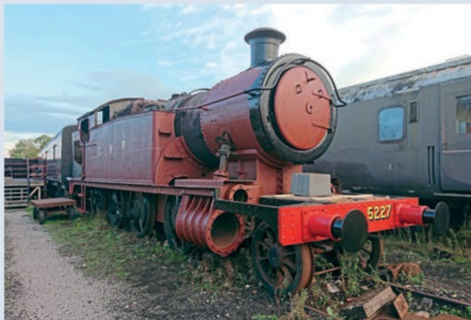
Ex-Barry scrapyard GWR 5205 2-8-0T No. 5227 at Didcot Railway Centre, destined to donate its boiler, pony wheelset and other components to new-build GWR County 4-4-0 No. 3840 County of Montgomery . PAUL HARLEY
