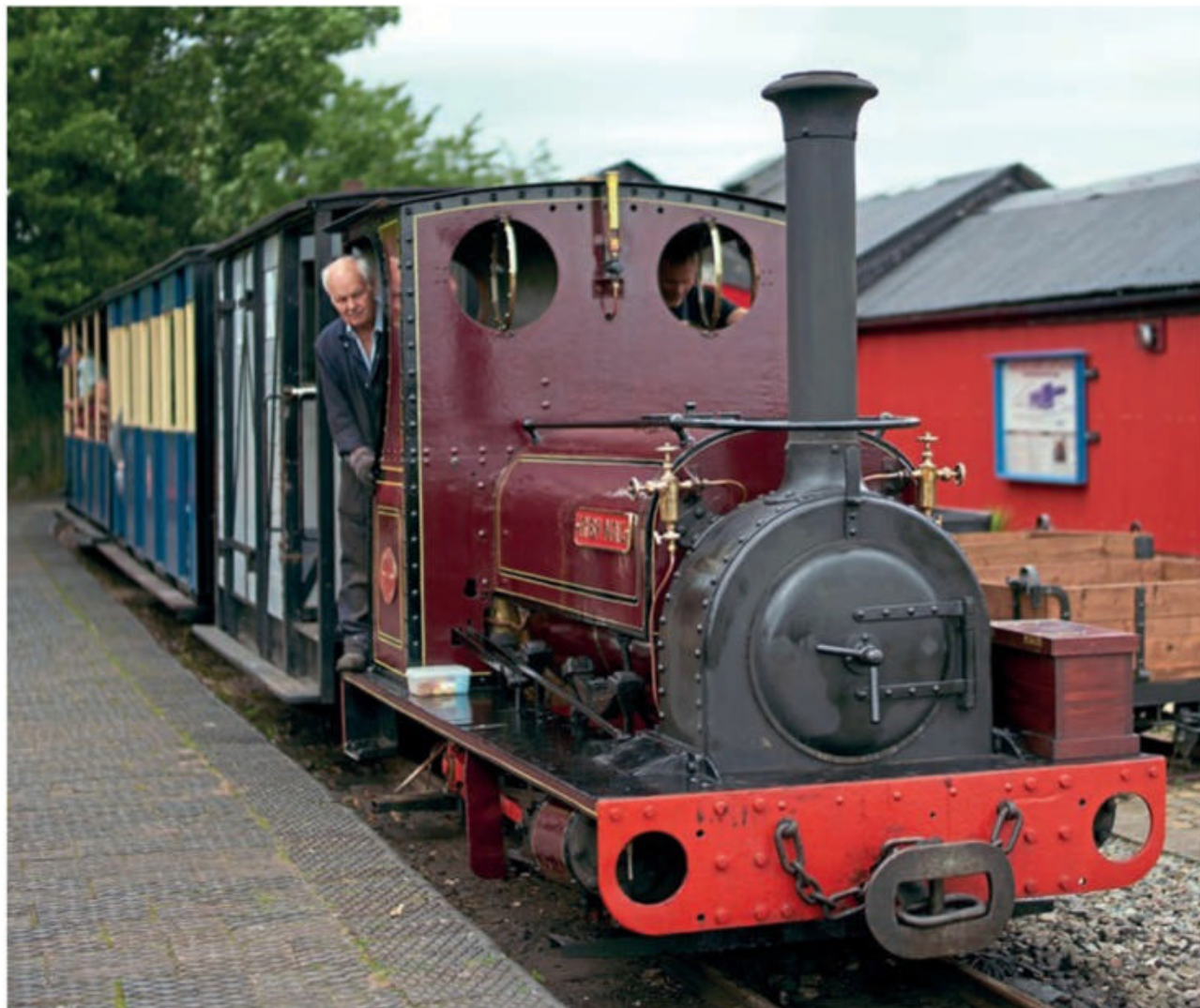
Third generation 'Alice' class Irish Mail 's upper cab has been restored in preservation on the West Lancashire Light Railway, as can be seen in this view at Hesketh Bank. Note the rear tank valence, which contrasts sharply with the pattern found on Britomart. Wild Aster/Thomas Bach carries a similar valence today in preservation, albeit with (yet another!) replacement tank. Significantly, Covertcoat , although always cabless during quarry days, latterly carried a replacement tank with a shallow Britomart-pattern rear valence. This would appear to have been originally made for Irish Mail when the latter still retained its original cab.
