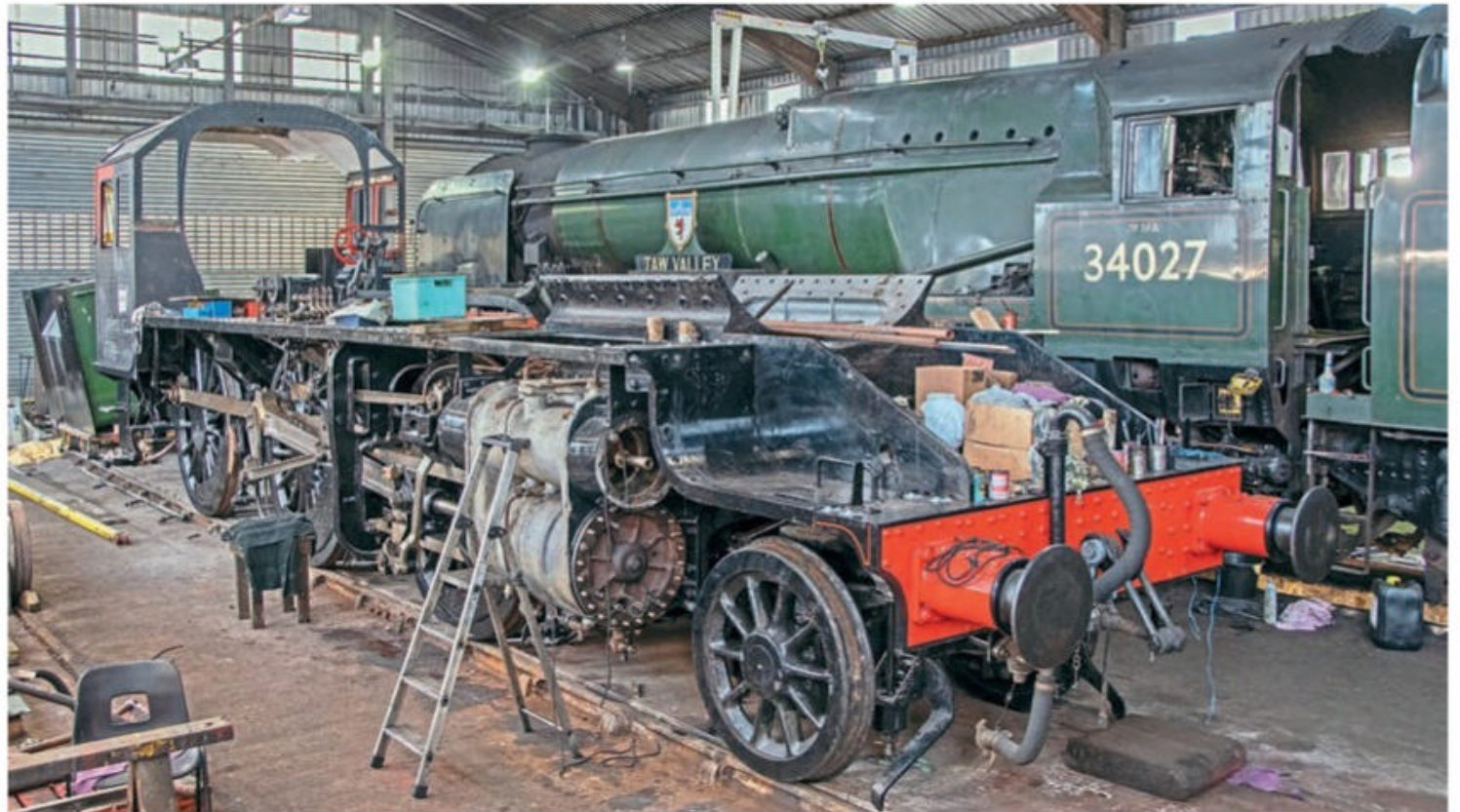
The frames of LMS 2-6-0 No 42968 and West Country 4-6-2 No. 34027 Taw Valley inside Bridgnorth shed on January 31. JOHN TITLOW
