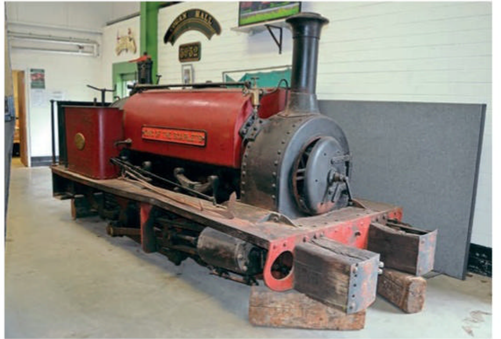
The present-day King of the Scarlets is thought to contain much of the original surviving material from Maid Marian as built, including the firebox-mounted handbrake column and high rear handrail, but today the locomotive has a standard Alice -pattern domeless boiler, short chimney, and early pattern tank and waist sheets. The third generation piston access holes (found on Irish Mail and Thomas Bach ) and footplate bolt holes for later pattern waist sheets add weight to the view that the engine's chassis is predominantly the one originally fitted to Maid Marian , as do parts of the right-hand motion stamped '822'.
