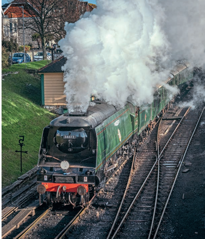
Set to visit the Great Central Railway's gala, Battle of Britain Pacific No. 34072 257 Squadron departs from Swanage with a loaded test run on December 10 following the replacement of its main internal steam pipe. DAVID ENSOR
