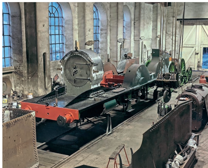
A classic from the past becoming a star of the future: LSWR 4-4-0 No. 563 under restoration in the Flour Mill workshop. NATHAN AU
