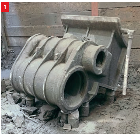
1: One of the cylinder castings cooling off at the foundry. DINMORE MANOR LOCOMOTIVE LIMITED
