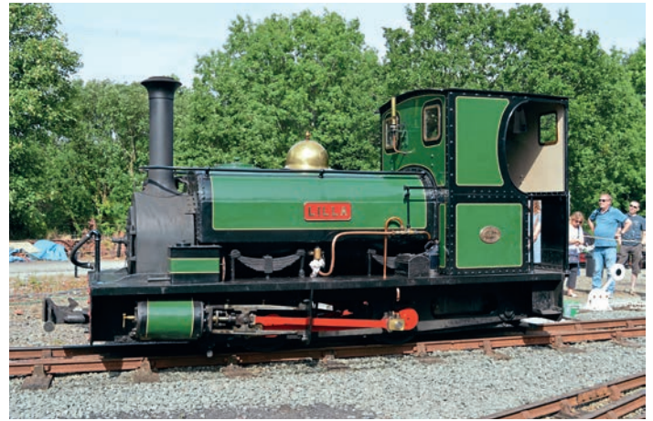
Today, Lilla is beautifully maintained in an attractive green livery on the Ffestiniog Railway, and is seen here at Minfordd during 2018's Hunslet 125 gala. The tank has a thin rear valance similar to the pattern later employed on Britomart .
