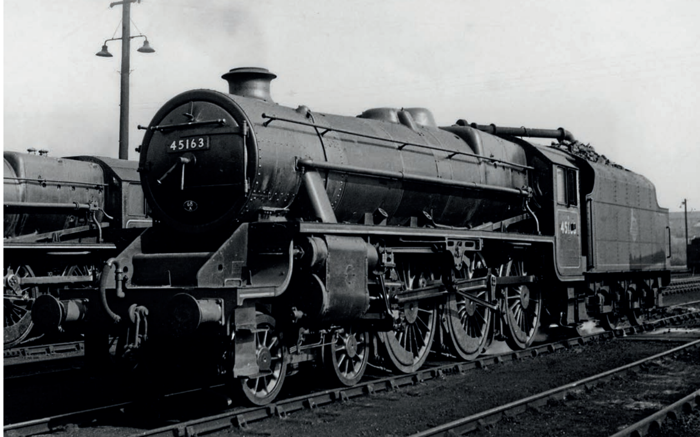
'Black Five' No. 45163 at its home shed of Carlisle Kingmoor in April 1953, showing the bracket on the cabside for the Bryson tablet catcher. JL STEVENSON
