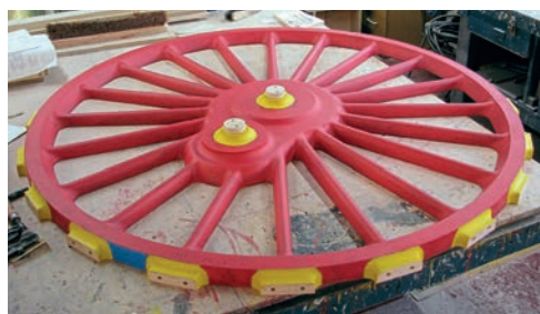
Left: The pattern borrowed from the A1 Steam Locomotive Trust to cast the 6ft 8in driving wheels for new-build B17 No. 61673 Spirit of Sandringham . B17 STEAM LOCOMOTIVE TRUST
