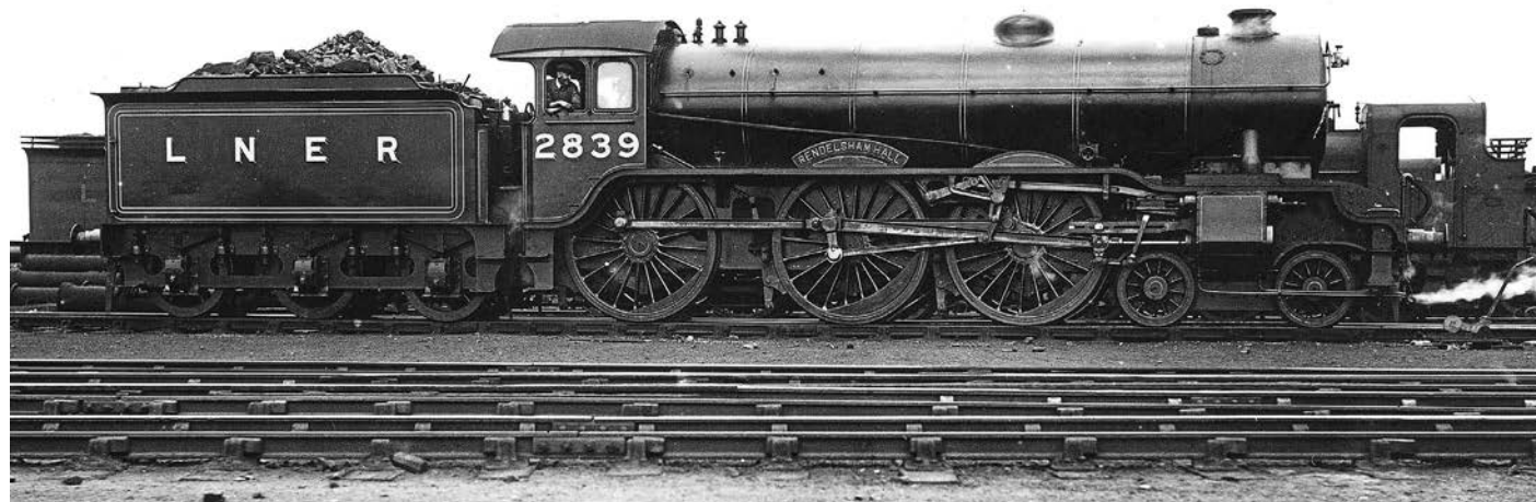
A fine view of LNER B17 4-6-0 No. 2839 Rendelsham Hall , showing its 6ft 8in driving wheels – the next components to be made for new-build example No. 61673 Spirit of Sandringham . B17 STEAM LOCOMOTIVE TRUST
