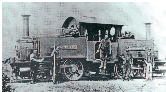
Nowadays, to unaccustomed eyes, the many standard gauge double Fairlies built throughout the world look distinctly odd. The Burry Port & Gwendraeth Valley Railway was the UK's only standard-gauge line to use such locomotives, and its 1869-built Mountaineer was pictured at Burry Port during the 1890s. MORTONS RAILWAY MAGAZINE ARCHIVE PHOTO.
