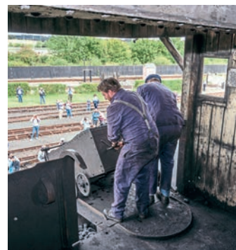
Loading coal from the tower into a locomotive below on August 31, 2020. The original half-ton capacity coal loading tubs and dumping mechanism are still in use. FRANK DUMBLETON
