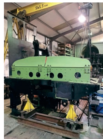
The new driver's side cab sheet in place on 'Black Five' No. 45163 at the Colne Valley Railway. 45163 LTD
