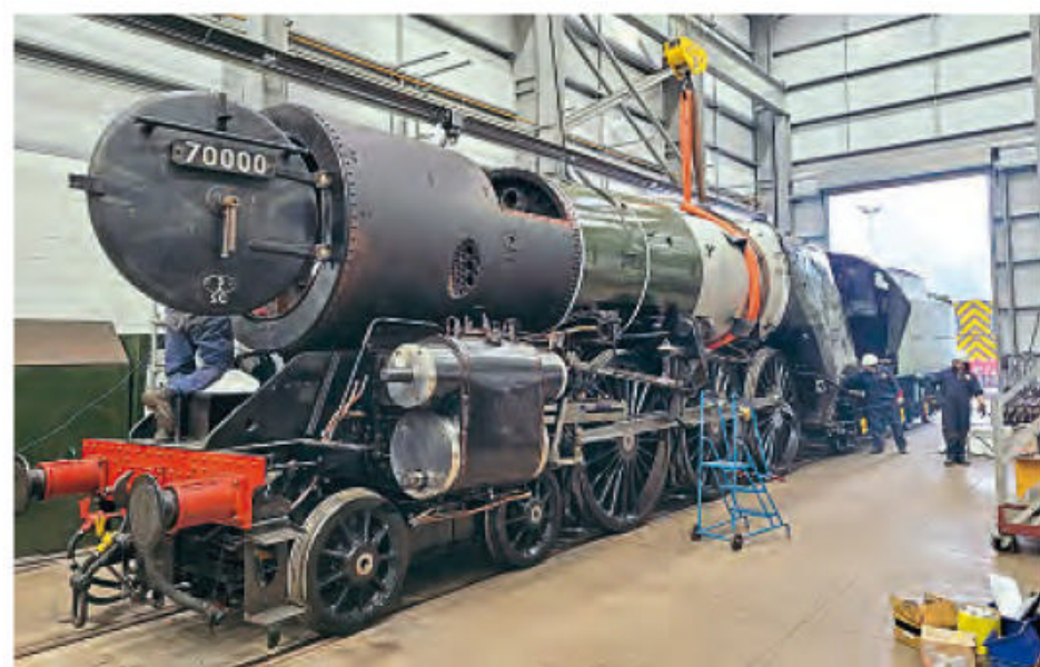
Back in the frames: The boiler of No. 70000 Britannia was lowered into place by the overhead crane at Locomotive Services Limited's Crewe workshops on November 8.
