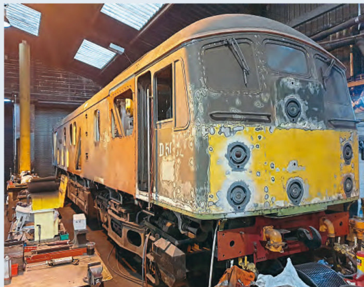
Class 24 diesel D5032 Helen Turner under overhaul in the North Yorkshire Moors Railway's Grosmont workshops. The work on its roof sections and cabs required the replacement of almost 2000 pop rivets. NICK SIMPSON/NYMR
