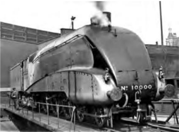
Beset with problems necessitating works attention during much of its life in its original high-pressure form, No. 10000 was rebuilt as a conventionally-boilered three-cylinder locomotive resembling a larger A4 Pacific in appearance. In this form it was pictured on the King's Cross turntable circa 1938. MORTONS RAILWAY MAGAZINE ARCHIVE/H.GORDON TIDEY
