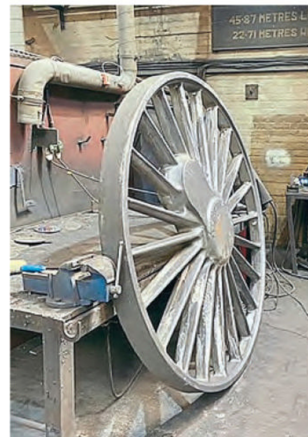
Right: The newly-cast driving wheels for No. 3840 at Trefoil Steel in Sheffield following initial cleaning. TREFOIL STEEL
