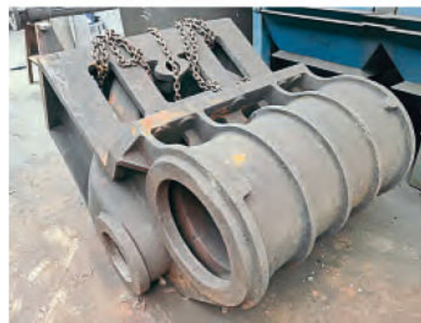
Above: The first cylinder for County 4-4-0 No. 3840 being prepared for inspection at Hargreaves Foundry. MIKE SOLLOWAY
