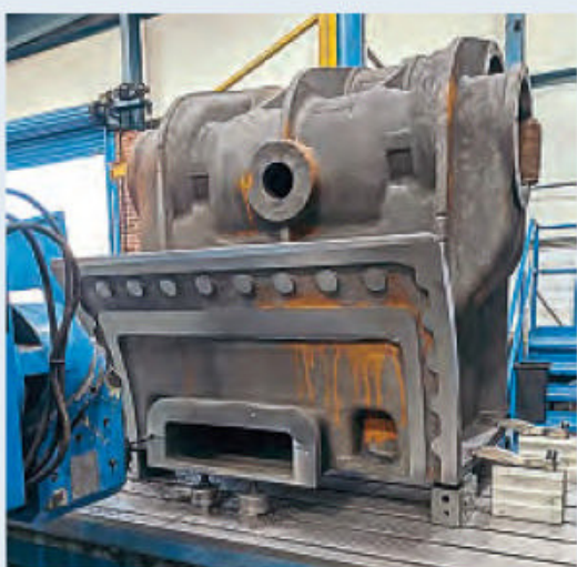
One of the cylinder castings for new-build GWR 'Night Owl' No. 4709 having its smokebox saddle machined at Roach Precision Engineering.
