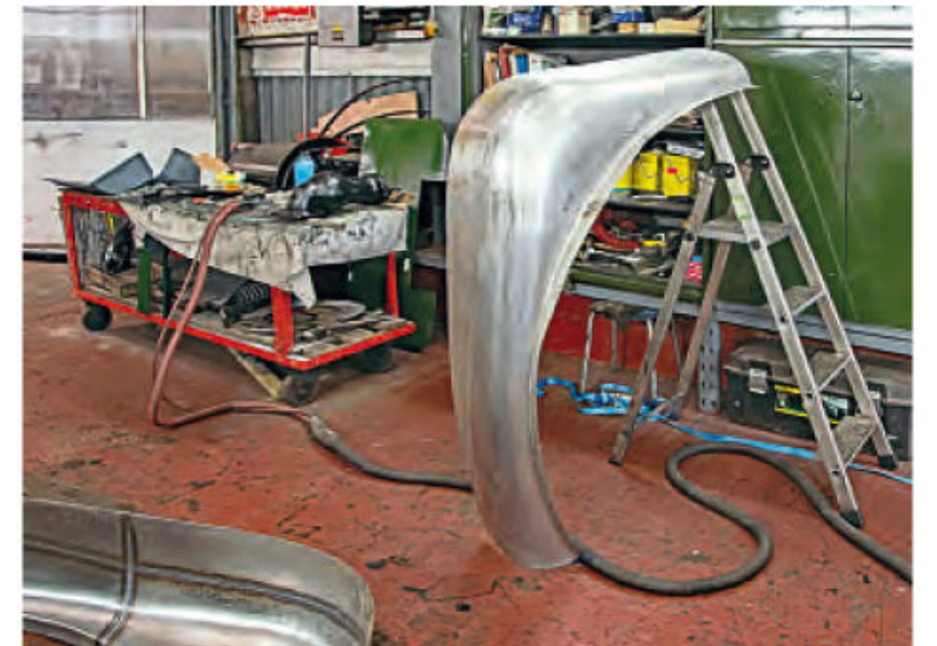
Cladding that fits around the firebox of No. 4930, which was made by a local car bodywork company, being prepared for painting inside the paint shop of Bridgnorth shed on September 15.
