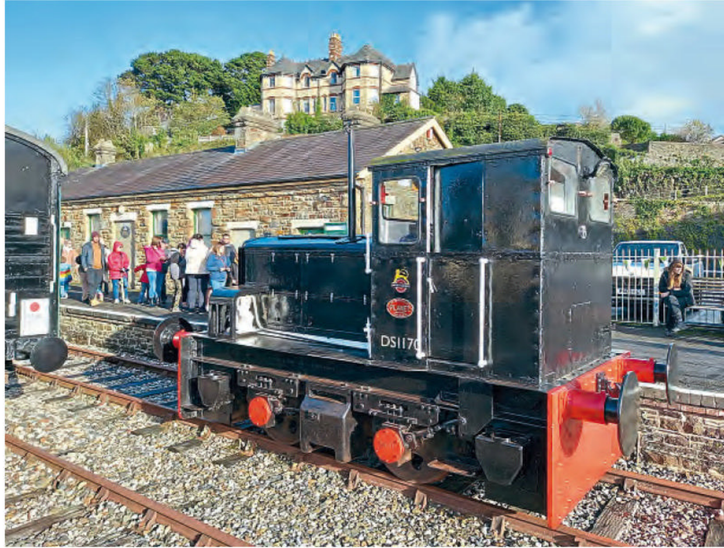
Now carrying BR black livery, Hibberd Planet chain-driven 0-4-0DM No. 3832 of 1957 Kingsley is seen running cab rides at Bideford Railway Heritage Centre on October 31. BRHC
