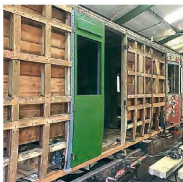
The first door refitted to London, Chatham & Dover Railway Brake Third No. 4115 at the Isle of Wight Steam Railway – only 15 more doors to go! IOWSR
