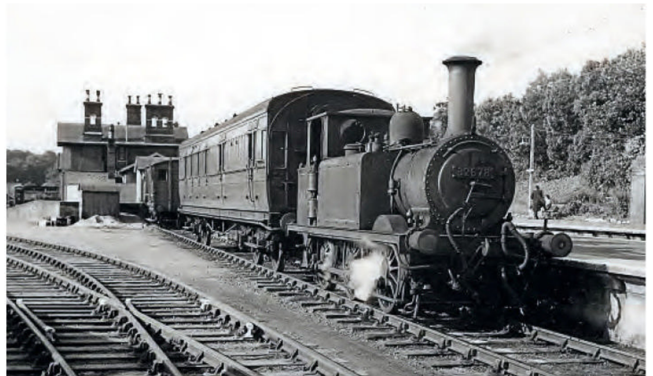
Ready for the off: Former LBSCR A1X 'Terrier' No. 32678 awaits departure from Robertsbridge with a one-coach train to Headcorn via Tenterden in about 1950. The 1880 Brighton-built 0-6-0T survived into preservation and is now a popular resident of the Kent & East Sussex Railway heritage line that runs from Tenterden to Bodiam. The Rother Valley Railway is based at Robertsbridge, where it has built a new platform and other facilities. If plans come to fruition, the current 2½-mile gap between the RVR and KESR would be bridged, leading to the probability that this 1950s steam era scene could be recreated seven decades after the original line's closure in 1954.
