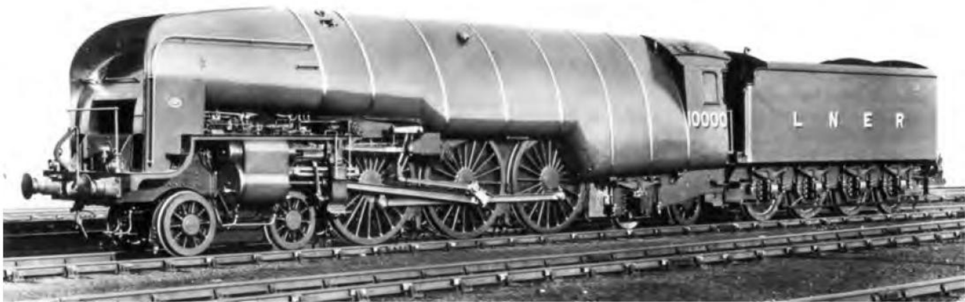
With its marine boiler dictating the shape of its boiler casing, Gresley's W1 high-pressure, four-cylinder 'Hush-Hush' compound No. 10000 must have looked like something from outer space when it posed for this LNER publicity photo in 1929. MORTONS RAILWAY MAGAZINE ARCHIVE
