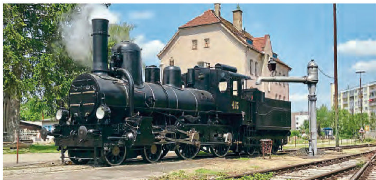
Newly restored Imperial & Royal Austrian Southern Railway 4-4-0 No. 415. BAHNPARK AUGSBURG
