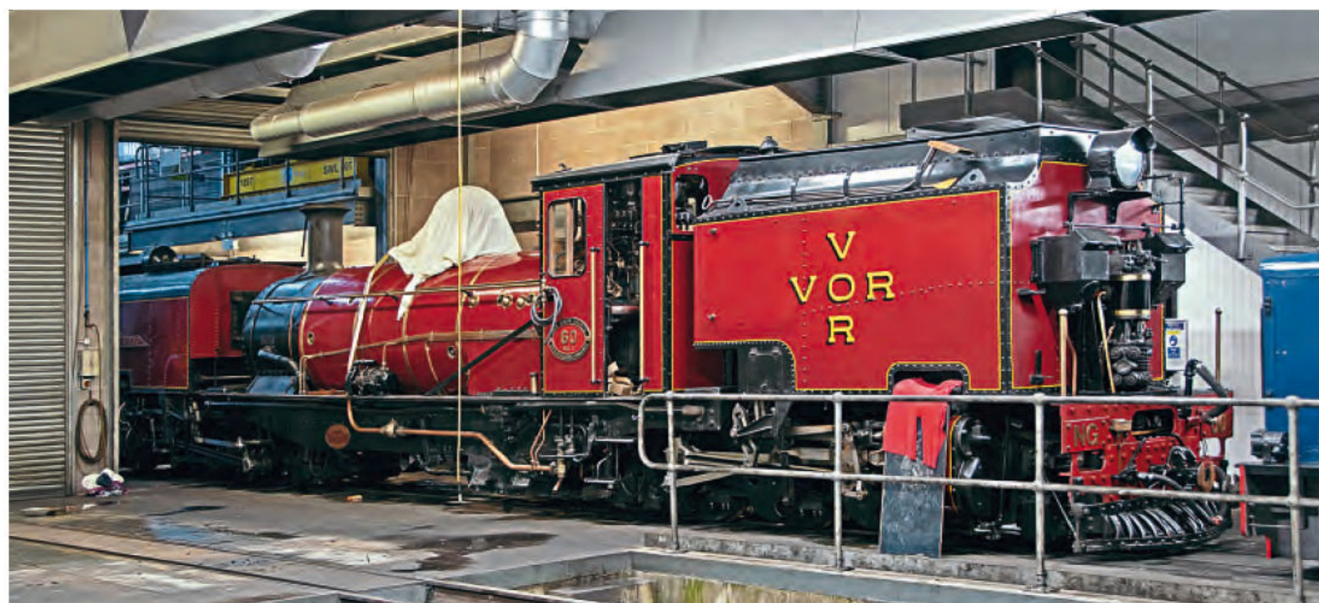
South African Railways articulated Garratt 2-6-2+2-6-2 No. 60 Drakensberg has been undergoing test runs on the Vale of Rheidol Railway, to where it was brought in 2017 from Switzerland. On October 18 it ran to Devil's Bridge on a loaded test run. The Hanomag 1927-built locomotive will enter service on the line next year. It is seen inside Aberystwyth shed on November 8. JOHN TITLOW
