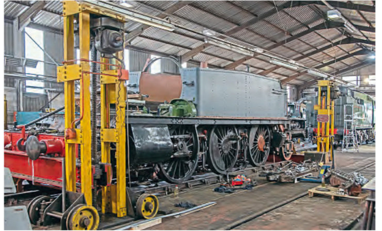
GWR 2-6-2T No. 4150, on road four inside the shed on the frame jacks with the superheater header belonging to No. 4930 prepared for testing on the right on August 13. Bulleid Pacific No. 34027 Taw Valley sits in the background.
