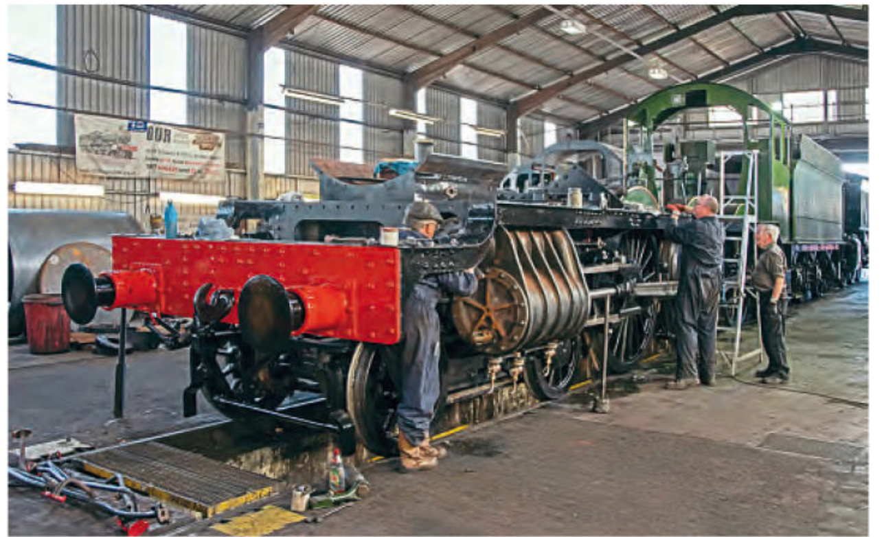
No. 4930 Hagley Hall 's drain cocks are fitted and the valves are in the process of fitting on September 8.
