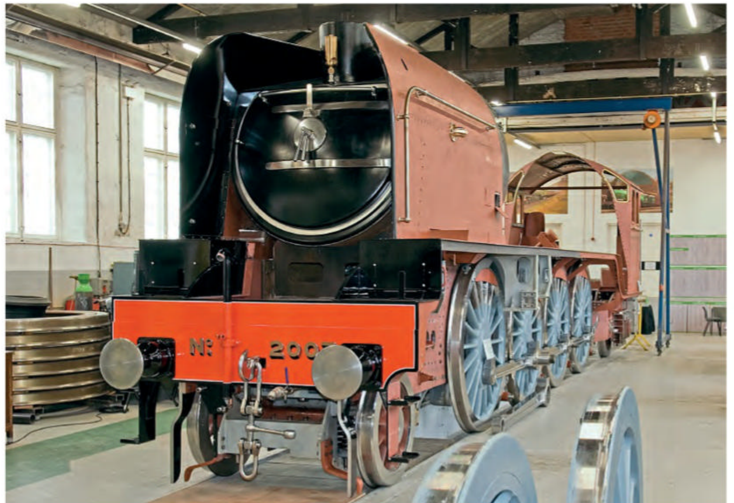
Right: Pony truck and coupling rods trial-fitted to No. 2007 Prince of Wales at Darlington Locomotive Works in time for The A1 Steam Locomotive Trust's annual convention. GRAHAM NICHOLAS/A1SLT
