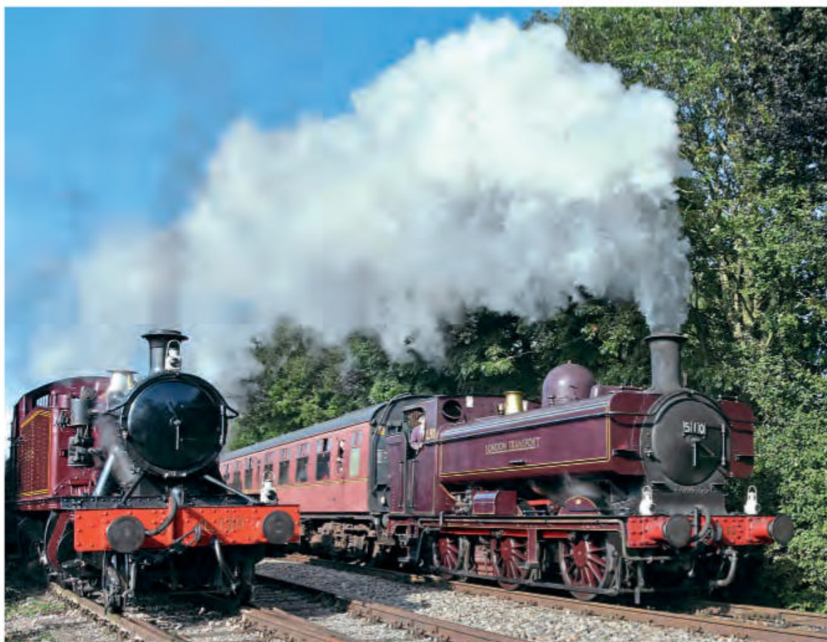
Above: GWR 4575 2-6-2T No. L150 (5521), which was specially adapted in 2013 to work on the Underground lines. KATIE PICKERSGILL/EOR
