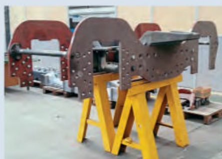
Above: The bogie frame for Clan No. 72010 Hengist trial-assembled at CTL Seal of Sheffield on October 4. BOB IFE/SSLC
