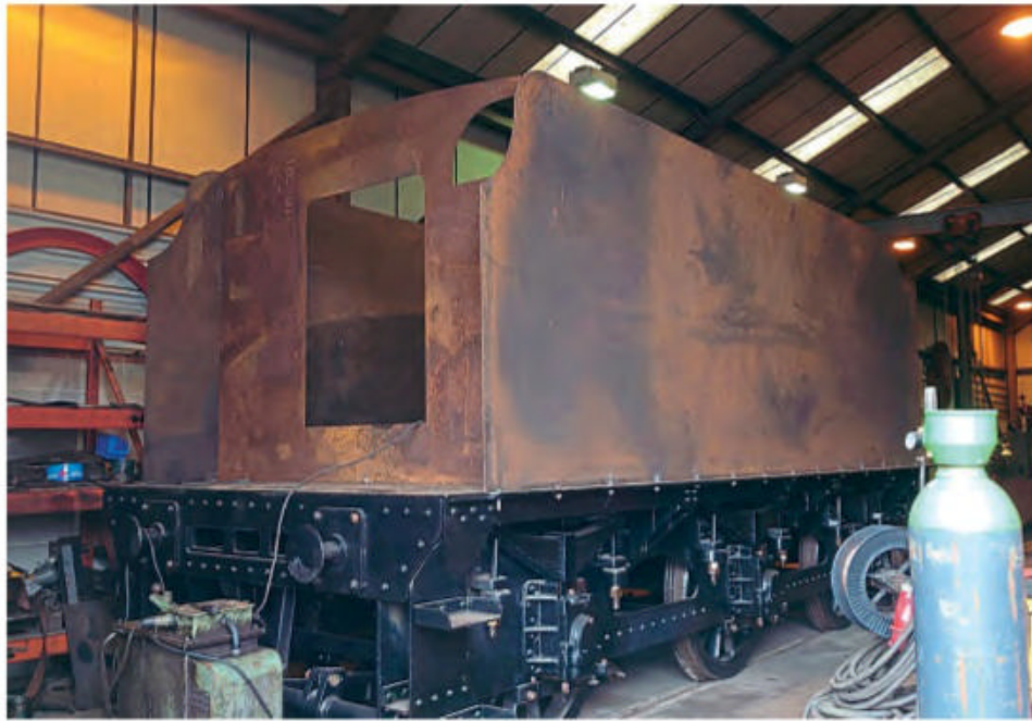
The new 8ft 6in wide Hawksworth tender tank being assembled for County No. 1014 County of Glamorgan at Didcot. 1014 GWR COUNTY PROJECT
