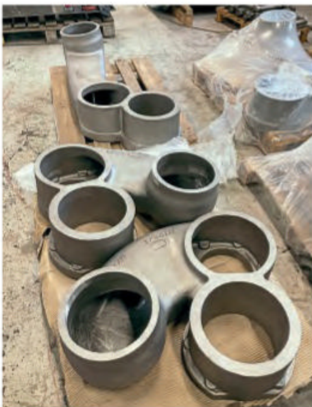
Above: Cast steam ports produced by William Cook Cast Products for the new P2 cylinder block are now at Darlington Locomotive Works. STEVE DAVIES/A1SLT
