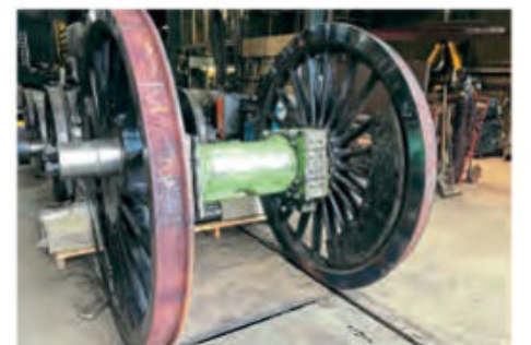
One of the driving wheelsets for Duke of Gloucester following the fitting of new tyres at South Devon Railway Engineering. BR CLASS 8 STEAM LOCOMOTIVE TRUST
