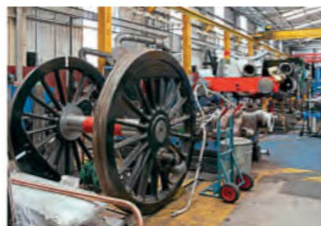
The rear driving wheels of A2 Pacific No. 60532 Blue Peter , with the multiple valve regulator, superheater casting and frames behind. JOHN TITLOW
