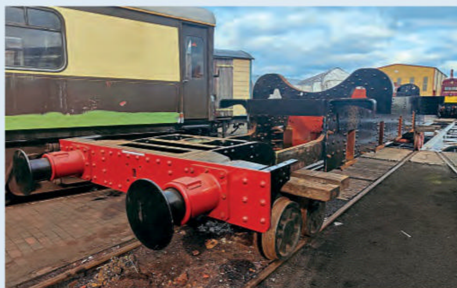
The frames of new-build GWR 47XX 2-8-0 No. 4709 on accommodation bogies following delivery to Tyseley, showing the front extension frames which will be removed for the fitting of the cylinders. PAUL PERTON
