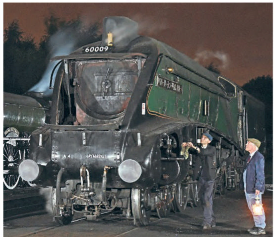
The 'cod's mouth' is wound open on Union of South Africa to access the smokebox door, while Flying Scotsman simmers in the background during the 3P20 Charters night shoot at Bury Buckley Wells on September 2. EDDIE BOBROWSKI
