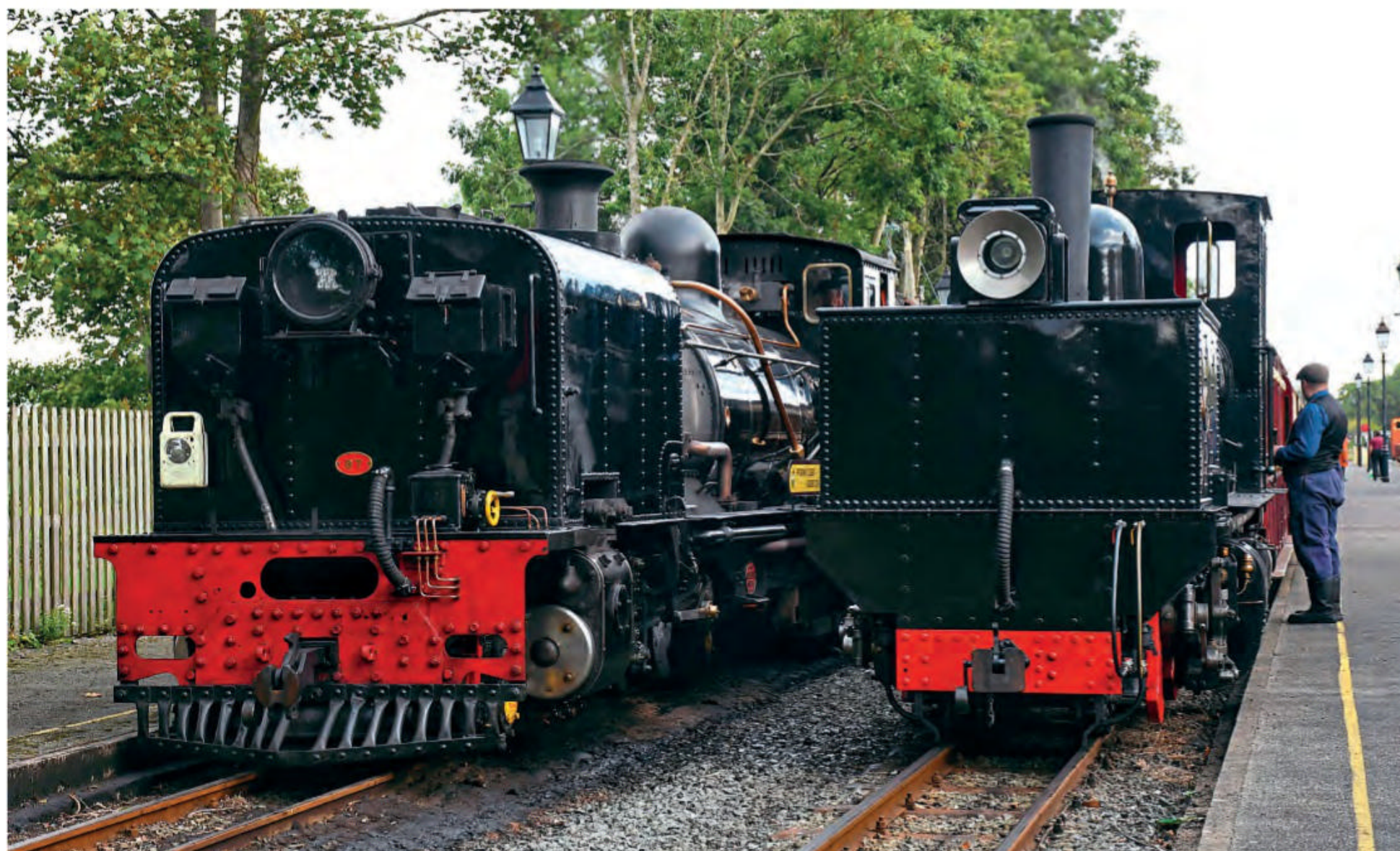
Cockerill articulated Garratt 2-6-2+2-6-2 No. 87 of 1936 and the world's first Beyer Garratt, Tasmanian Railways K1 0-4-0+0-4-0 K1, together at Dinas on the Welsh Highland Railway on September 17. On loan to restorer the Statfold Barn Railway for 10 years, K1 returned home for the Welsh Highland Railway Society's September 17-19 annual general meeting weekend, during which it worked passenger trains from Caernarfon to Rhyd Ddu for members. CHRIS PARRY/FF&WHR
