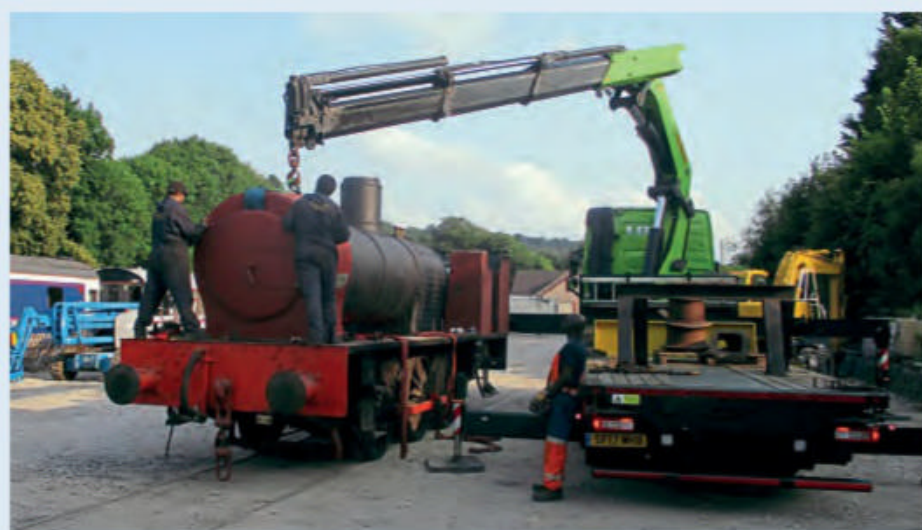
Bagnall Austerity 0-6-0ST The Duke receiving its overhauled boiler at Warkworth on July 21. BAGNALL LOCOMOTIVE GROUP
