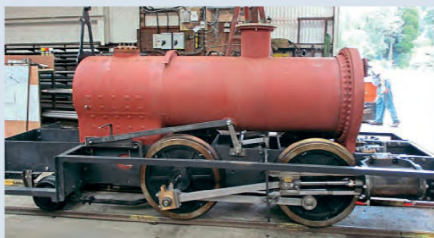
The boiler trial-fitted into the frames of new Corris Railway Hughes 0-4-2ST No. 10. ALAN KEEF LTD
