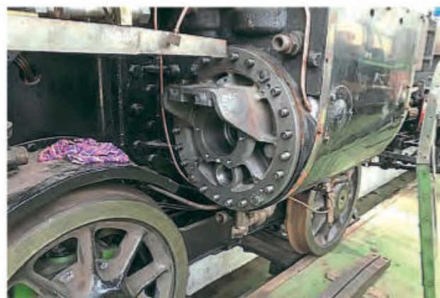
The right-hand cylinder of No. 71000 Duke of Gloucester , showing the new bracket incorporated into the rear cover casting to support the bottom slidebar (the top one is already in place).
