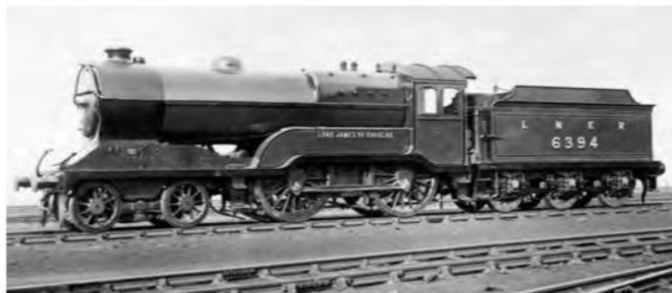
Left and above: The loading-gauge differences between the D11/1 and D11/2 sub-classes can be clearly seen in these photos of D11/1 No. 506 Butler-Henderson after restoration for preservation around 1961 and D11/2 No. 6394 Lord James of Douglas in ex-works condition in the 1930s. MORTONS RAILWAY MAGAZINE ARCHIVE/LMR PUBLICITY AND LPC LTD RESPECTIVELY.
