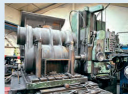
One of No. 4709's cylinders being machined at Roach Engineering. PAUL PERTON
