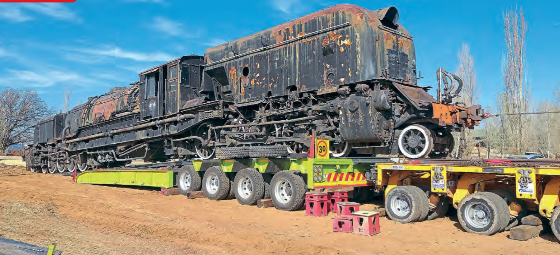
Glasgow-built articulated GMAM Garratt 4-8-2+2-8-4 No. 4114 of 1957 on its way to permanent safety at Sandstone Estates. GERT JUBILEUS
