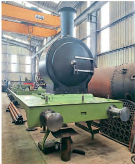
The frames of new-build GER F5 2-4-2T No. 789 at Tyseley on September 18, complete with smokebox and chimney. The front end is fully riveted and is now awaiting final polishing and painting. ELLIOT POWICK
