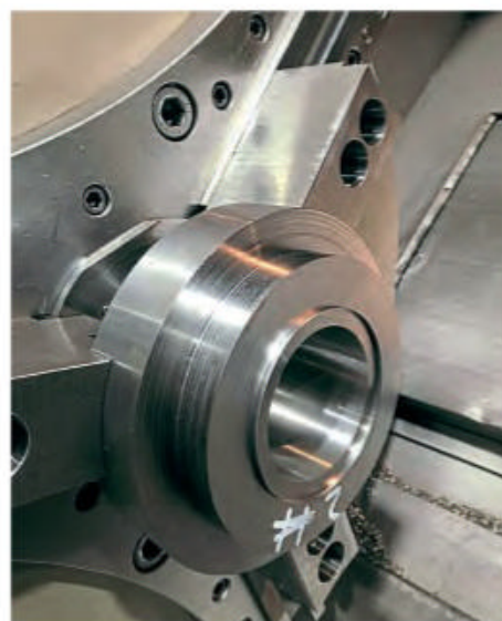
Outside cylinder inlet and exhaust valve guide housing the first stage turning on CNC lathe at Howco Group plc. HOWCO GROUP PLC/A1SLT
