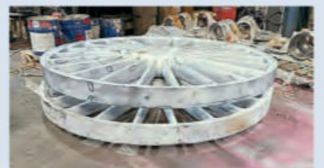
The newly-cast first two driving wheels for No. 3840 County of Montgomery . CCT
