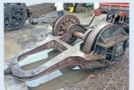
The unique fabricated trailing truck from Merchant Navy No. 35011 General Steam Navigation , which was removed from the ex-Barry Bulleid Pacific in October 2020. GENERAL STEAM NAVIGATION LOCOMOTIVE RESTORATION SOCIETY
