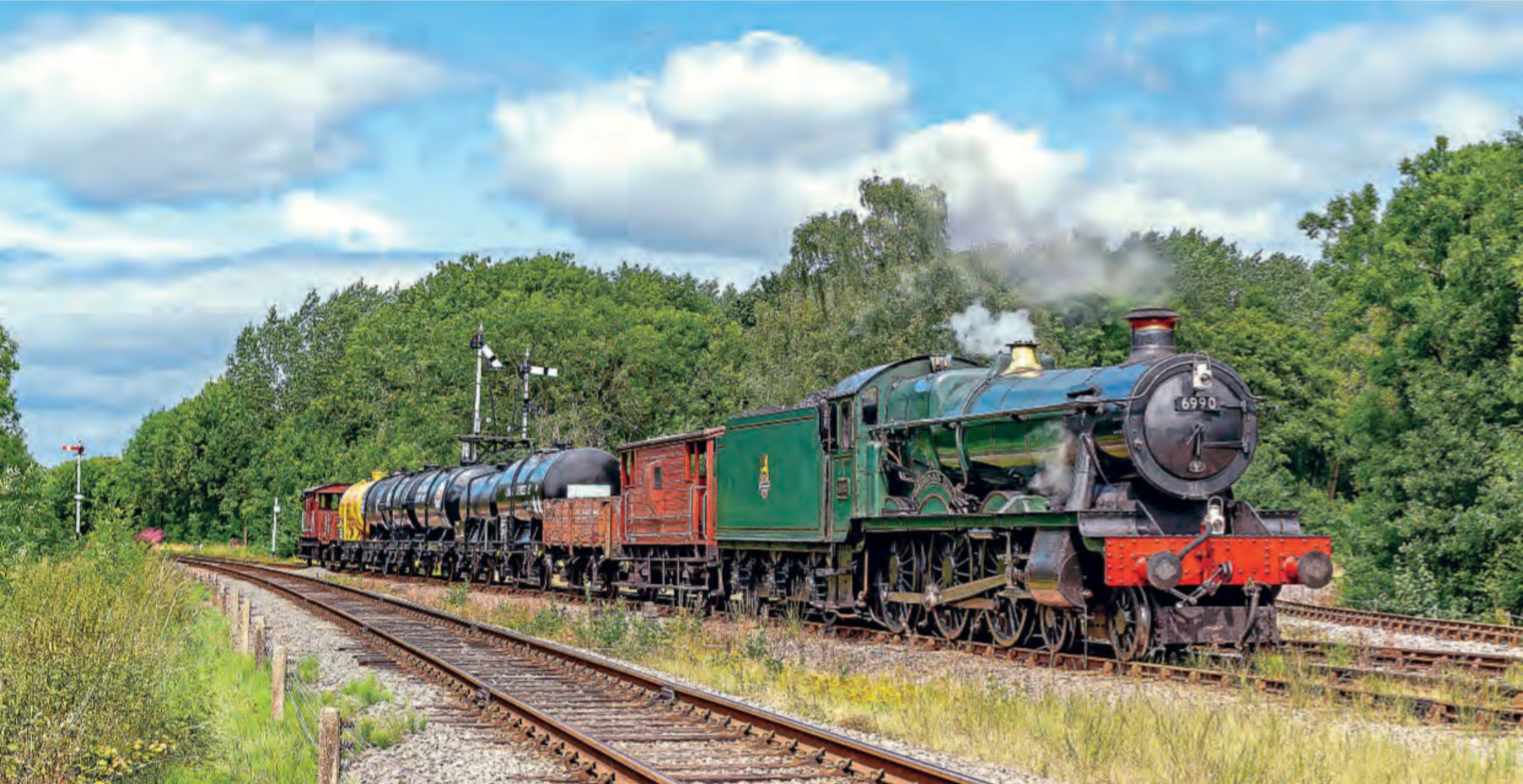
The Great Central Railway recreated a sight seldom seen in preservation during its Railways at Work gala on August 14/15 – a tanker train. Accurately marshalled with barrier wagons at the front and rear, as was the practice in steam days for tankers carrying hazardous substances, the train enters Swithland Sidings behind Hawksworth Modified Hall 4-6-0 No. 6990 Witherslack Hall on August 15. ALAN WEAVER
