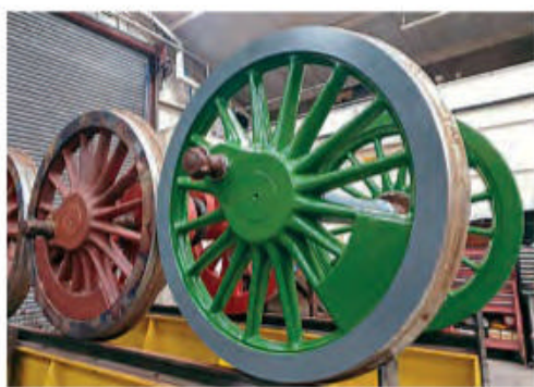
A landmark for the restoration of NER J21 No. 65033 was the first application of NER green to the refurbished driving wheels. Work is not expected to begin on the engine's rolling chassis until early next year, once the tender is completed. DAVID WRIGHT
