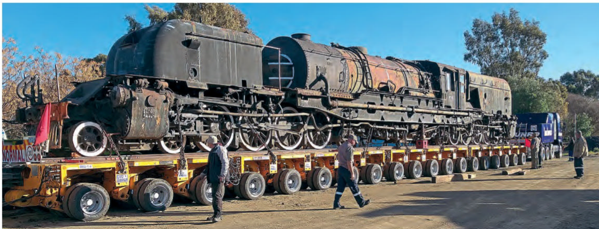
North British-built GMAM Garratt No. 4114 on the low-loader at Bloemfontein, ready for the move to Sandstone. DAVE RICHARDSON
