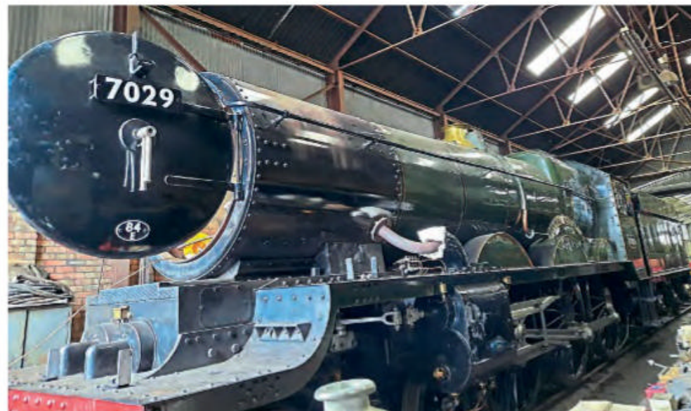
Above: GWR 4-6-0 No. 7029 Clun Castle undergoing repairs inside Tyseley Locomotive Works following the superheater header mishap on July 26. VT
