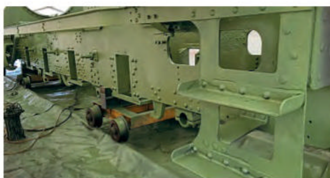
The frames of No. 2874 following cleaning and painting with anti-corrosive primer. DAVID HOLMES
