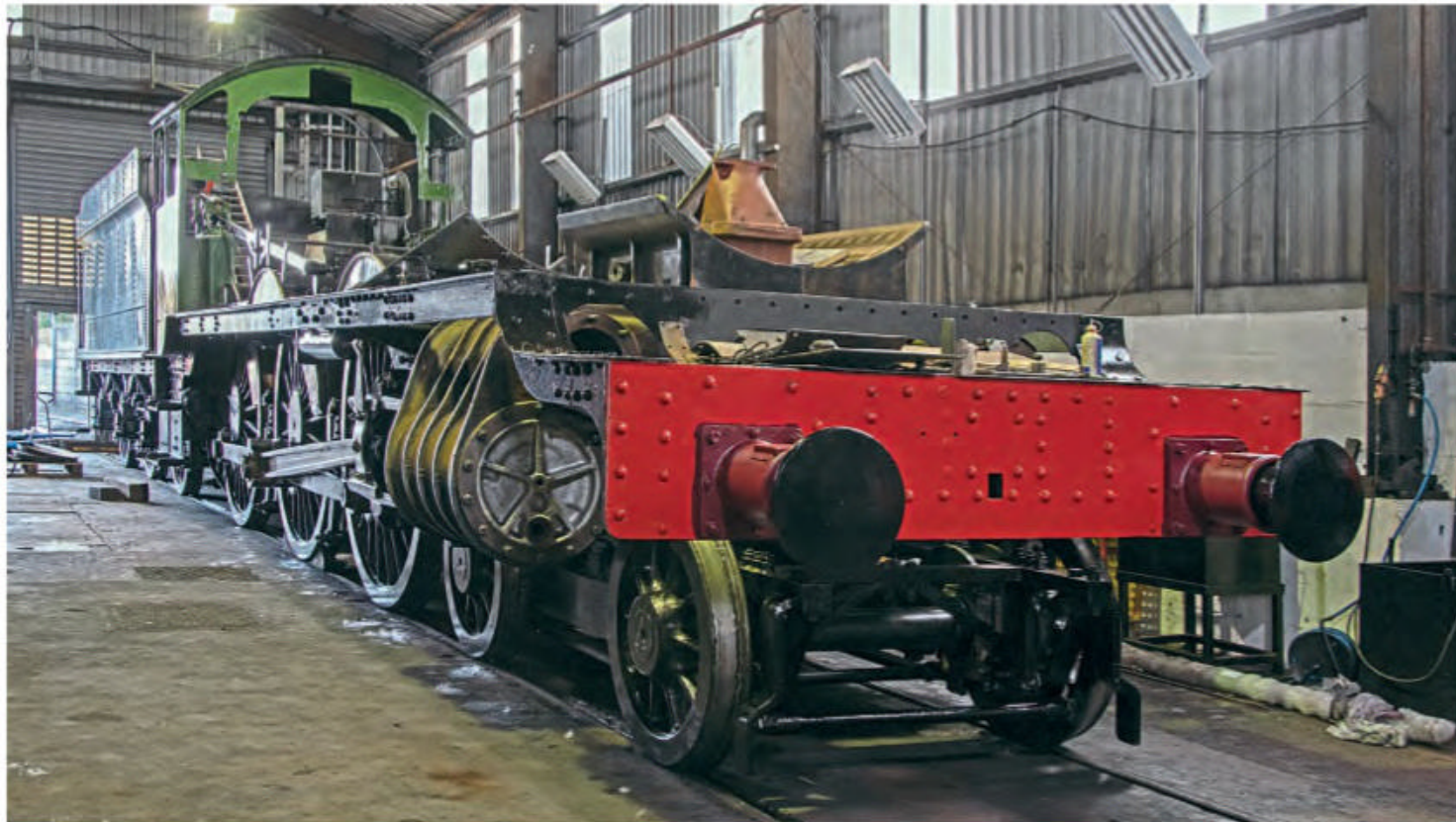
GWR Hall 4-6-0 No. 4930 Hagley Hall back on its wheels, and with its cab and rods refitted, in Bridgnorth shed on August 13. The Severn Valley Railway is appealing for funds to reroof this building – see story below. JOHN TITLOW
