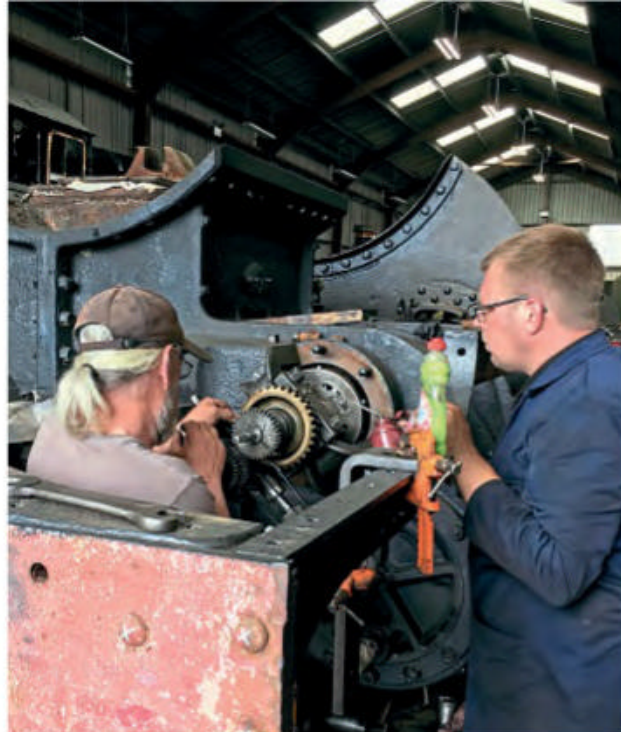
Above: Mike Solloway watching the valves being rebored by a member of the Tyseley Locomotive Works team. DAVID HOLMES
