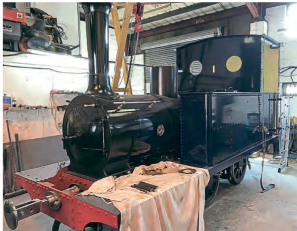
The new Blyth inside the North Bay Railway Engineering Services workshop in Darlington, ready for its final coat of blue paint. NBRES
