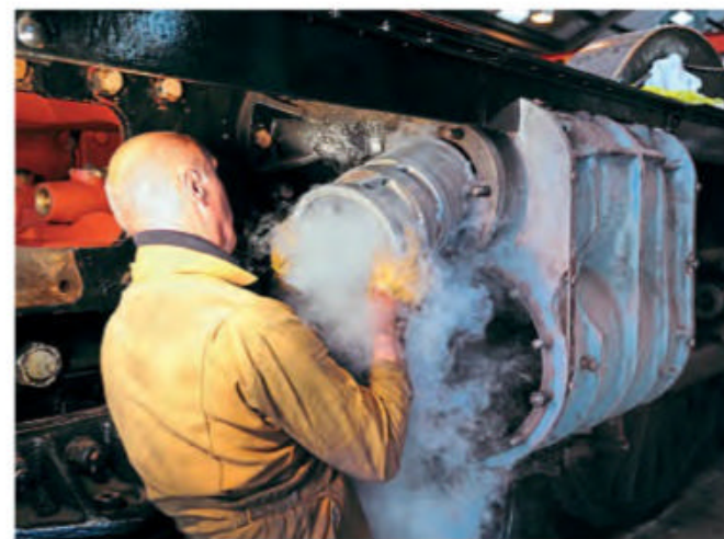
Above: One of the biggest engineering tasks on Pendennis Castle 's restoration, apart from the boiler, was relining the valves and cylinders, work which was contracted to Bryn Engineering of Wigan. In December 2010, John Marrow and Duncan Ward, of Bryn Engineering, were at Didcot Railway Centre to clean and measure the valve and cylinder castings on the locomotive, before machining to size the liners, which had already been cast, and later returning to shrink fit them. Duncan is seen here pushing the front valve liner into the left-hand outside cylinder of No. 4079, after it had been shrunk in liquid nitrogen. FRANK DUMBLETON
