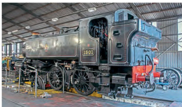
Hawksworth 15XX 0-6-0PT No. 1501 having its front driving wheels removed using the wheeldrop in Bridgnorth shed on July 21, for inspection of the bearings and replacement of the oil pads. JOHN TITLOW
