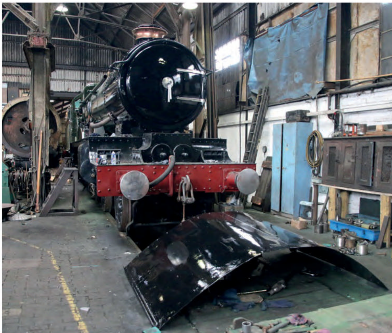
Above: One of the biggest engineering tasks on Pendennis Castle 's restoration, apart from the boiler, was relining the valves and cylinders, work which was contracted to Bryn Engineering of Wigan. In December 2010, John Marrow and Duncan Ward, of Bryn Engineering, were at Didcot Railway Centre to clean and measure the valve and cylinder castings on the locomotive, before machining to size the liners, which had already been cast, and later returning to shrink fit them. Duncan is seen here pushing the front valve liner into the left-hand outside cylinder of No. 4079, after it had been shrunk in liquid nitrogen. FRANK DUMBLETON
