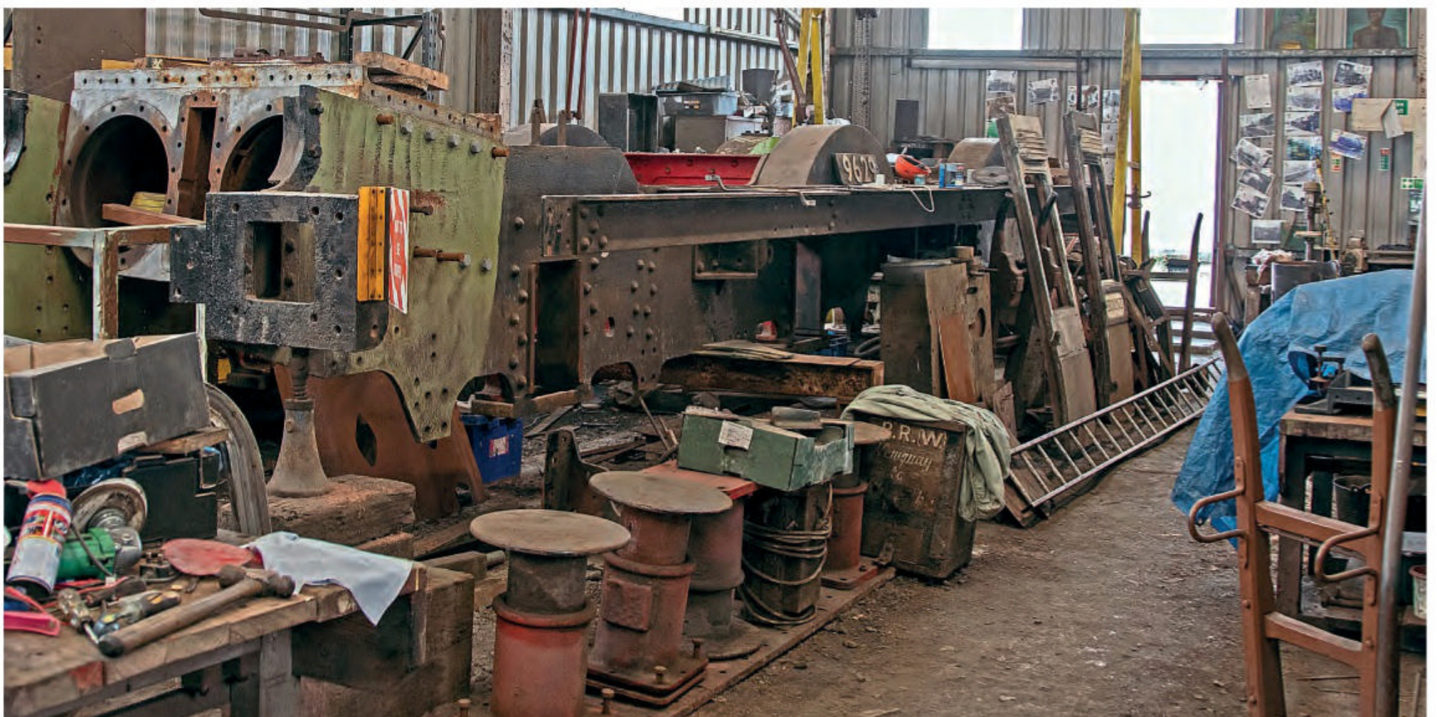
Below: The stripped-down frames of ex-Barry pannier tank No. 9629 under restoration. JOHN TITLOW
