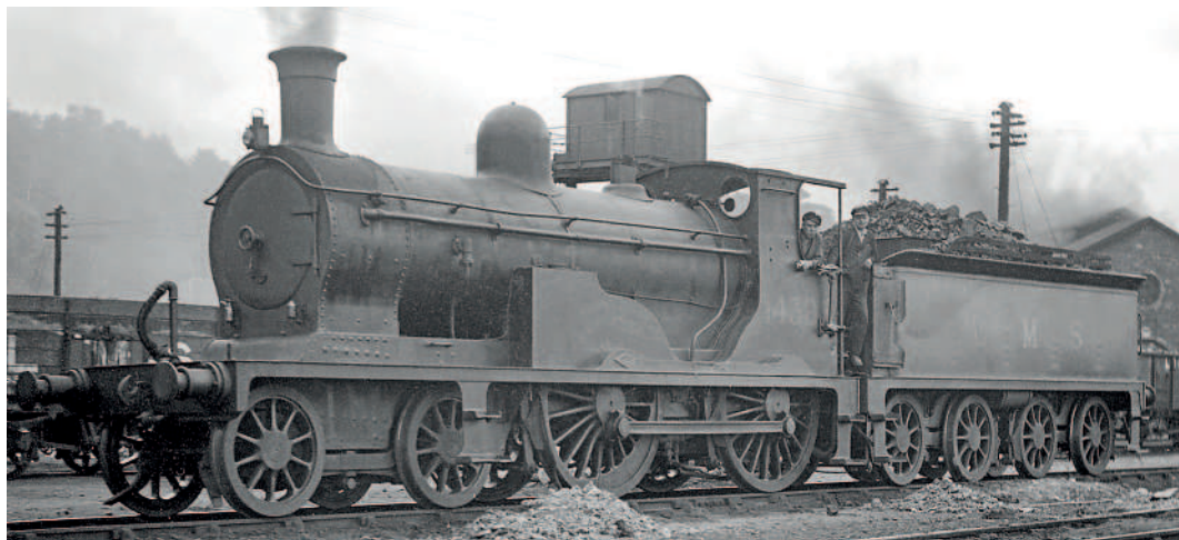
In LMS days, Ben Alder stands on Inverness shed showing its inside-axlebox Drummond tender. MIKE MORANT
