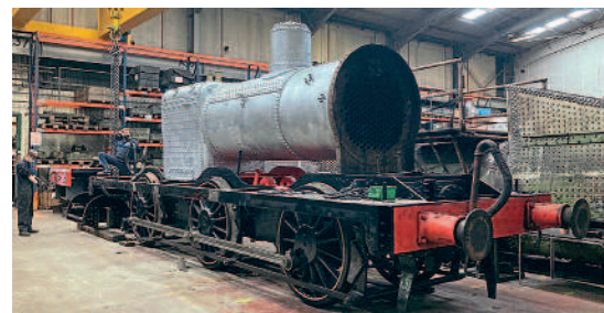
Once the boiler arrived at Riley & Sons workshop, it was quickly fitted to the rolling chassis. MR-B
