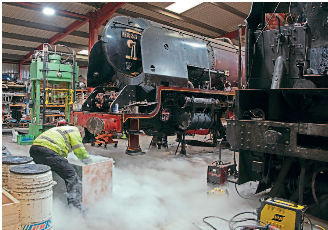
Above: Fitting the replacement outside cylinder liners to No. 6233 Duchess of Sutherland inside the West Shed on July 6. JOHN TITLOW
