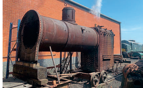
The boiler of No. 16440 lifts its safety valves during a boiler test at the North Norfolk Railway before transportation to Riley & Sons (E) workshop for fitting to the restored frames. MR-B
