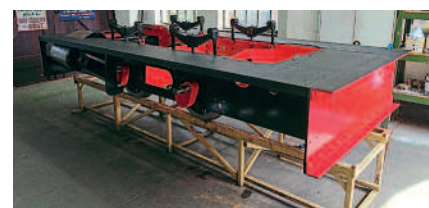
The frames and wheelsets of the latest new-build Quarry Hunslet Juliette in the Statfold Engineering Ltd workshops. SBR
