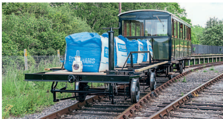
Ryde Pier tramcar No. 2 at Smallbrook Junction during its test runs with the chassis of its replica trailer No. 10, ballasted to simulate its weight once the bodywork is added. JOHN FAULKNER
