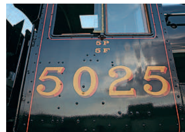
A close-up of the fireman's side of the cab showing the extra lining around the sides and bottom of the windows that was applied only to the first 50 Vulcan Foundry-built examples, Nos. 5020-5069. JAYNE-LOUISE EMSLEY
