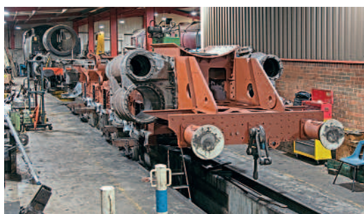
The stripped-down frames of 9F No. 92212 under overhaul in the West Shed. In the background are BR Standard 2-6-4T No. 80098 and LMS 4-6-2 No. 46233 Duchess of Sutherland . JOHN TITLOW
