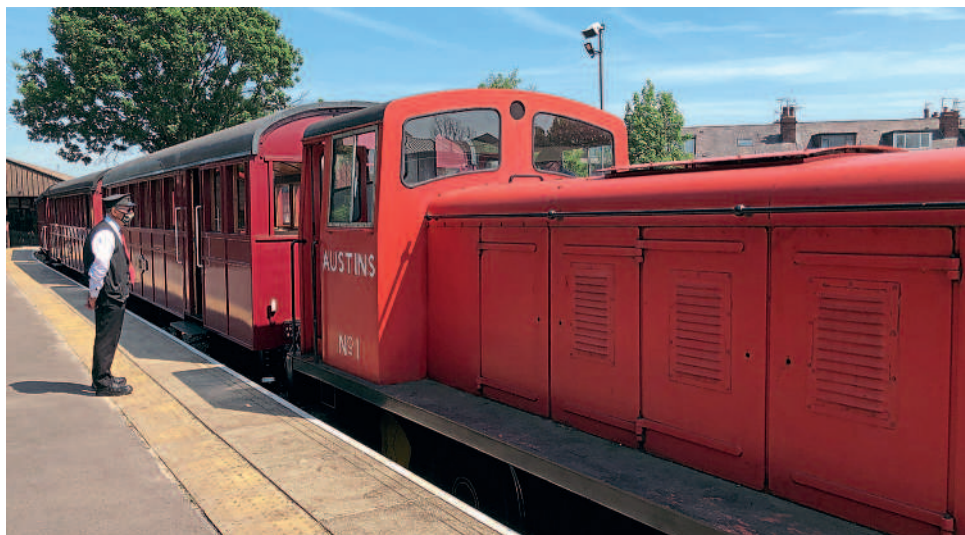
Mind the gap: Peckett 0-4-ODM No. 5003 of 1961 Austins No. 1 awaits its passengers. One of only five diesel shunters built by Peckett, it started out as a demonstration locomotive and in 1961 was sold to Dewsbury stockholders James Austin & Sons, hence its name.
