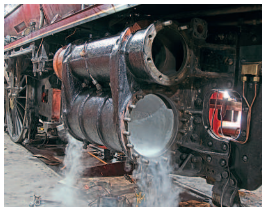
Above: Fitting the replacement outside cylinder liners to No. 6233 Duchess of Sutherland inside the West Shed on July 6. JOHN TITLOW
