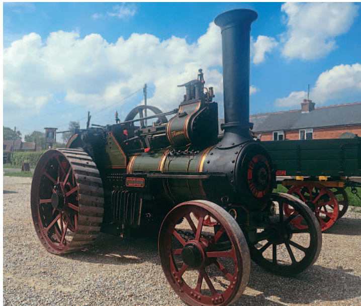
This 1901 Burrell single-crank compound, double drive, general purpose traction engine, Works No. 2386 Titaness , is being used for trials of biocoal. It belongs to Bill Giles, one of the organisers of the Weald of Kent Steam Rally, which will be held on August 7/8. BILL GILES
