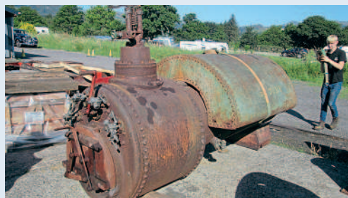
The boiler, smokebox and saddle tank of Dorothy back in the country where it was built to serve. TIM WILLIAMS
