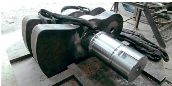
The crank axle for No. 71000 ready to place its cannon boxes. BC8SLT
