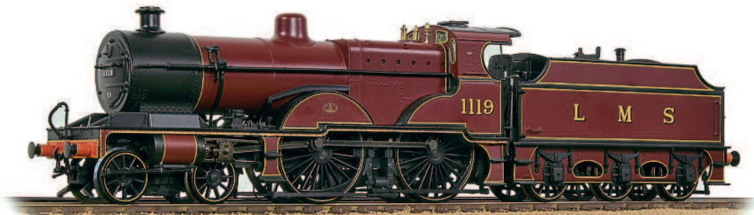
The elegant lines of the 195 three-cylinder Compound 4-4-0s built by the LMS between 1924 and 1932 are captured to perfection in this left-hand-side view of Bachmann's new OO-scale model of No. 1119 (31-934).
