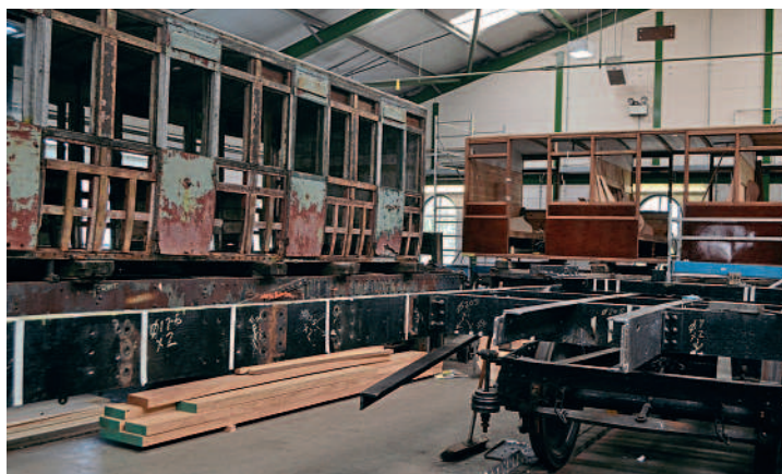
The body of London, Chatham & Dover Railway Brake Third No. 4115 (left) in the works at Havenstreet. In the foreground is the Southern Railway 'elephant van' underframe to which it will be fitted, showing where it will be shortened by 5ft in the centre. In the background, restoration work on Isle of Wight Railway Oldbury First No. 21 is making steady progress, with the new lower panels in place.
