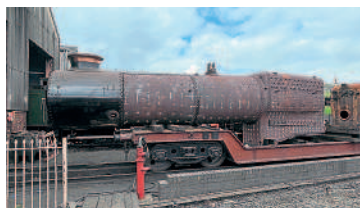
The boiler of GWR Castle 4-6-0 No. 5043 Earl of Mount Edgcumbe awaiting its hydraulic test at Tyseley. DENIS CHICK/VT
