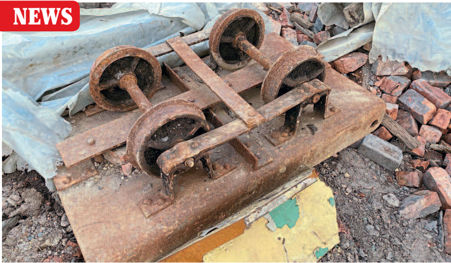
Rediscovered: The two foundry wagons which ran on the 18in gauge internal system at Horwich Works. ANDREW WALDRON
