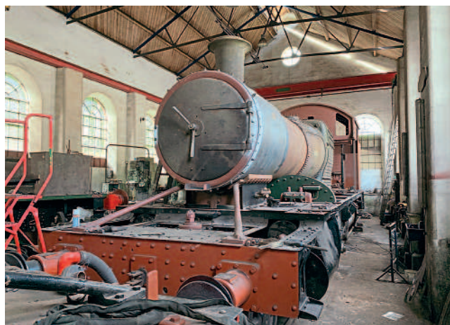
Above: The boiler of Mike Little's small 2-6-2T No. 5538 trial fitted into the frames at the Flour Mill. BILL PARKER
