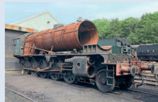
WD 2-10-0 No. 3672 Dame Vera Lynn awaiting movement into Deviation shed at Grosmont on June 23. Its smokebox, front tubeplate and boiler tubes have already been removed in preparation for its forthcoming overhaul. IAN FOOT
