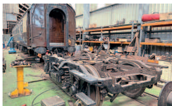
The wheelset change and brake overhaul of Pullman car Eagle inside Tyseley Locomotive Works. DENIS CHICK/VT
