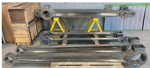
The two outside connecting rods for No. 2007 Prince of Wales at Darlington Locomotive Works. A1SLT
