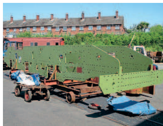
The frames, with buffer beam, after sandblasting and a protective coat of paint at Whitehead. RPSI
