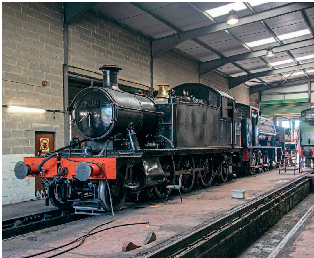
GWR 4575 2-6-2T No. 5553 is almost ready to return to service at Peak Rail following overhaul by the Waterman Railway Heritage Trust. Having made initial moves under its own steam at the beginning of March, it was photographed in Rowsley shed on June 12, awaiting final painting and the construction of its firebox brick arch. The last steam locomotive to leave Barry scrapyard in 1990, it returned to steam at Tyseley in 2002 and spent the next 10 years based on the West Somerset Railway and touring other preserved lines until its boiler certificate expired. ALISTAIR GRIEVE
