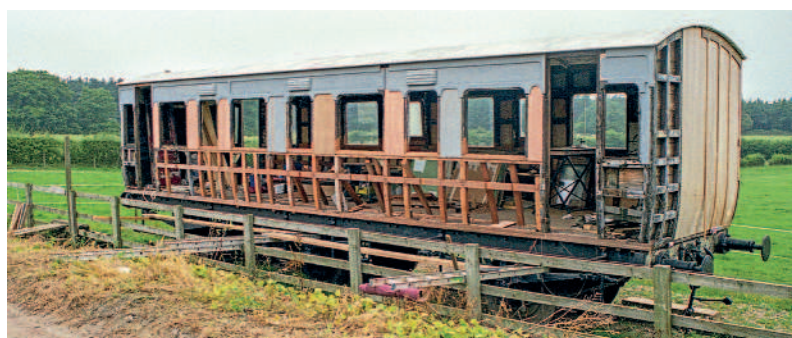
Within 12 months of Stephen purchasing GER coach No. 37 in 1998, around £15,000 had been spent on a sound but speedy restoration outdoors in the corner of a Harrogate stable's car park. Most of the money went on hiring specialist contractors to replace 70% of the rotten frame. Certainly, this carriage would have been considered beyond economic 'traditional restoration' but Stephen's realistic approach means that it is now in a condition that will guarantee many years' use. STEPHEN MIDDLETON
