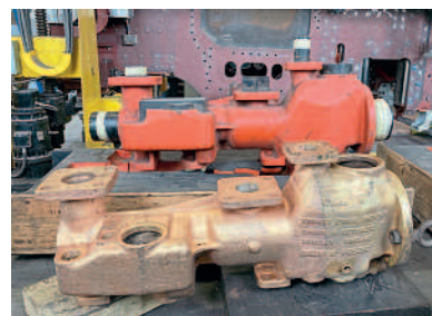
Cleaned Class K exhaust steam injector body from No. 70000 Britannia and the pattern for that for No. 71000 Duke of Gloucester . A1SLT
