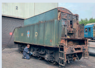
Grosmont shed fitter Andrew Jeffrey checking the axleboxes on the tender of WD 2-10-0 No. 3672 Dame Vera Lynn on June 23 in preparation for its move to Ian Riley's works for a contract overhaul. IAN FOOT
