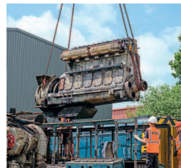
The engine is lifted out of Class 08 No. 08635 at Kidderminster diesel depot. PHIL SEYMOUR/SVR
