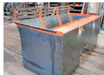
Heritage Engineering Ireland staff have built a replacement coal bunker for Drumboe using original drawings and copying the existing bunker, ready for when the former County Donegal Railways locomotive steams again. HEI
