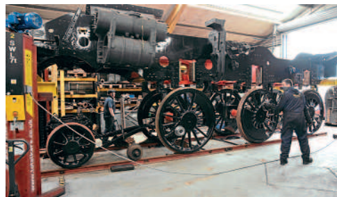
The frames of ex-Barry scrapyard BR 4MT 2-6-0 No. 76077 about to be lowered onto the wheels at Locomotive Maintenance Services of Loughborough on June 17. IAN CROWDER
