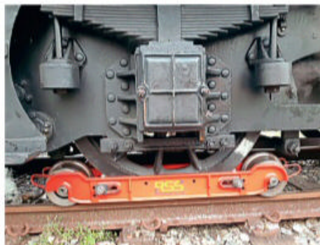
A close up of the RSS WheelSkate supporting the first axle of No. 45231's tender. ANDREW GOODMAN/RSS
