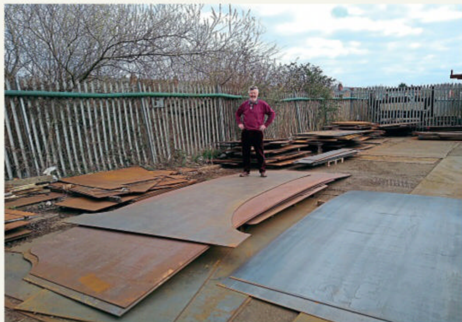
The kit of parts for the new tender tank. GWS
