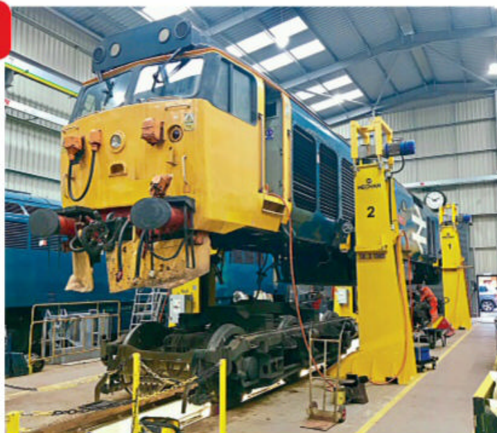
The Class 50 Alliance's No. 50049 Defiance on the jacks inside Kidderminster diesel depot. C50A
