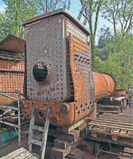
The current state of the boiler of No.1466 showing where new platework will be fitted. PHIL MORRELL
