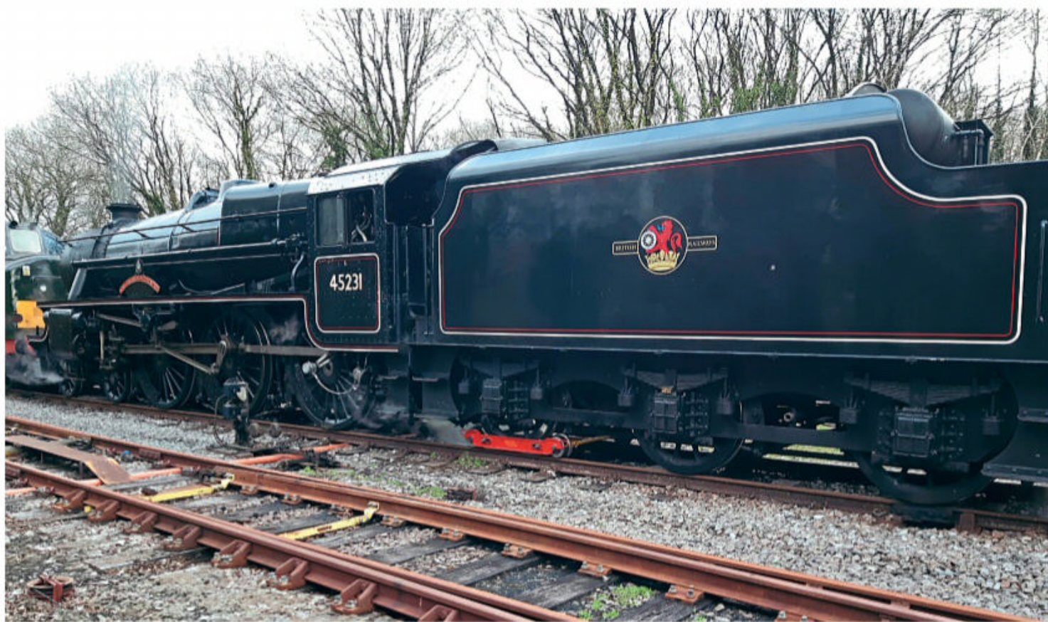
With the locomotive coupled to a Class 37, the front axle of No. 45231's tender is supported by an RSS WheelSkate. ANDREW GOODMAN/RSS
