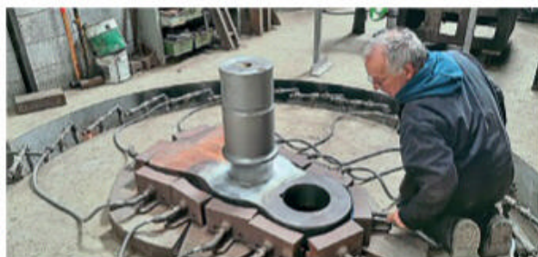
Above: One of the crank axle webs is seen being heated and being prepared for the crank pin to be fitted at South Devon Railway Engineering.
