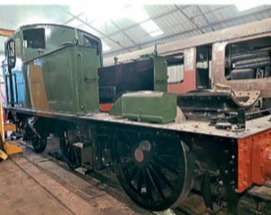
GWR 0-4-2T No. 1466 rewheeled as the latest stage in its most thorough overhaul for 60 years. ED FREEMAN
