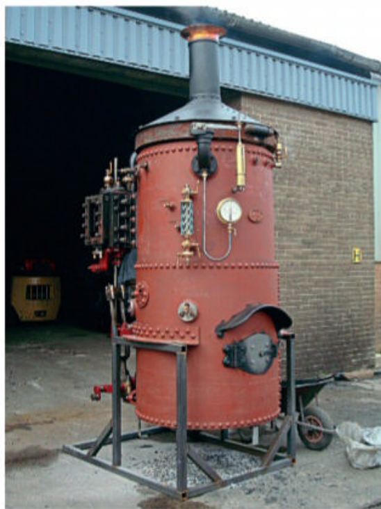
Above: The new boiler being steam tested for the first time, using a special cradle to stand it upright. BEAMISH
