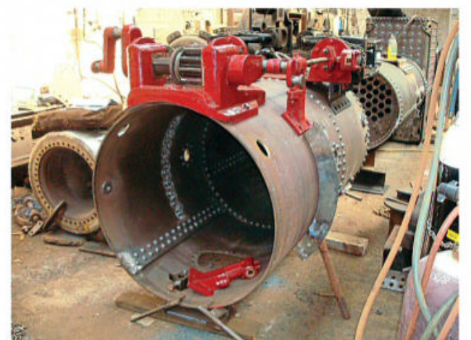
The new boiler is seen under construction at Israel Newton & Sons near Bradford. This represented a significant investment in the project and has enabled 'Coffee Pot' to remain operational since March 2010. BEAMISH MUSEUM
