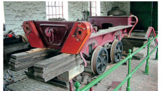
The frames are a single piece of cast iron, a very unusual arrangement for a railway locomotive. They are seen here at the start of the last restoration in late 2006. BEAMISH MUSEUM
