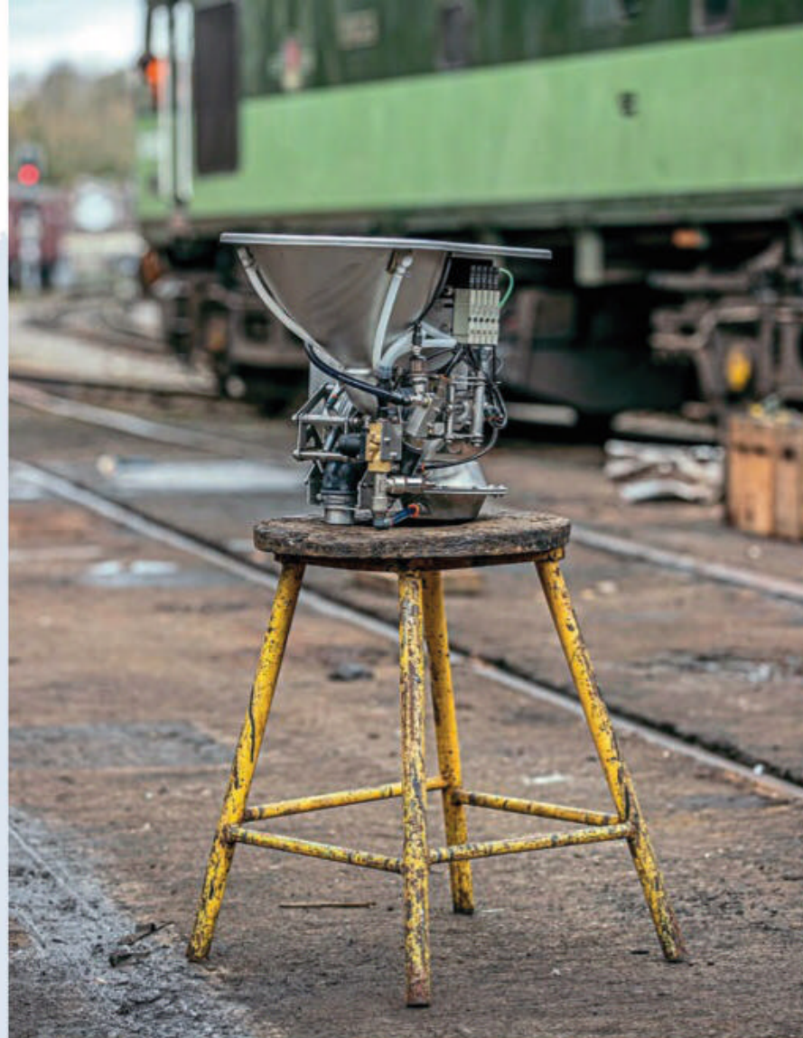
The carriage toilet retention tank apparatus. NYMR
