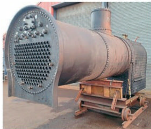
Above: The boiler of Bagnall Austerity The Duke , ready in March for hydraulic testing. EVR
