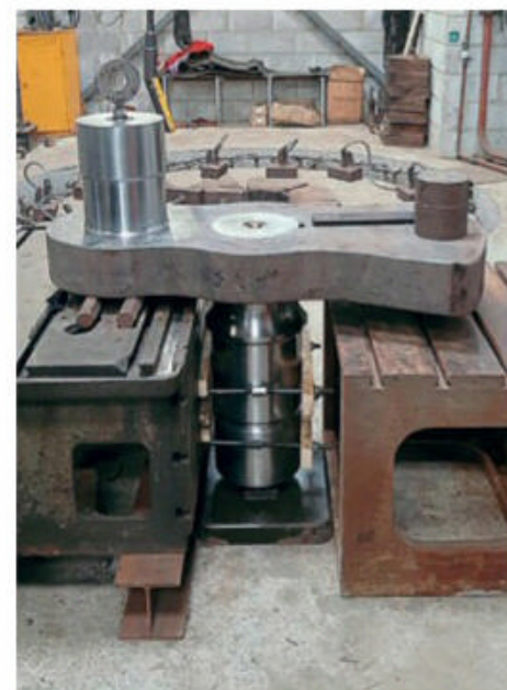
Above: One of the machined new front cylinder covers for No. 71000 Duke of Gloucester , seen at Tyseley.
