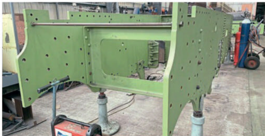
The main frames for County of Montgomery erected at Tyseley Locomotive Works. GARY BOYD-HOPE
