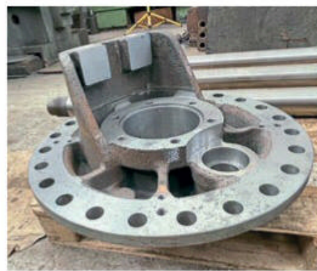
Above: One of the machined new front cylinder covers for No. 71000 Duke of Gloucester , seen at Tyseley.
