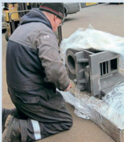
Mark Ashton, of North Bay Railway Engineering Services of Darlington, is seen examining the excellent exterior finish of the new Mountaineer's right-hand cylinder on March 23. NBRES
