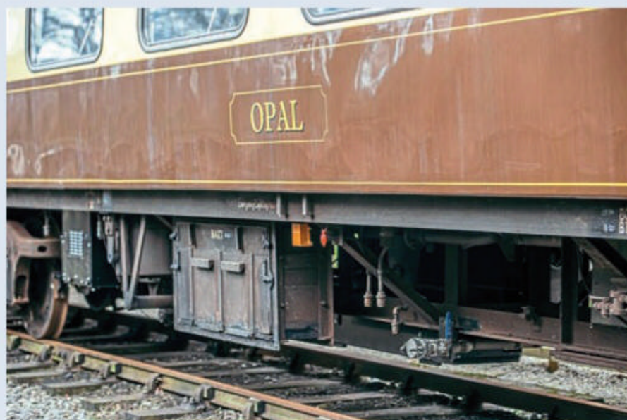
Pullman dining car Opal with its new retention tank. NYMR
