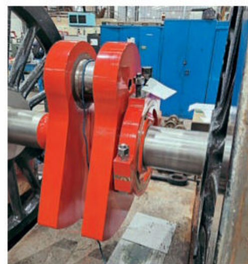
No. 60532 Blue Peter 's crank axle, showing the eccentric strap and sheave after fitting to the axle. LSL
