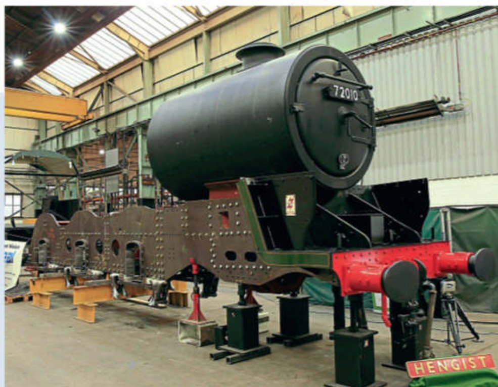
New-build Clan Pacific No. 72010 Hengist takes shape in the CTL Seal factory in Sheffield. SSLC
