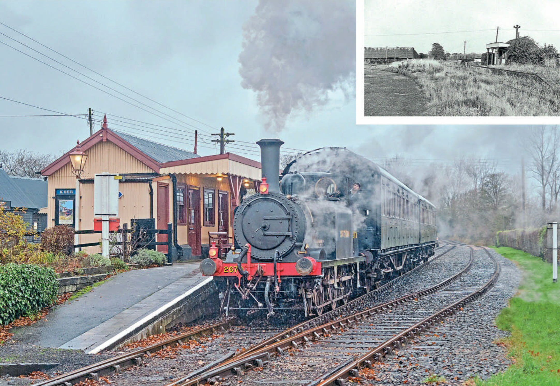
Ready for service: LBSCR Class A1X No. 32678 Knowle , in Southern Railway livery as No. 2678, departs from the Kent & East Sussex Railway's Bodiam station during a pre-Christmas loaded test run. It culminated in the 141-year-old 0-6-0T passing its steam test and thus becoming available for a post-Covid return to traffic after a two-year overhaul, which included the fitment of a larger Isle of Wight-style bunker. The Brighton-built 'Terrier' was saved for preservation after withdrawal in 1963 with 1,411,436 miles on the clock, arrived at the KESR in 1988, and has become a mainstay of the line and popular with passengers and volunteers alike. Bodiam station was opened by the Rother Valley Railway in April 1900, closed by BR to passengers in January 1954 and to freight in June 1961, and was reopened by KESR preservationists in April 2000 to become the 10½-mile Tenterden-based line's southern terminus. ALAN CROTTY. Inset: An abandoned Bodiam station in August 1962, just over a year after it had been closed by BR, looking eastward towards Tenterden. CREATIVE COMMONS
