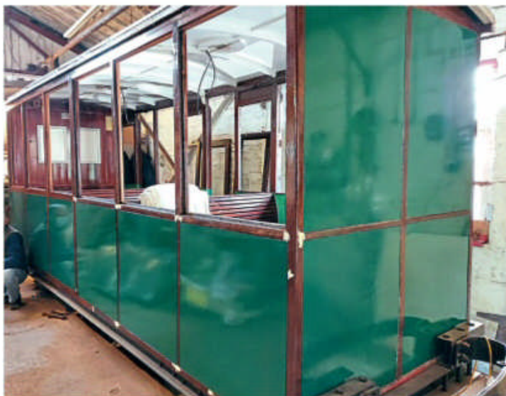
Preparing and filling the exterior woodwork of carriage No. 4. ALAN TITHERIDGE
