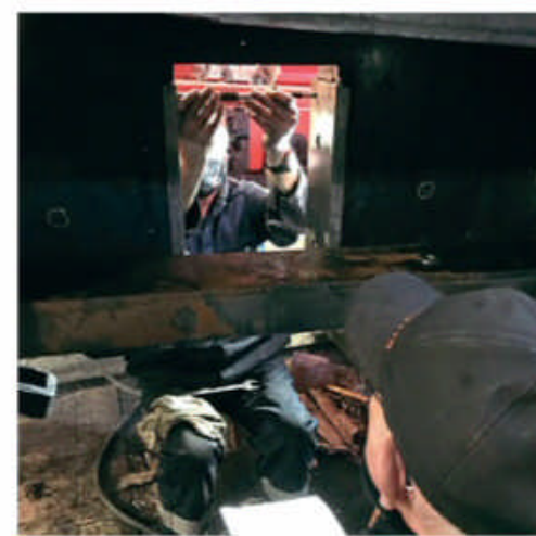
The left leading horn guide for No. 63395 is seen being measured on November 18. IAN PEARSON/NELPG
