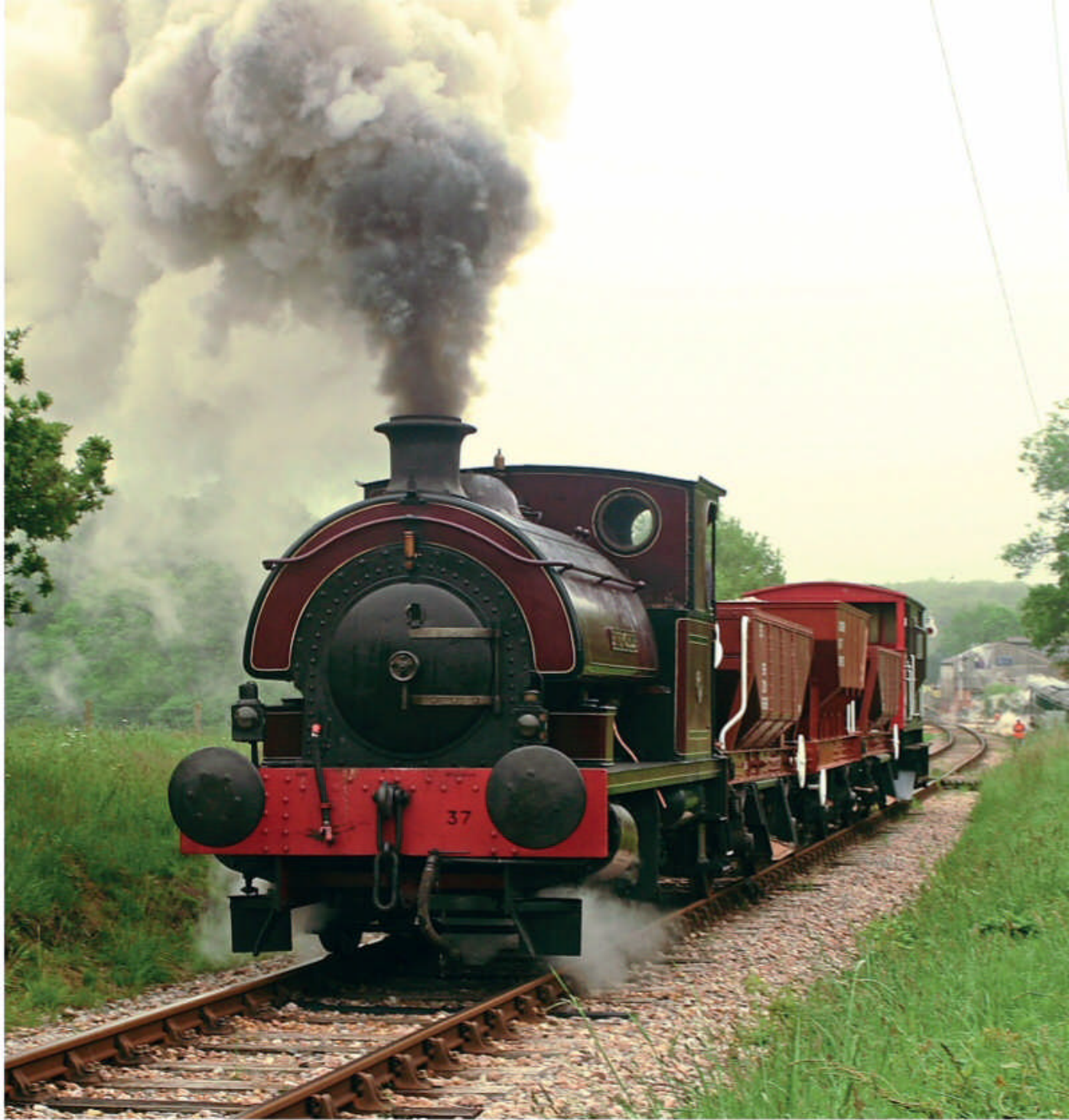
Hawthorn Leslie 0-4-0ST No. W37 Invincible arrived on the line on June 3, 1971. Although currently under overhaul, the locomotive is seen in fine form climbing the 1 in 68 from Havenstreet with a demonstration freight train on May 6, 2006. PHIL MARSH
