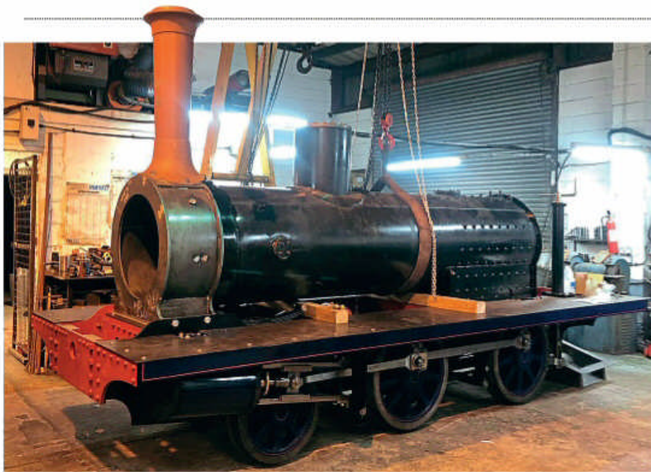
The chimney has been fitted to the £300,000 replica of Sharp Stewart 3ft gauge 2-4-0T Blyth which is being built by North Bay Railway engineering Services in Darlington for the Southwold Railway, with the hope it will steam this summer. NBRES
