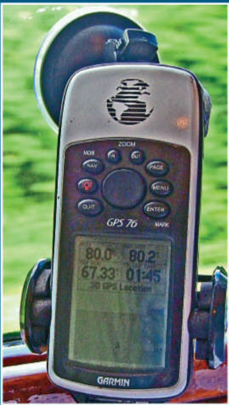
A key tool for recording train performance is a GPS instrument. Pictured here is the author's Garmin 76 GPS, showing readings at St Cross, just south of Winchester. DON BENN
