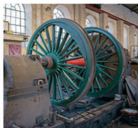
Above: The T3 wheelset journals being polished on the Flour Mill lathe. 563LG
