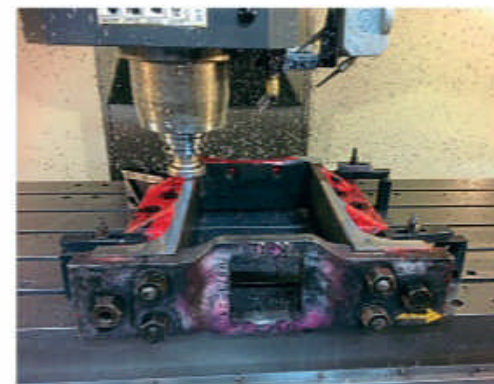
The horn guide for No. 69023 Joem is machined on December 18. NEAL WOOD/NELPG
