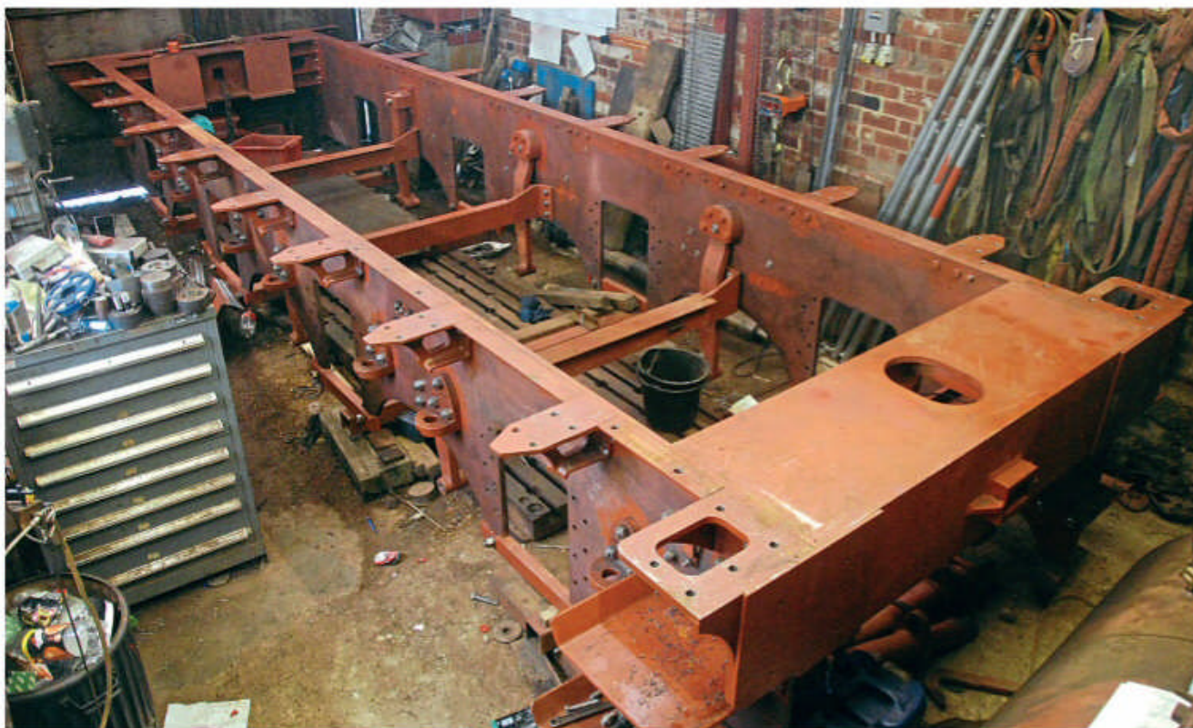
Steady progress with the tender frames continues at Ian Howitt's workshop at Crofton. The initial machining of the hornblocks having been completed, they have been dispatched to North View Engineering Solutions for welding on manganese steel liners, and are now back at Crofton for final machining. Many details for the brake linkage and handbrake mechanism have been made, including the brake cross stay and brake cross shaft. NIGEL FACER/AISLT
