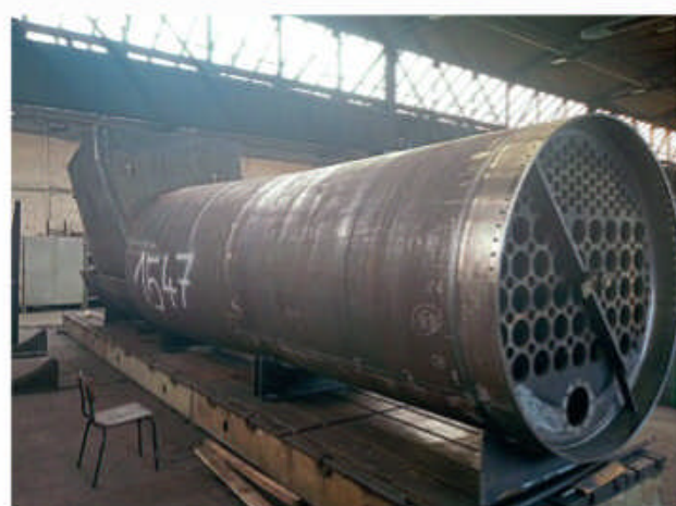
Assembly of the first boiler taking place at DB Meiningen. A1SLT
