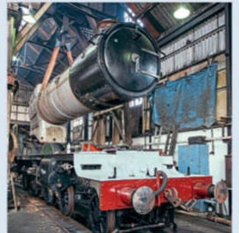
The overhauled and tested boiler of GWR 4-6-0 No. 4079 Pendennis Castle being reunited with the frames in Didcot's lifting shop. FRANK DUMBLETON
