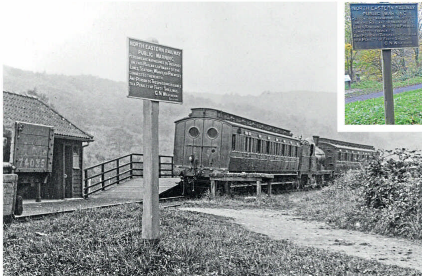
Sign here: A push-pull autotrain at the isolated Beck Hole station in North Yorkshire in about 1910. The train was driven from a driving compartment in the leading coach with the fireman on the footplate of the centrally-located locomotive. The driver had control of the regulator by way of a connection to the engine that ran under the coach, and also controlled the brakes via a second connection to the locomotive which also operated the whistle above the driving compartment. The driver and fireman communicated through a speaking tube. Other than information boards, the only indication today that this remote spot was once the location of a station is the surviving North Eastern Railway trespass sign. NYMR ARCHIVE. Inset: The trespass sign today. BARBARA PRINCE
