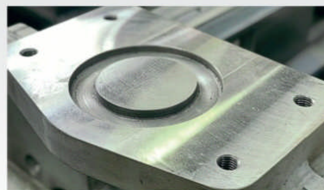
A machined pony truck frame vertical bearer pad at North View Engineering Solutions. A1SLT
