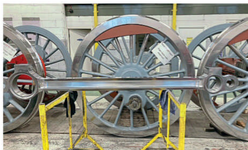
Above: Mirror finish polished intermediate coupling rod. A1SLT
