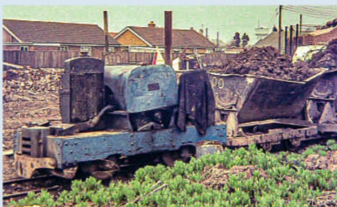
The Simplex in everyday working condition at Skegness Brickworks, hauling 'tubs' of clay for making into bricks. GEOFF HANKIN/LCLR
