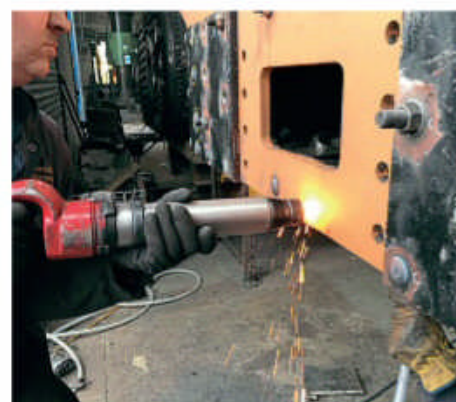
No. 76077's new rear buffing plate being riveted in place. IAN CROWDER
