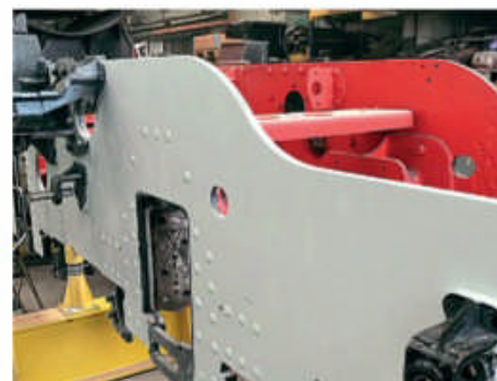
The left-hand side of No. 76077's frames ready for finish coats of gloss black. IAN CROWDER
