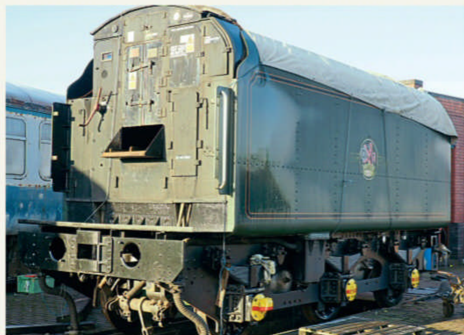
The tender body for No. 71000 has now been returned to the chassis at Tyseley.
