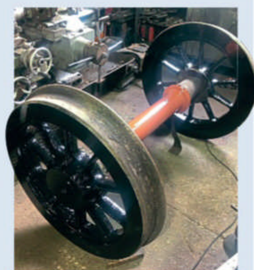
Nearing reassembly, the new 'Night Owl's' pony wheelset has been shot blasted, primed, undercoated and already received its first coat of gloss paint. On completion, the entire truck will join its other wheelsets in storage. LEAKY FINDERS
