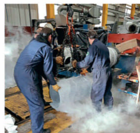
A cylinder liner is fitted to No. 60532 Blue Peter at Crewe on November 17. IAN WALKER
