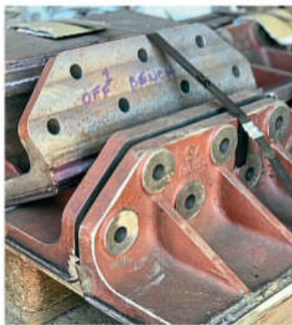
Steady progress with the tender frames continues at Ian Howitt's workshop at Crofton. The initial machining of the hornblocks having been completed, they have been dispatched to North View Engineering Solutions for welding on manganese steel liners, and are now back at Crofton for final machining. Many details for the brake linkage and handbrake mechanism have been made, including the brake cross stay and brake cross shaft. NIGEL FACER/AISLT
