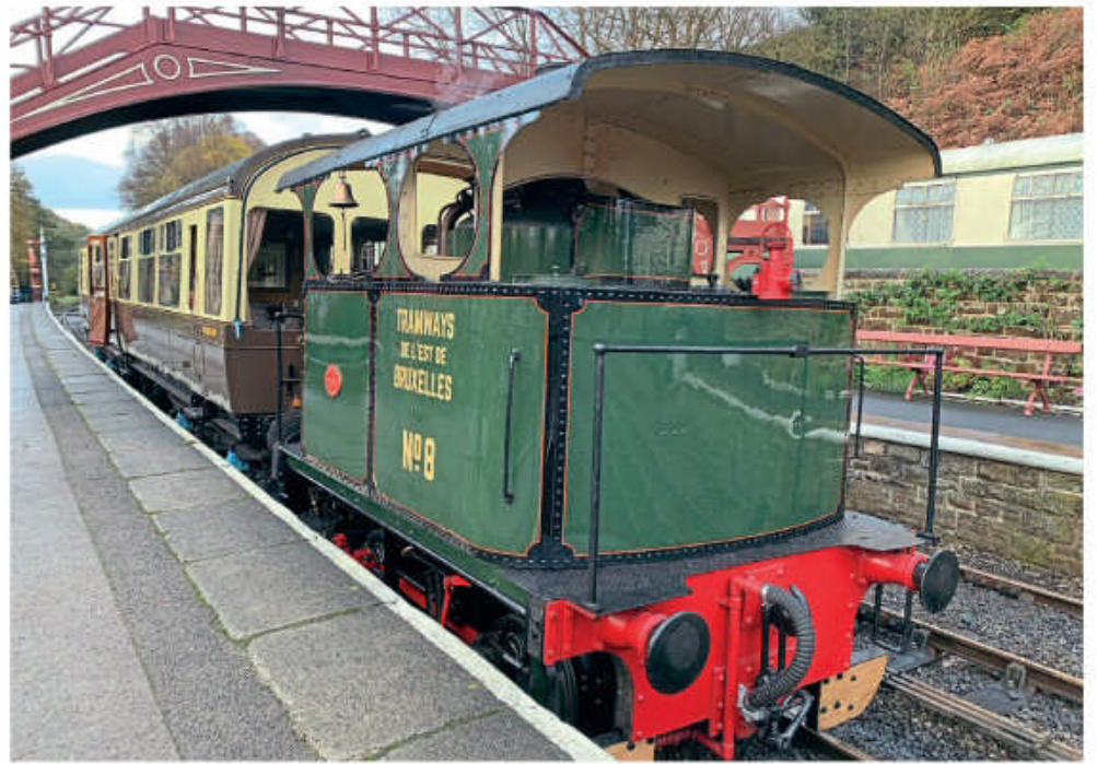
The smallest steam locomotive on the North Yorkshire Moors Railway has returned to traffic following overhaul. Cockerill 0-4-0 vertical-boilered steam tram No. 8 Lucie , which dates from 1898, was bought by NYMR traction and rolling stock manager Paul Middleton from the Middleton Railway in September 2017, and is now running again. Lucie is seen at Goathland during its first loaded test run on October 30. It is now likely to be used for carriage steam heating and shunting. BILL PARKER
