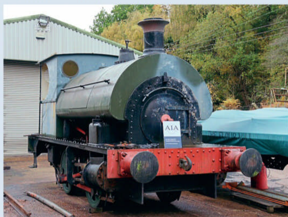
Avonside 0-4-0ST No. 1498 of 1906 Desmond is set for a return to steam at the Flour Mill after nearly half a century. LMMR
