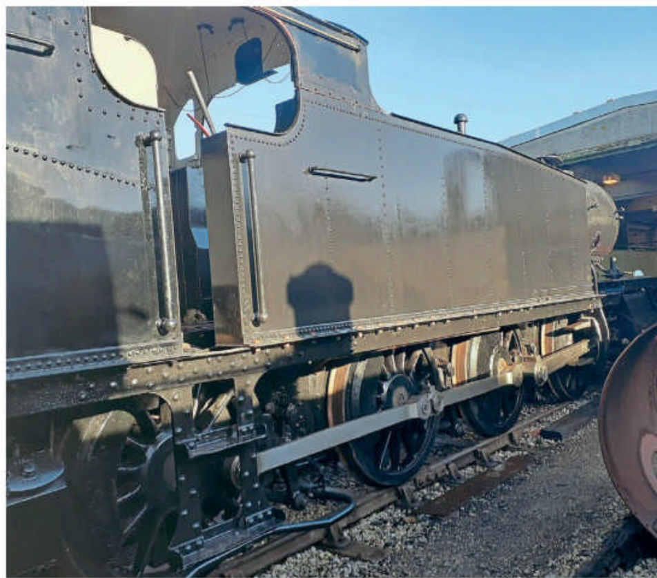
Right: On the way to becoming the first of its class to run in the heritage era: the cab, side tank and smokebox back on the frames of GWR 2-8-2T No. 7200 at Quainton Road on November 13. 7200 TRUST
