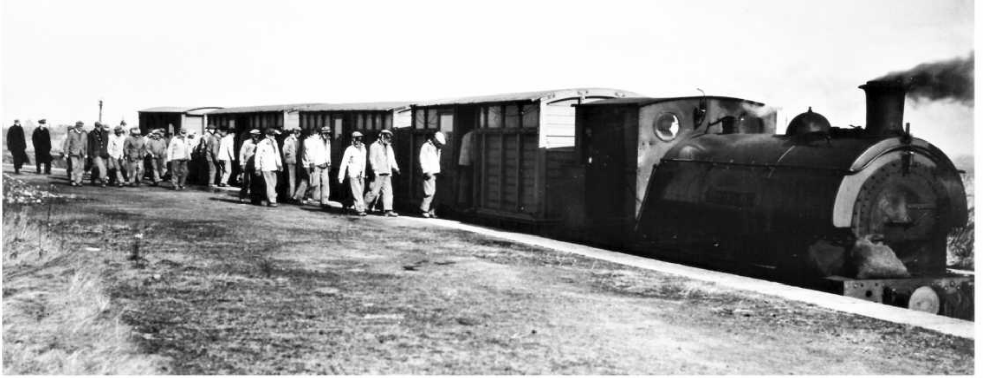
At the featureless Admiralty station within the prison yard we find R & W Hawthorne, Leslie & Co 0-6-0ST Edward VII waiting with a train of three of the line's four-wheel carriages and the brake van as a large group of men board for work at the Stirling Hill quarries in the early 1950s, with two prison warders bringing up the rear. The angle of the shadows suggest that this is the 1pm train returning inmates to the quarry after their lunch break. Five locomotives were purchased for the Admiralty railway, all new, that pictured being the largest and also the last, in 1905. June 1941 had seen Edward VII sent to Rosyth dockyard on the north side of the River Forth, and it did not return home until March 1946, with its scrapping ultimately undertaken in 1957. Maud Railway Museum Collection
