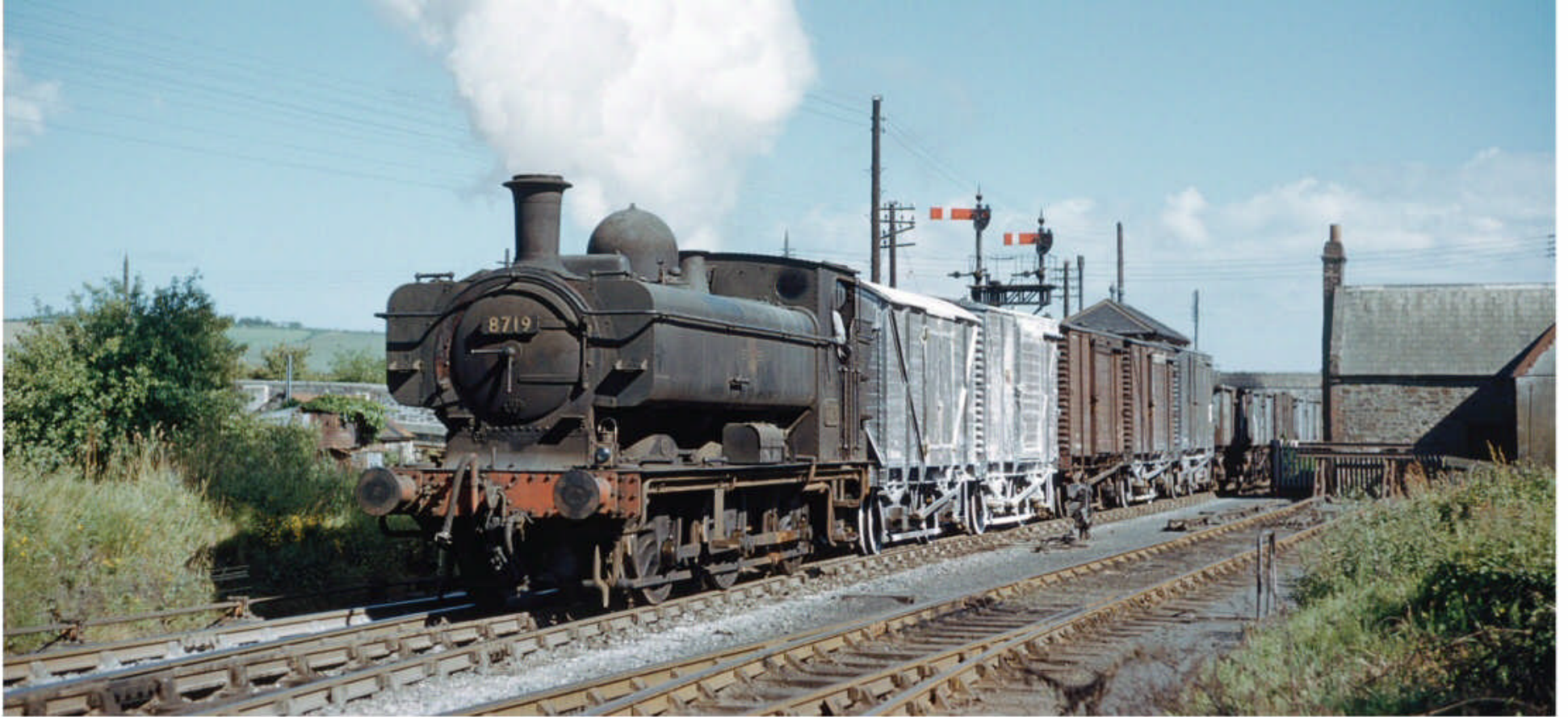
GWR '5700' 0-6-0PT No 8719 leaves the Par Harbour branch and joins the Fowey line at Par Bridge in June 1960. ECC clay dries around the port were fed by pipeline from the production areas, the 16 ton mineral wagons likely to be empties that conveyed coal inwards for these, while the box vans will be taking bagged clay away. The maximum permitted load was 30 wagons, with trains going in the other direction being propelled from St Blazey yard to the harbour transfer siding inside the docks. Keith Pirt, courtesy Book Law Publications
