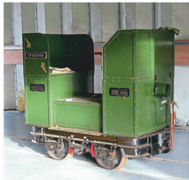
The Ashover Light Railway Society's restored unique battery electric locomotive Spondon . ALRS
