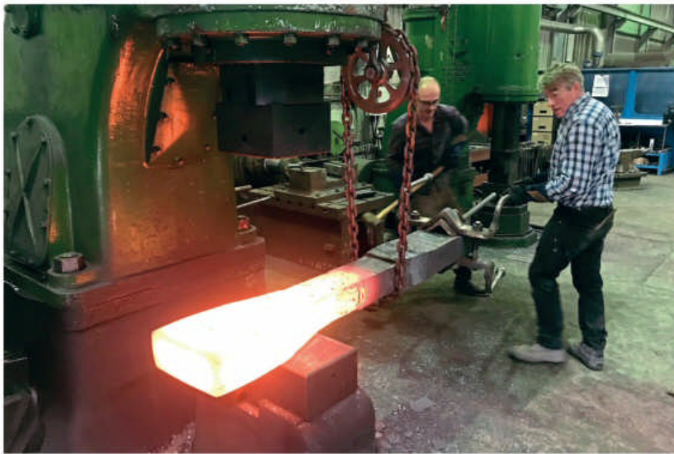
One of the final pair of coupling rods for new-build Gresley P2 2-8-2 No. 2007 Prince of Wales is seen being forged by Stephenson Engineering of Lancashire on November 12. The firm, meanwhile, is nearing the completion of machining the leading coupling rods. To date, more than £2.5 million has been spent and more than £3 million raised of the required £5 million to complete the locomotive within the next three years. To donate to, or join, The A1 Steam Locomotive Trust's project, visit www.p2steam.com , email enquiries@p2steam.com or telephone 01325 460163. A1SLT
