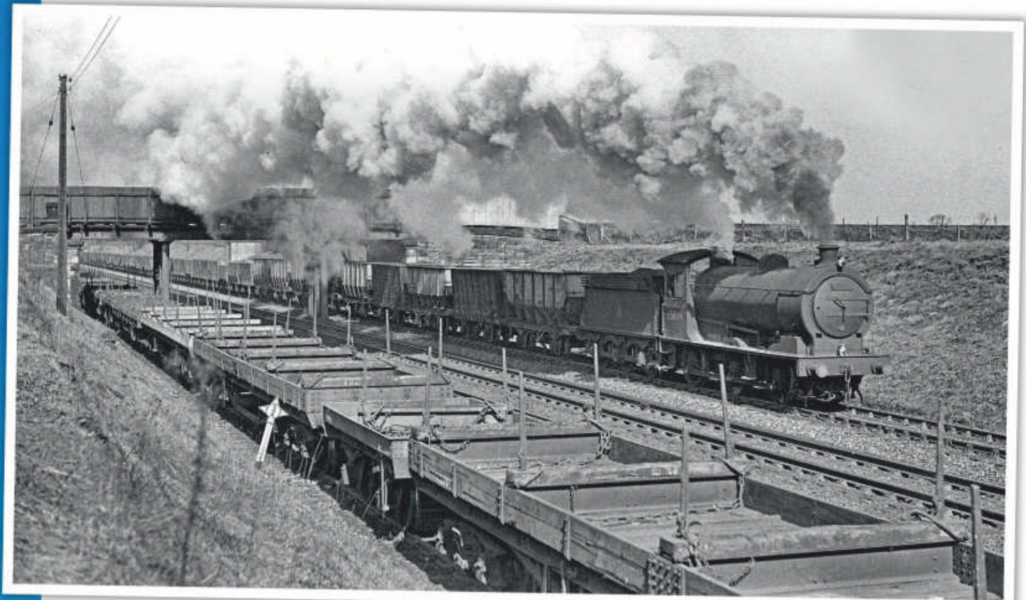
In the late 1950s, J27 0-6-0 No. 65894 is seen heading southbound on the East Coast Main Line at Thirsk with a lengthy train of mineral wagons. JW HAGUE/NELPG ARCHIVE
