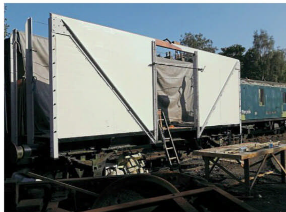
The first painted side panels of LNER four-wheel express fish van No. 75169 bolted into position in early September. ANDREW DANIEL
