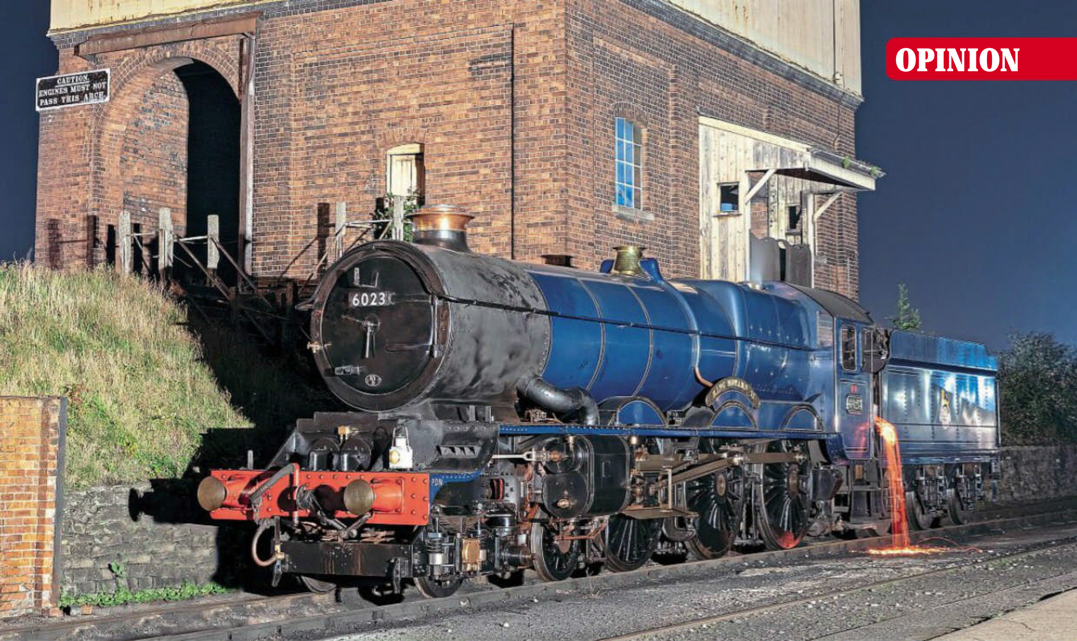
Blue-liveried GWR 4-6-0 No. 6023 King Edward II having its fire dropped for the penultimate time on its last weekend in steam at Didcot Railway Centre on September 12. Its 10-year boiler ticket has now expired. DON BISHOP
