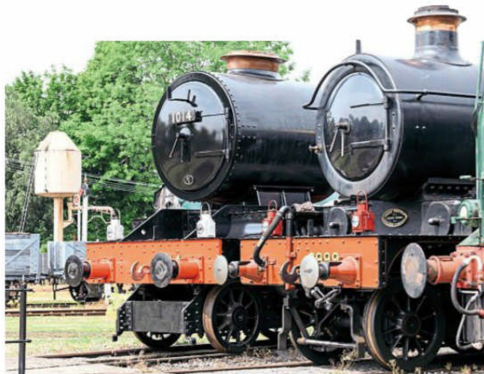
Above: Didcot's two GWR new-builds side by side: No. 1014 County of Glamorgan (left), which has yet to have its boiler fitted, and the Heritage Railway Association award-winning new Saint 4-6-0 No. 2999 Lady of Legend . GWS
