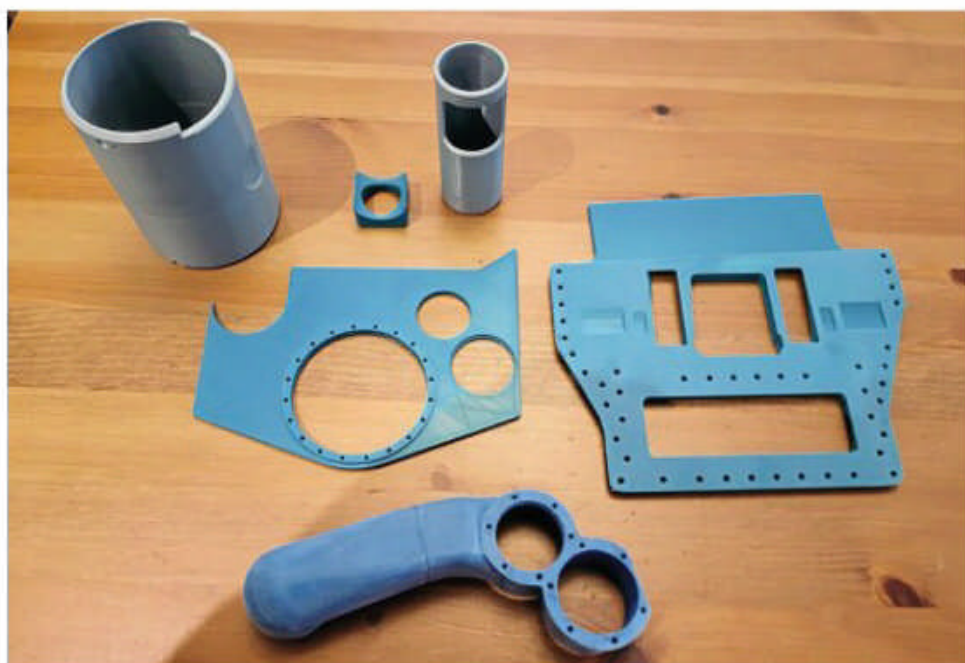
Below: 3D printed cylinder components. A1SLT
