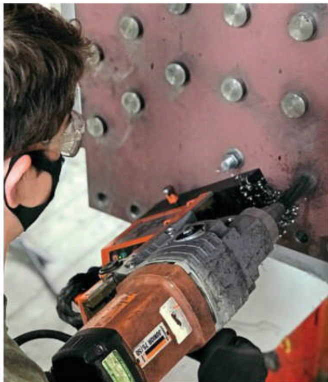
Above: Driven bolts and cold-turned rivet in a spring hanger on July 29. DANIELA FILOVA
