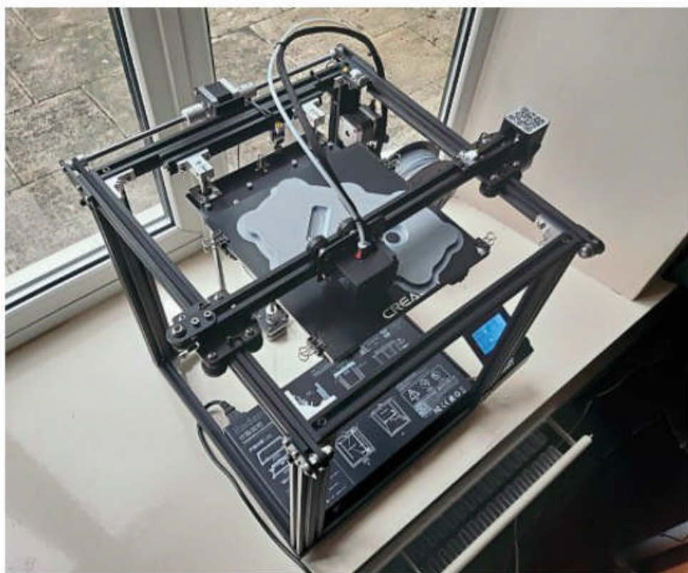
Above: 3D printing of the regulator stuffing box cover underway on July 15. A1SLT
