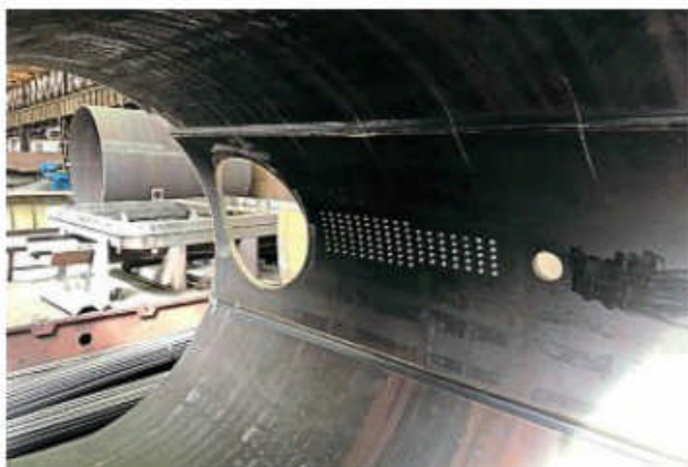
Above: The dome and steam collector holes for the Banjo dome. DANIELA FILOVA
