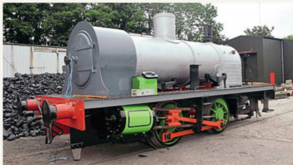
The refurbished boiler back on Swanscombe No. 6 . MR
