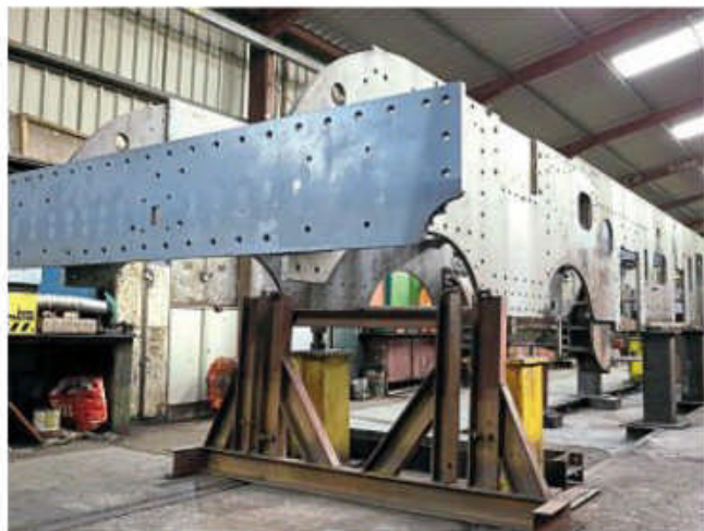
The fully-assembled chassis of B17 No. 61673 Spirit of Sandringham at Llangollen. B17SLT
