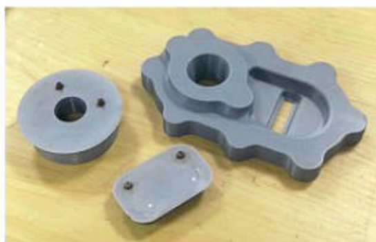
Above: 3D printing of the regulator stuffing box cover underway on July 15. A1SLT
