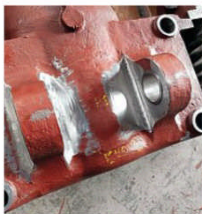
Right: The cannonbox after machining on August 8.
