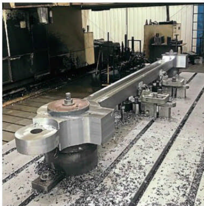
The two middle coupling rods are approaching completion of machining at Stephenson (Engineering) Ltd at Atherton. It is hoped that the relaxation of Covid-19 rules will enable resumption of forging of the other rods in the near future.
