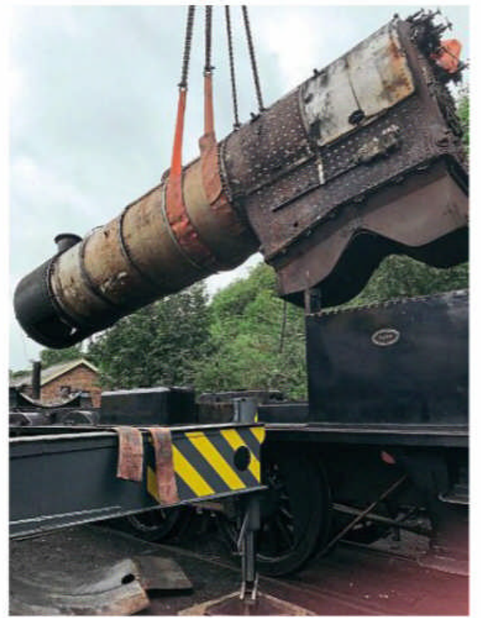
The boiler from Q6 No. 63395 was lifted at Grosmont on September 7. IAN PEARSON/NELPG
