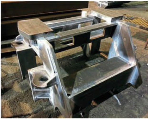
The pony truck frame fabrication on July 9. STEVE DAVIES
