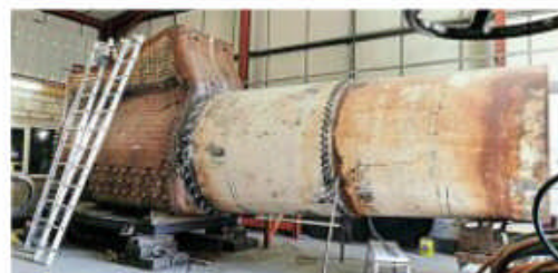
The firebox and the new boiler barrels for No. 1014 County of Glamorgan . GWS
