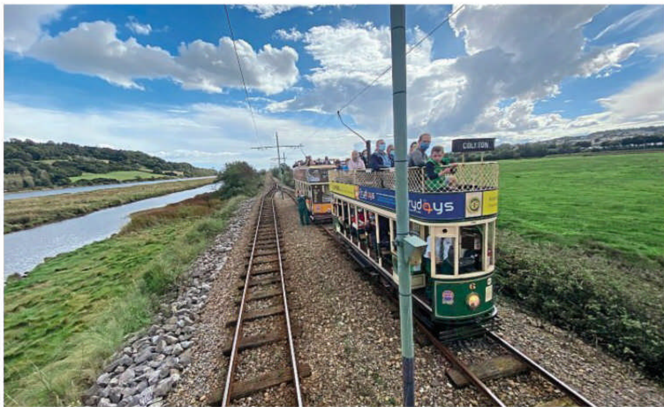
Built in 1954 as a 15in gauge single deck open toast rack, based on the design that operated at Llandudno & Colwyn Bay, Car 6 was rebuilt as a 2ft gauge open topper in 1956 for operation at Eastbourne, based on the ex-Bournemouth open toppers which ran at Llandudno & Colwyn Bay, and again in 1962 with lower deck saloons at either end. It was regauged to 2ft 9in in 1974, rebuilt again in 1989, reverting to its original cross bench lower deck seating arrangement, and is seen in action on the 50th anniversary event on August 28. ST
