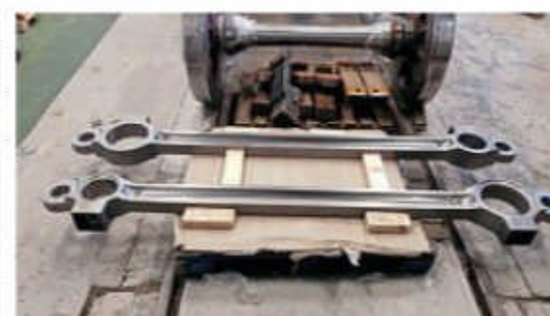
Amongst the latest components to be manufactured for The A1 Steam Locomotive Trust's Gresley P2 2-8-2 No. 2007 Prince of Wales is this pair of coupling rods, machined by Stephenson Engineering of Lancashire and delivered to Darlington Locomotive Works in late September. Will this be the heritage era's greatest achievement? See special feature: pages 60-65. A1SLT
